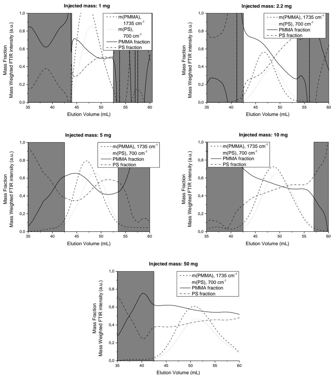
A PS-*b*-PMMA copolymer that shows changes in the chemical composition distribution (CCD) was injected several times with different volumes into a SEC system with TIMO detection to demonstrate the influence of overloading to the CCD. The eluent was THF at 1 mL/min. A semi preparative linear S SDV column was used.
