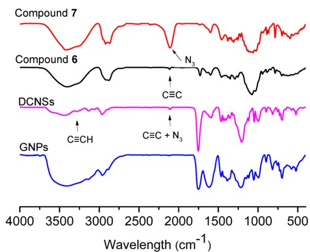
**Fig. S13** IR spectra of **7** (red), **6** (black), DCNSs from **1 + 4** (pink), and glyconanoparticles (GNPs, blue).
