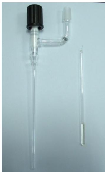
Figure S4. The tube reactor for in situ NMR measurement.
