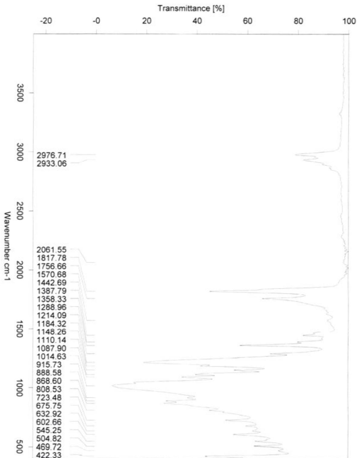
Figure S89. FTIR spectrum of 2-((Ethoxycarbonothioyl)thio)acetic anhydride (14).
