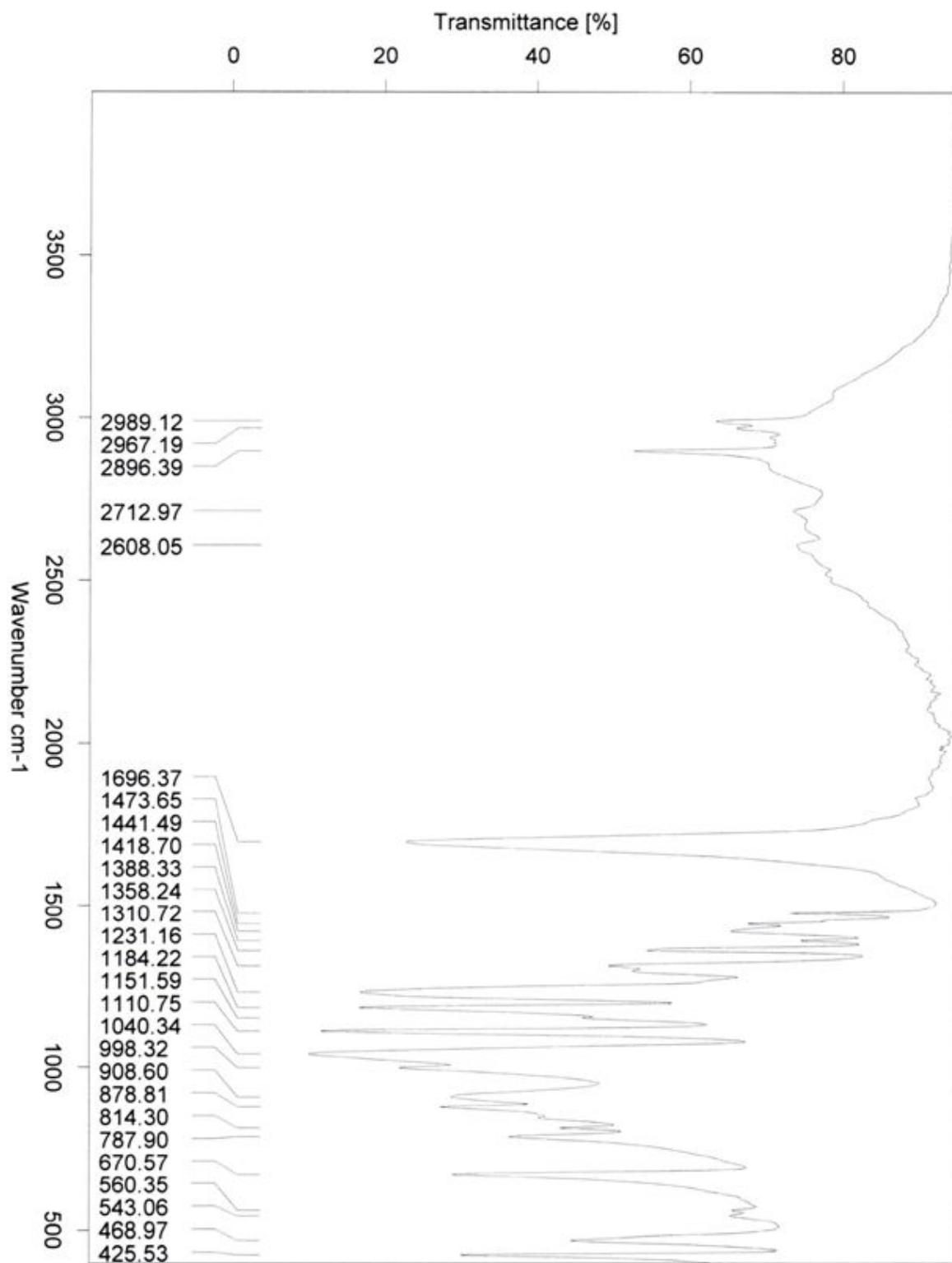
Figure S88. FTIR spectrum of 2-((Ethoxycarbonothioyl)thio)acetic acid (13).
