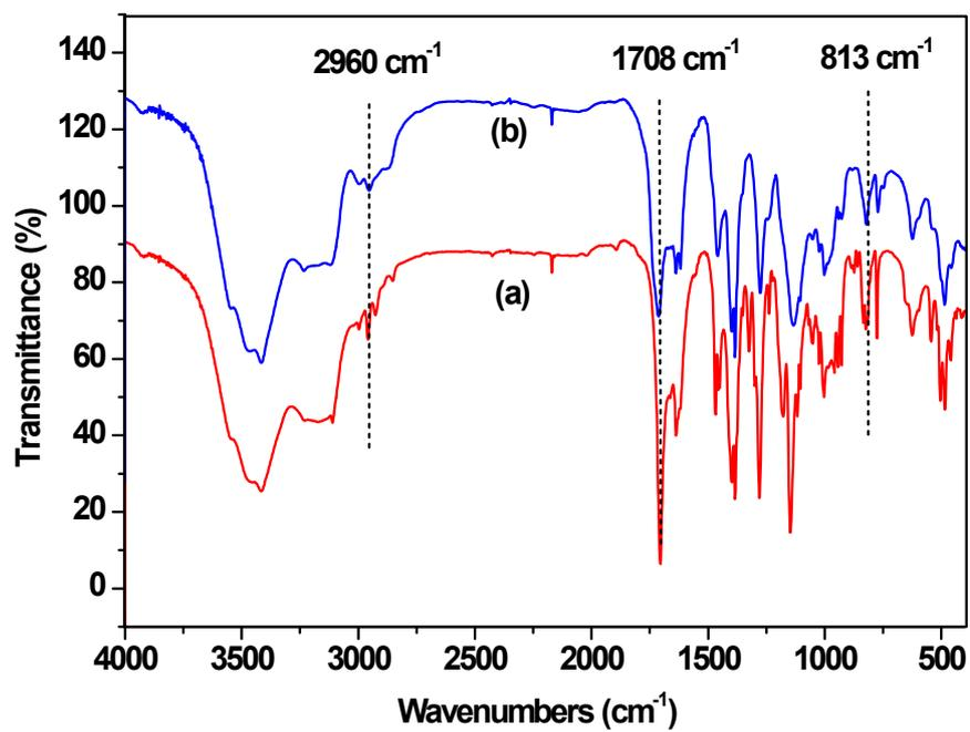
**Fig. S5.** FT-IR spectra of ferrocene-containing monomer MAEFc (a) and block copolymer PEG<sub>45</sub>-*b*-PMAEFc<sub>38</sub> (b).
