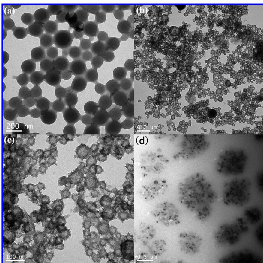
**Fig. S8.** The TEM images of PEG<sub>45</sub>-*b*-PMAEFC<sub>38</sub> vesicles before oxidation (a); after oxidation with KMnO<sub>4</sub> equal amount of ferrocene units in different scale bar (b), (c); reduction with ascorbic acid (d) .
