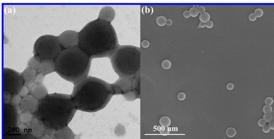
**Fig. S7.** The HR-TEM (a) and SEM (b) images of PEG<sub>45</sub>-*b*-PMAEFC<sub>38</sub> vesicles (polymer concentrations: 0.3 mg mL<sup>-1</sup>, common solvent: DMSO).
