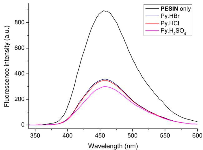
**Figure S5.** Fluorescence spectra of **PESIN** (10  $\mu$ M) upon addition of 125 equiv of pyridine hydrochloride (Py·HCl), pyridine hydrobromide (Py·HBr) and pyridine sulfate (Py·H<sub>2</sub>SO<sub>4</sub>), respectively, in 99:1 (v/v) of DMF/H<sub>2</sub>O, excited at 320 nm.
