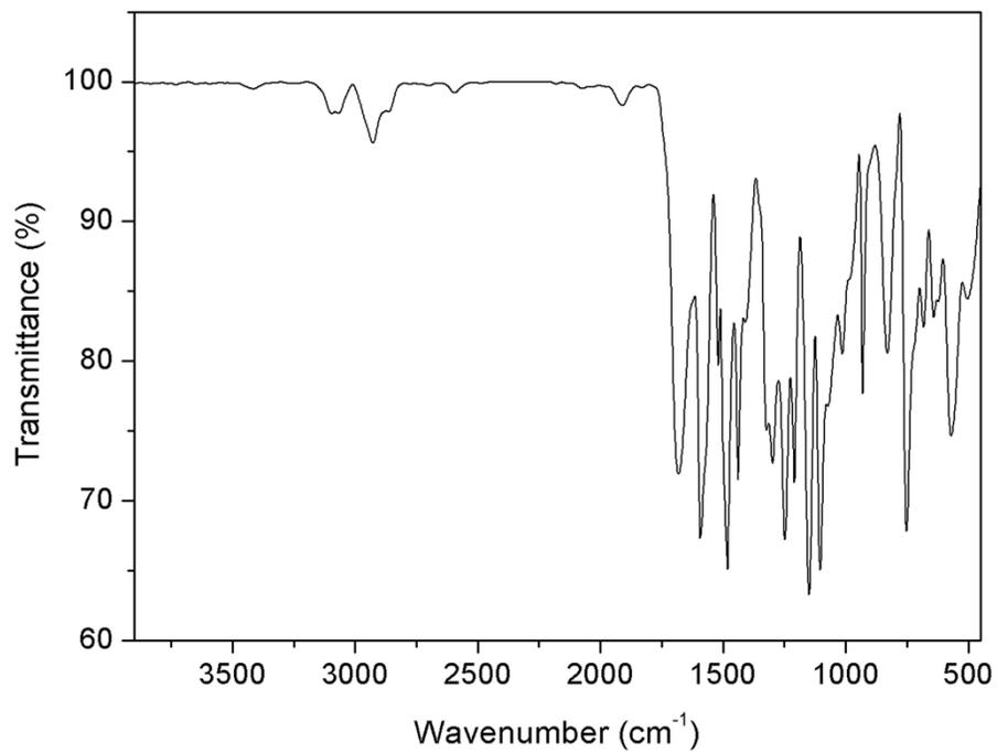
**Figure S6.** The IR spectrum of polymer **PESIN**.
