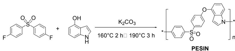
**Scheme S1.** Synthesis of **PESIN** via C–N/C–O coupling reaction.
