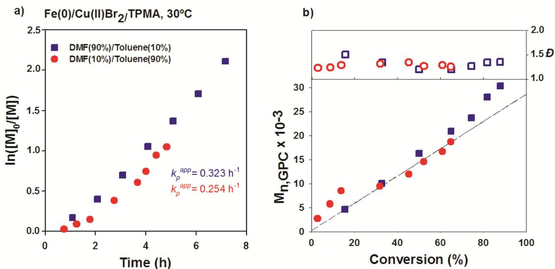
**Fig. S1** SARA ATRP of GMA in toluene/DMF = 10/90 (v/v) and toluene/DMF = 90/10 (v/v) at 30°C. (a) First-order kinetic plot, (b) evolution of MWs and  $M_w/M_n$  with conversion (the dashed line represents the theoretical MW at a given conversion). Reaction conditions:  $[GMA]_0/[EBiB]_0/[Fe(0)]_0/[CuBr_2]_0/[TPMA]_0=200/1/1/0.1/1.1$  (molar).
