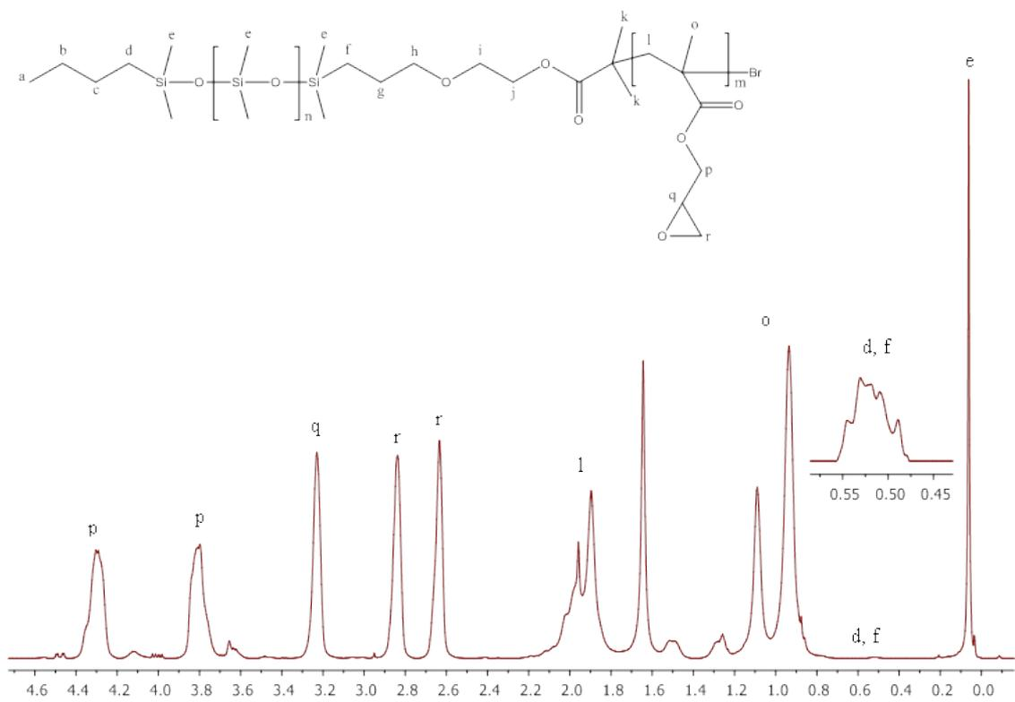
**Fig S3** <sup>1</sup>H-NMR spectrum of the PDMS-*b*-PGMA obtained ( $M_{n,GPC} = 33900 \text{ g mol}^{-1}$ ;  $D = 1.5$ ;  $M_{n,NMR} = 27500 \text{ g mol}^{-1}$ ); in  $\text{CDCl}_3$ .
