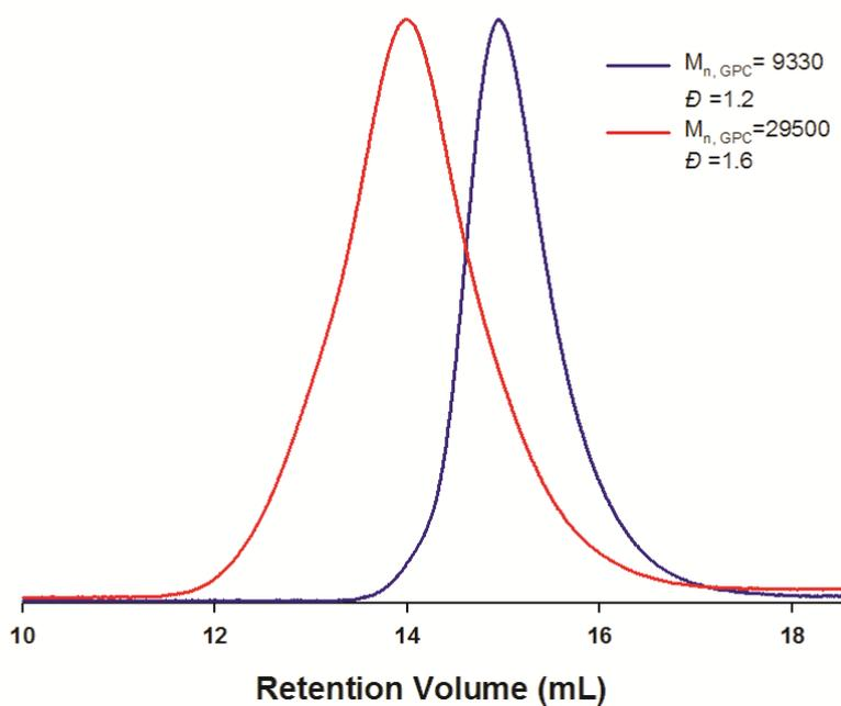
**Fig. S2** GPC traces of PGMA before (blue line) and after (red line) the chain extension experiment.
