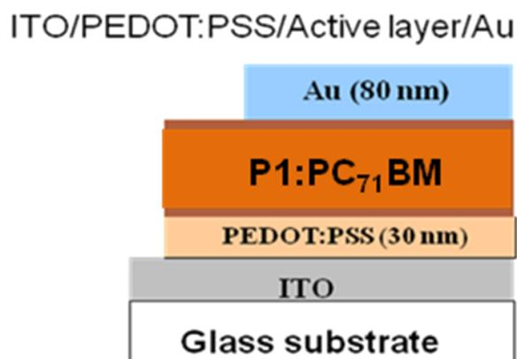
Figure S15. Configuration of the hole only device.
