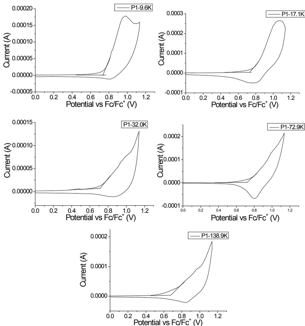
**Figure S13.** Cyclic voltammograms of the polymer fractions. Ferrocene/ferroceium redox couple was used as the internal standard. The HOMO energy level was calculated from the onset of the oxidation potential of the polymer using the following:  $E_{\text{HOMO}} = -(4.8 + E_{\text{ox}} \text{ onset}) \text{ eV}$ .
