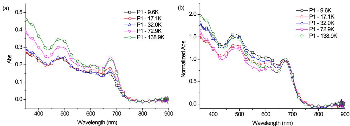
**Figure S14.** (a) Absorption spectrum from films of polymers **P1** blended with PC<sub>71</sub>BM in a 1:2 weight ratio and (b) absorption spectra normalized at the  $\lambda_{\text{max}}$  of the absorption band at 670 nm.
