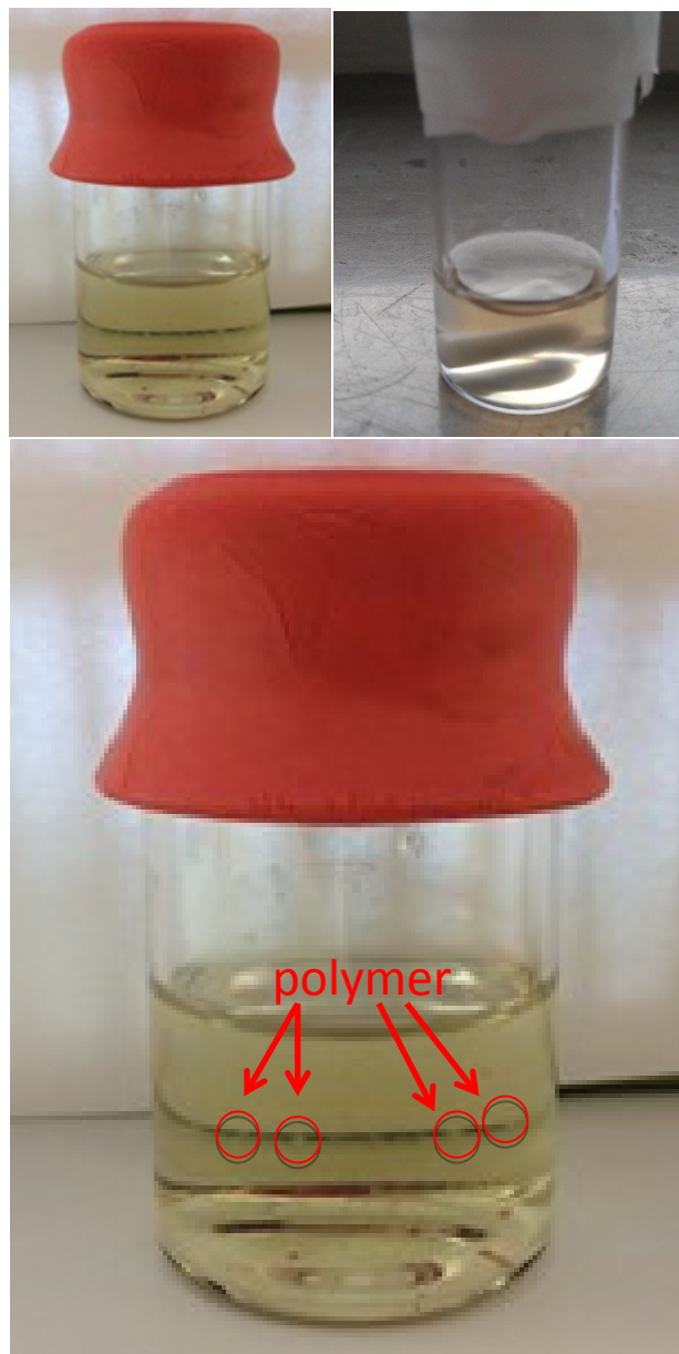
Figure S5. Pictures of l-PDMA (top left) and PDMA (top right) and enlarged picture of PDMA (bottom) in 0.1 mM NaOH solution kept under the protection of nitrogen
