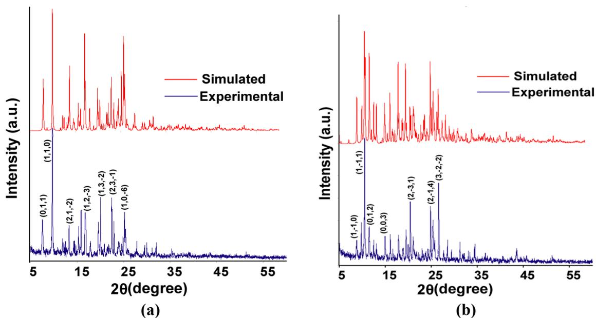
Figure 9S: PXRD pattern of the (a) complex 6 and (b) complex 7
