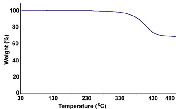
Figure 13S: Thermogravimetry of the complex **1**
