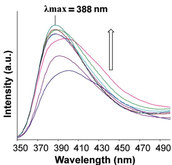
Figure 12S: Temperature dependent fluorescence spectra of the ligand, **L**. Fluorescence intensity increases with increasing temperature ( $30^{\circ}\text{C}$  to  $100^{\circ}\text{C}$ ,  $0.1\text{mM}$  solution in DMF,  $\lambda_{ex} = 340 \text{ nm}$ )
