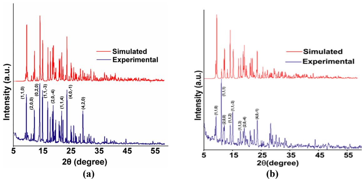
Figure 7S: PXR D pattern of the (a) complex 2 and (b) Complex 3
