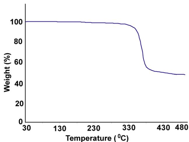
Figure 18S: Thermogravimetry of the complex 6. Complex 6 shows a gradual one step weight loss due to the degradation of organic ligands in the temperature range 130-460 °C.
