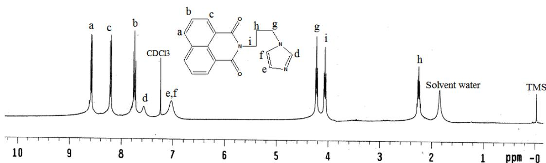
Figure 5S:  $^1\text{H}$ NMR (400MHz,  $\text{CDCl}_3$ ) spectrum of the ligand, **L**
