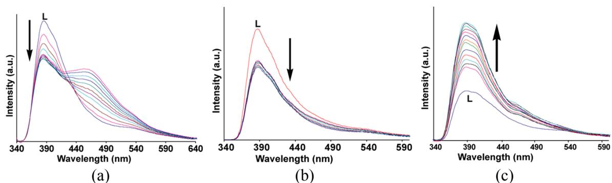
Figure 20S: The changes in the intensity of fluorescence emission ( $\lambda_{\text{ex}} = 340\text{nm}$ ) of the ligand, L (2ml of  $10^{-4}$  M solution in DMF) on addition of (a)  $\text{ZnCl}_2$ , (b)  $\text{CdCl}_2$  and (c)  $\text{HgCl}_2$  (5 $\mu\text{l}$  aliquots of  $10^{-2}$  M solution in methanol) .
