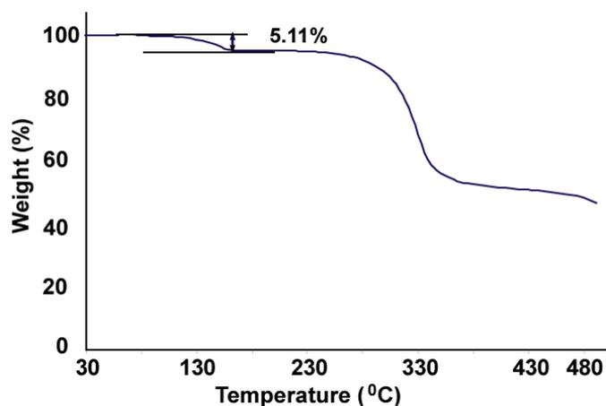
Figure 16S: Thermogravimetry of the complex **4** (For the complex **4**, one step weight loss due to the two solvent acetonitrile molecules takes place in the temperature range 70–170 °C corresponding to a weight loss of 5.11% (calcd 5.56%). The decomposition of ligand at 250 °C-460 °C.
