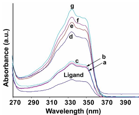
Figure 11S: UV-Vis spectra of the ligand, (a) complex **2**; (b) complex **1**; (c) complex **3**; (d) complex **6**; (e) complex **5**; (f) complex **4**; (g) complex **7**; in DMF (concentration of  $10^{-6}$ M each).
