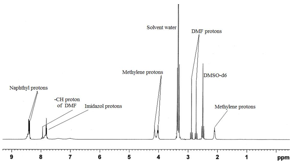
Figure 22S: <sup>1</sup>H-NMR (600 MHz, DMSO-d<sub>6</sub>) spectra of the complex **7**.
