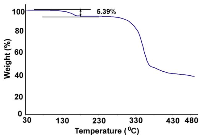
Figure 17S: Thermogravimetry of the complex **5**. The two solvent acetonitrile molecules are lost in the range 88-200 °C corresponding to a weight loss of 5.39 % (calcd. 5.55 % ) and the decomposition of organic ligands at 260 °C-460 °C.
