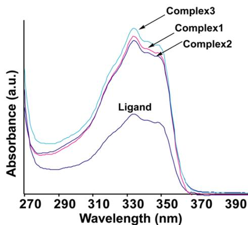
Figure 10S : UV-Vis spectra of the ligand, complex 1, complex 2 and complex 3 in DMF (concentration of  $10^{-6}$ M each)
