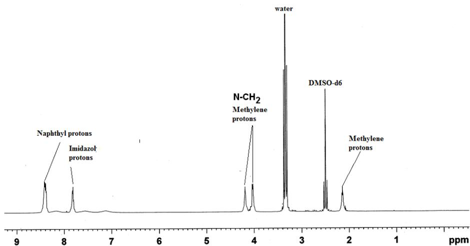
Figure 21S: <sup>1</sup>H-NMR (600 MHz, DMSO-d<sub>6</sub>) spectra of the complex **6**.
