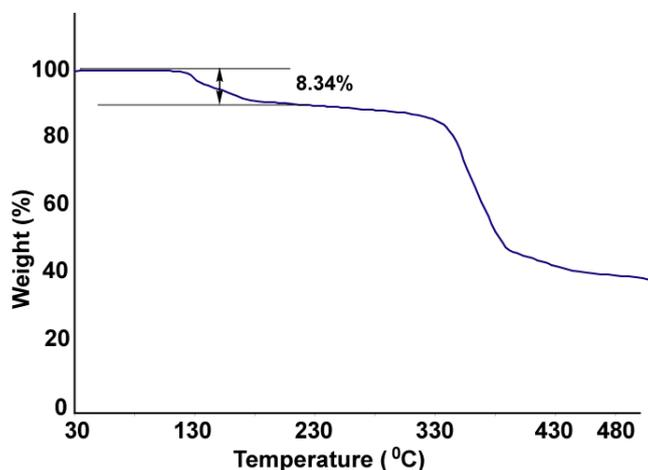
Figure 19S: Thermogravimetry of the complex 7. The complex 7 shows weight loss of 8.34 wt % (calcd. 8.98 wt%) in the range of 120-182 °C corresponds to the loss of one lattice dimethylformamide molecule and one coordinated dimethylformamide molecule.
