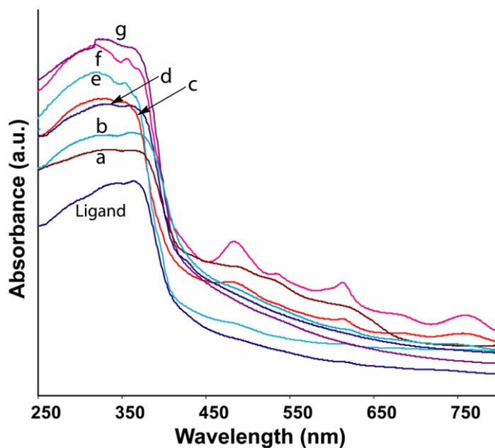
Figure 6S: Solid state UV-vis spectra of (a) complex **5**, (b) complex **7**, (c) complex **6**, (d) complex **2**, (e) complex **3**, (f) complex **1**, and (g) complex **4**.
