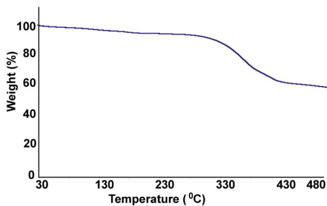
Figure 14S: Thermogravimetry of the complex **2**. In case of the complex**2**, the decomposition of the organic ligand started from 280 °C
