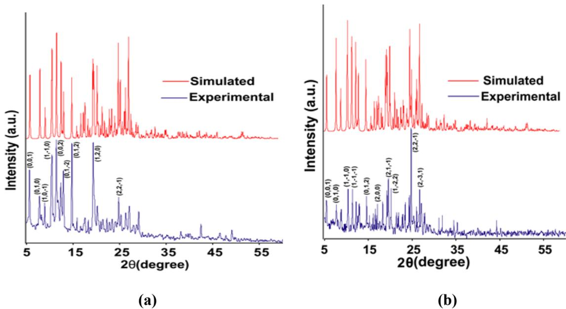
Figure 8S: PXR D pattern of the (a) complex 4 and (b) Complex 5
