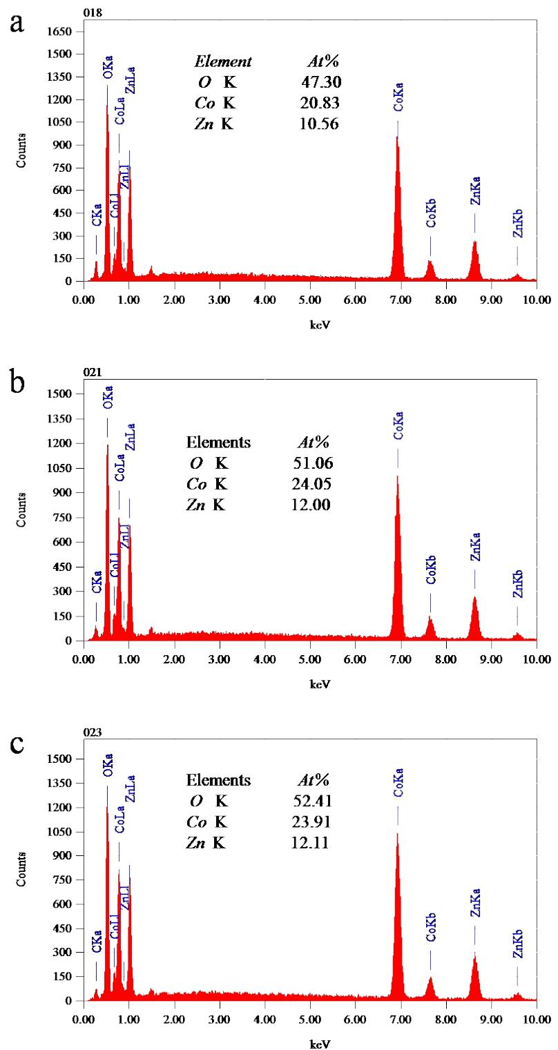
Fig. S5 EDS spectra of (a) compound 1, (b) compound 2 and (c) compound 3.
