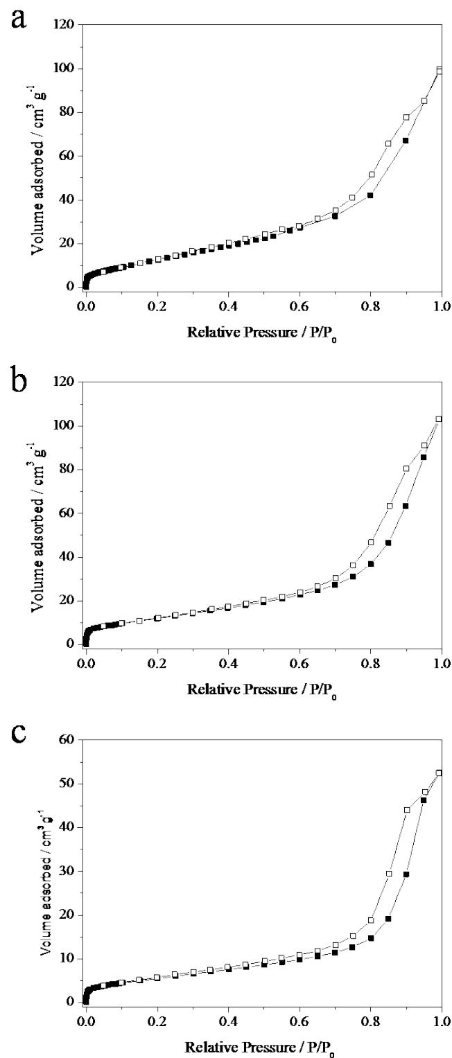
**Fig. S6**  $\text{N}_2$  adsorption-desorption isotherms of (a) compound **1**, (b) compound **2** and (c) compound **3** (solid symbols, adsorption; open symbols, desorption).
