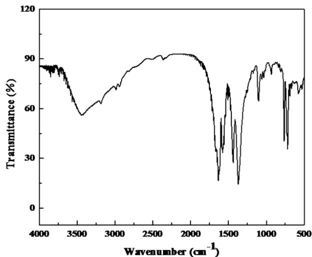
**Fig. S3** FTIR spectra of as-synthesized JUC-155.
