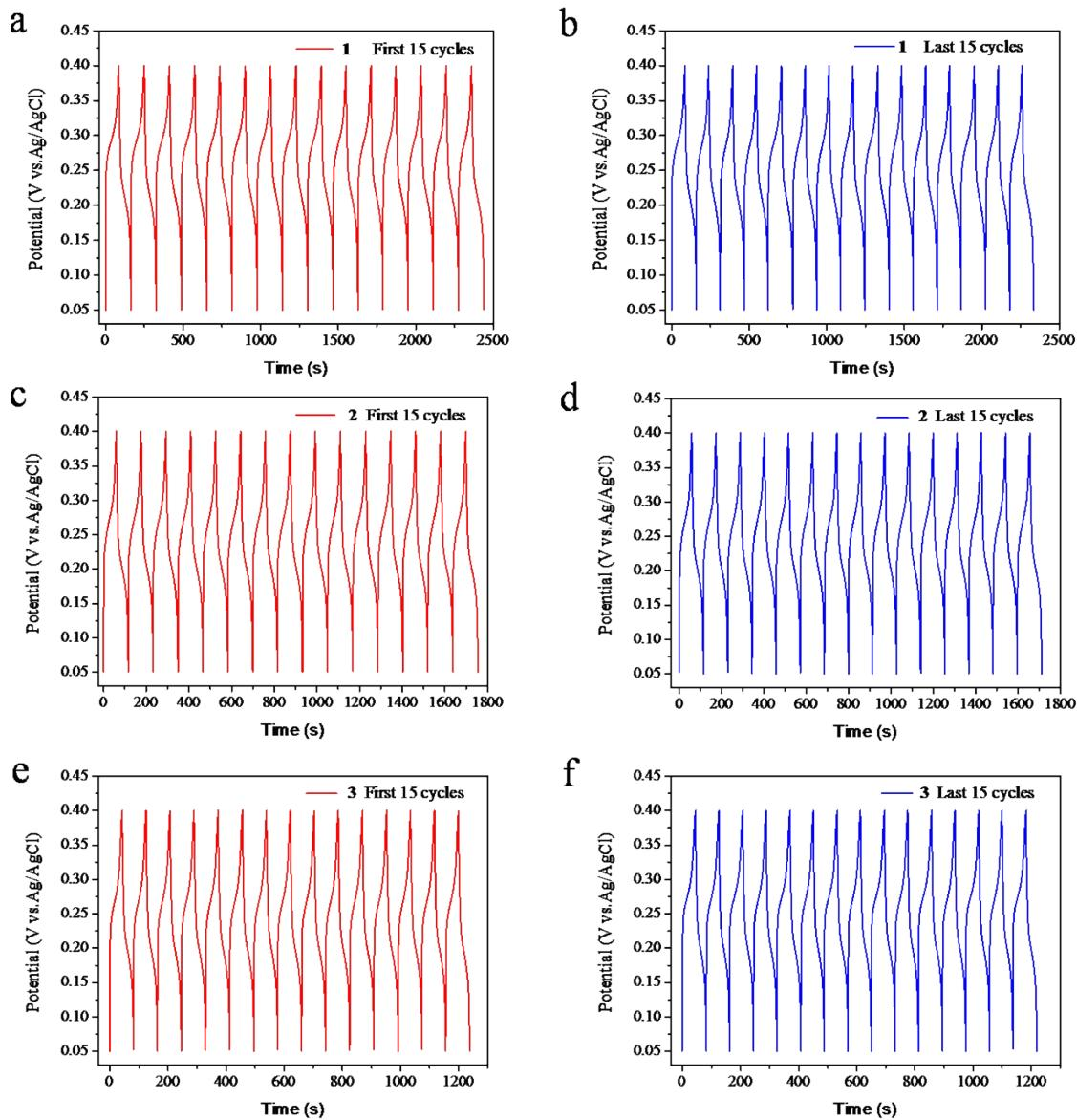
**Fig. S10** The first 15th cycles galvanostatic charge-discharge curves and the last 15th cycles galvanostatic charge-discharge curves of (a, b) 1 electrode, (c, d) 2 electrode and (e, f) 3 electrode at  $2 \text{ A g}^{-1}$ .
