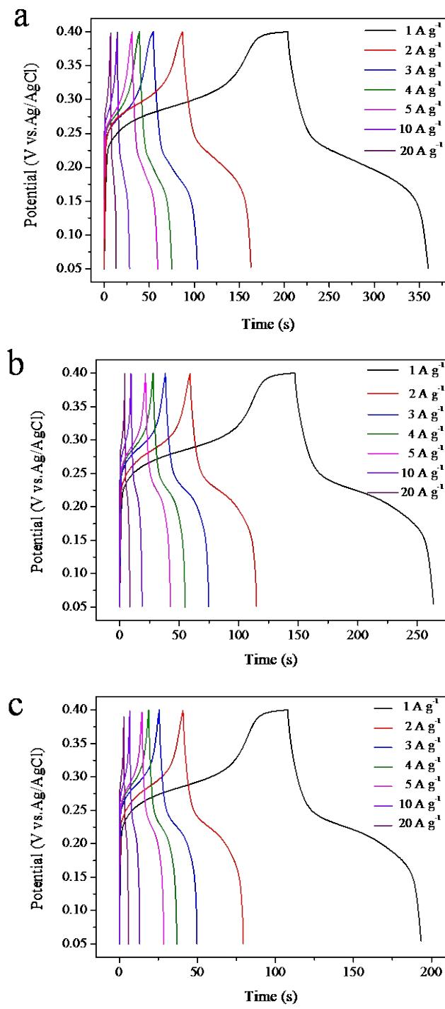
**Fig. S9** Charge-discharge curves at different current densities of (a) **1** electrode, (b) **2** electrode and (c) **3** electrode in 6M KOH aqueous electrolyte.
