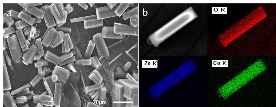
**Fig. S1** (a) SEM images and (b) EDS mapping images of as-synthesized JUC-155.
