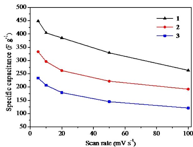
**Fig. S8** Specific capacitance derived from the Cyclic voltammetry (CV) measurement of the **1**, **2** and **3** electrodes.
