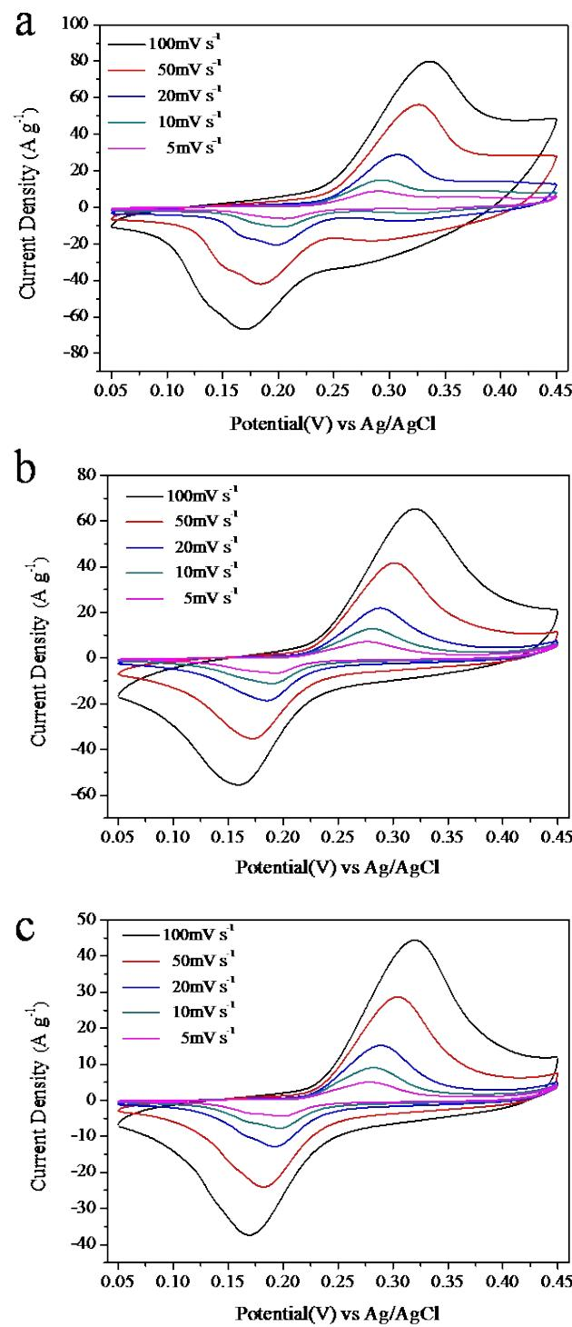
**Fig. S7** Cyclic voltammetry (CV) at different scan rates of (a) **1** electrode, (b) **2** electrode and (c) **3** electrode in 6M KOH aqueous electrolyte.
