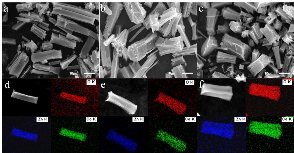
**Fig. S4** SEM images and EDS mapping images of compound **1** (a, d), compound **2** (b, e) and compound **3** (c, f).
