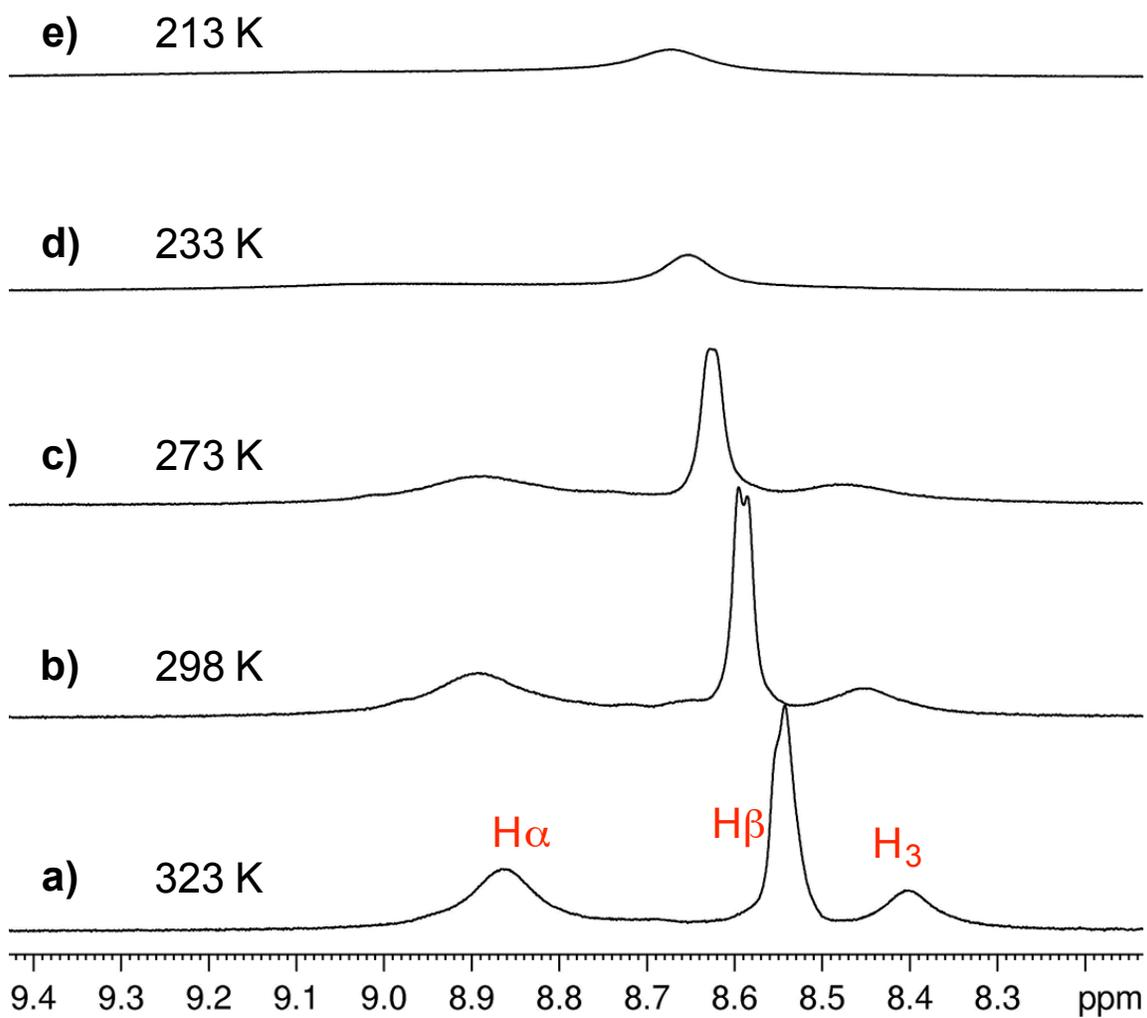
Figure S2. Partial <sup>1</sup>H NMR (500 MHz) spectra of **TPY1** in CDCl<sub>3</sub> at a) 323 K, b) 298 K, c) 273 K, d) 233 K, and e) 213 K.
