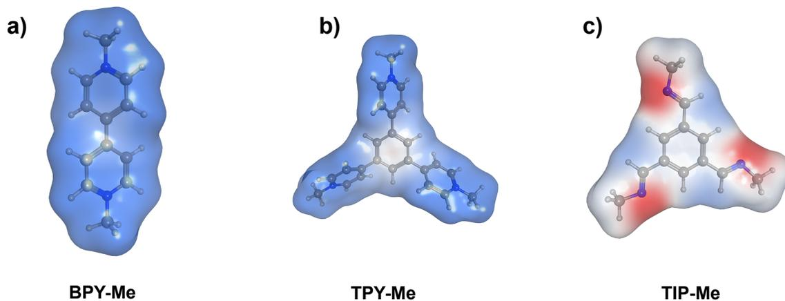
Figure S3. Electrostatic potential surfaces of three model compounds with methyl substituents. a) **BPY-Me**, b) **TPY-Me**, and c) **TIP-Me**. Blue represents positive electrostatic potential and red stands for negative electrostatic potential. The surfaces were optimized with the MMFF94x force field.
