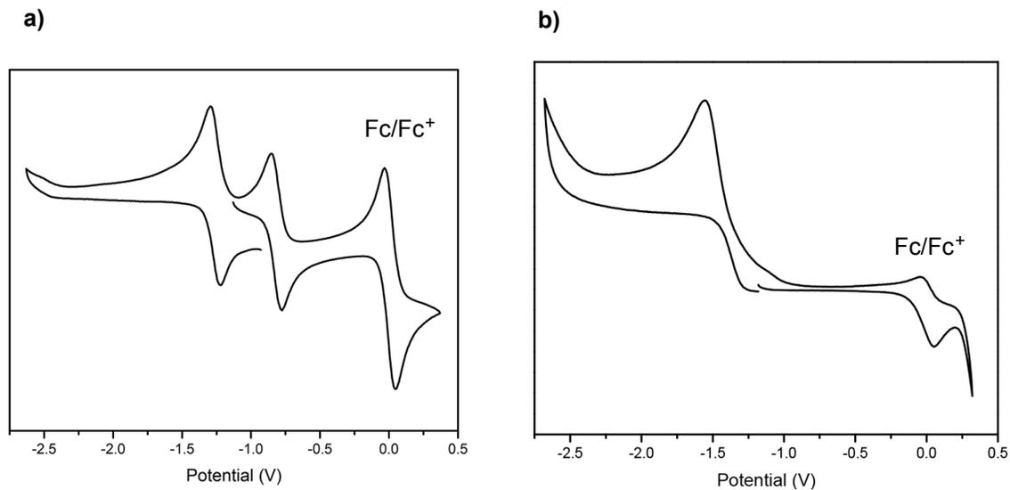
Figure S4. CV of a) **BPY1**, and b) **TPY1** in MeCN, using tetrabutylammonium hexafluorophosphate (0.1 M) as the electrolyte, using ferrocene/ferronium ( $Fc/Fc^+$ ) redox couple as an internal standard. The graphs were calibrated with respect to  $Fc$ .
