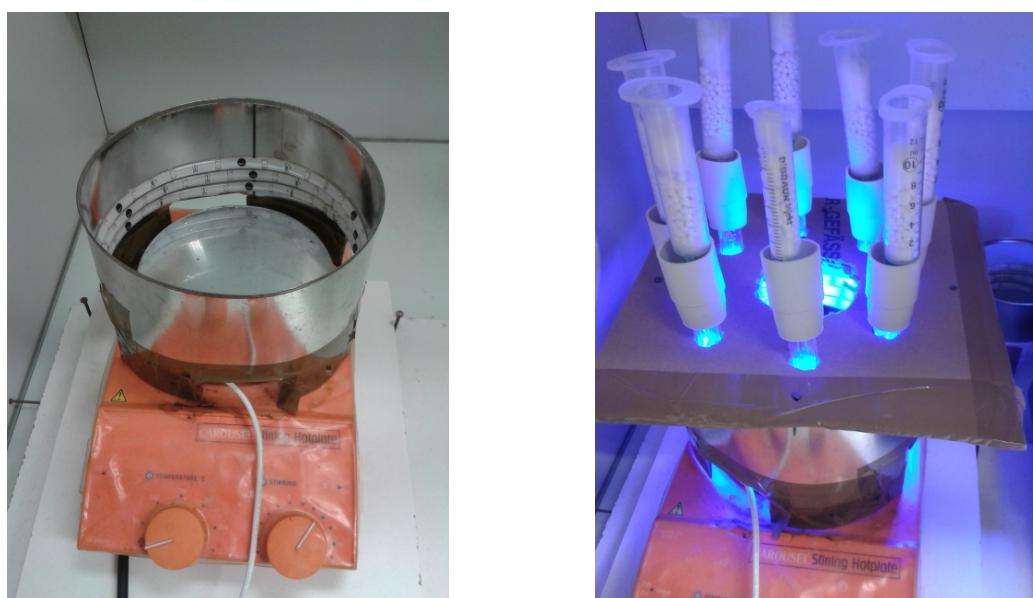
**Figure 1.** Picture of the light chamber equipped with blue LED strips (left) and picture of the light chamber during catalytic assays (right).
