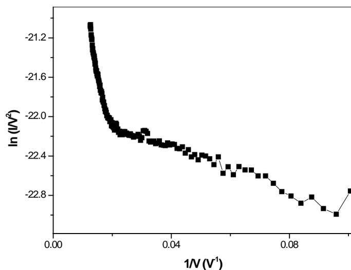
FN plot of ZnO nanotips on MWCNT mat. Linear fit was performed in the high field region and the Value of the slope was found to be -80. Enhancement factor was obtained from the slope of the FN plot.
