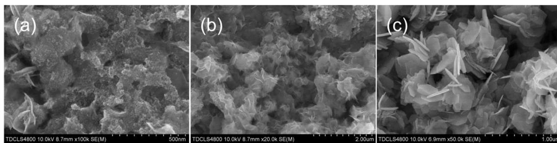
**Fig. 2** SEM images of as-synthesized flower-like microspheres obtained by hydrothermal treatment for different time: (a) 2 h; (b) 5 h; and (c) 20 h.
