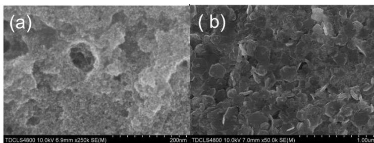
**Fig. 3** SEM images of as-synthesized nanoplates obtained by hydrothermal treatment for different time: (a) 1.5 h and (b) 4h.
