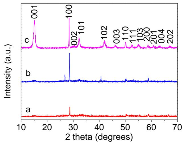
**Fig. 1** XRD patterns of as-synthesized flower-like microspheres obtained by hydrothermal treatment for different time: (a) 2 h; (b) 5 h; and (c) 20 h.
