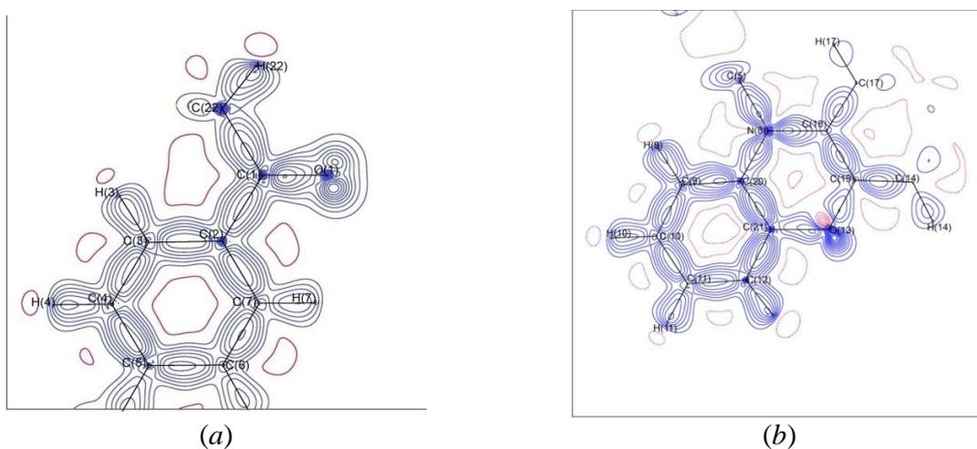
**Figure 4S.** Static deformation density maps for **PAO**: (a) the O(1)C(1)C(2) plane; (b) the O(13)C(20)C(21) plane. Blue solid line – the positive values, red dashed lines – the negative ones. Contours at  $\pm n \cdot 0.1 e \cdot \text{\AA}^{-3}$  ( $n = 0, 1, 2, \dots$ ).
