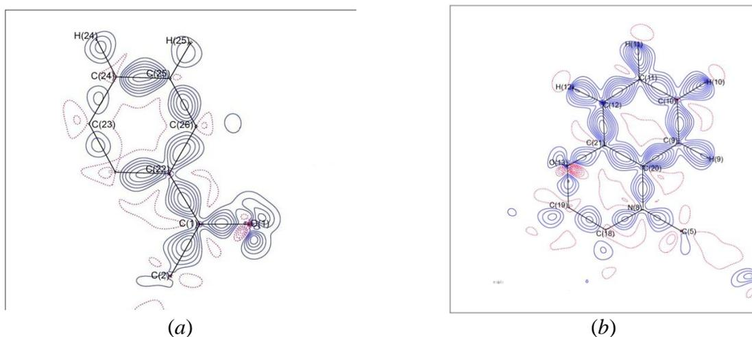
**Figure 14S.** Static deformation density maps for **PBO**: (a) the O(1)C(1)C(2) plane; (b) the O(13)C(20)C(21) plane. Blue solid line – the positive values, red dashed lines – the negative ones. Contours at  $\pm n \cdot 0.1 e \cdot \text{\AA}^{-3}$  ( $n = 0, 1, 2, \dots$ ).
