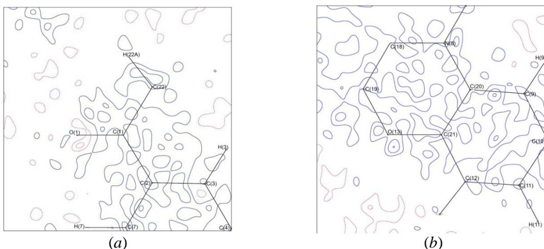
**Figure 3S.** Residual density maps for the **PAO** molecule: (a) the O(1)C(1)C(2) plane; (b) the O(13)C(20)C(21) plane. Blue solid line – the positive values, red dashed lines – the negative ones. Contours at  $\pm n \cdot 0.05 e \cdot \text{\AA}^{-3}$  ( $n = 1, 2, \dots$ ).
