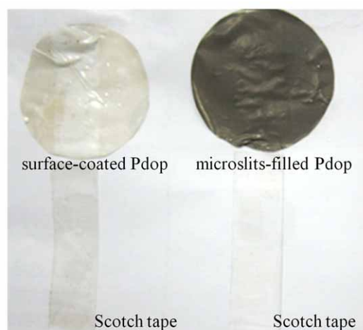
Fig 2S. Pdop modified porous PE films (surface coated and microslits-filled) after applying Scotch tape peeling test.
