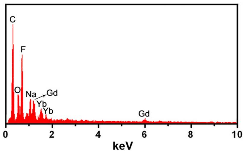
**Fig. S2** EDS spectrum of core-shell  $\text{Fe}_3\text{O}_4@ \text{NaGdF}_4:\text{Yb/Er}@ \text{NaGdF}_4:\text{Yb/Er}$  NCs.
