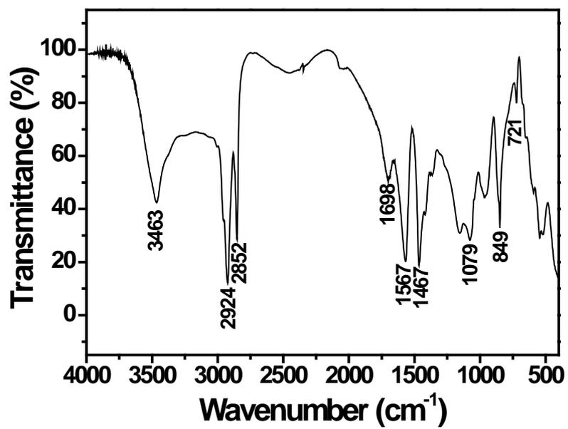
**Fig. S3** FT-IR spectrum of core-shell Fe<sub>3</sub>O<sub>4</sub>@NaGdF<sub>4</sub>:Yb/Er@NaGdF<sub>4</sub>:Yb/Er NCs.
