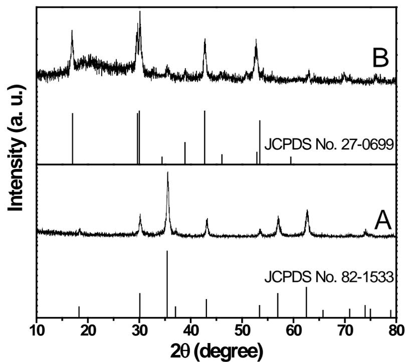
**Fig. S1** XRD patterns of the as-prepared  $\text{Fe}_3\text{O}_4$  core NCs (A) and core-shell  $\text{Fe}_3\text{O}_4@ \text{NaGdF}_4:\text{Yb}/\text{Er}@ \text{NaGdF}_4:\text{Yb}/\text{Er}$  NCs (B). The standard data for cubic  $\text{Fe}_3\text{O}_4$  phase (JCPDS no. 82-1533) and hexagonal  $\text{NaGdF}_4$  phase (JCPDS no. 27-0699) are shown as references.
