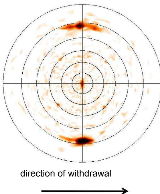
Figure S2: X-ray diffraction pole figure of a dip-coated film of the molecule DH3T (withdrawal velocity of  $50 \mu\text{m}/\text{sec}$ ) in respect to the direction of withdrawal. The measurement was performed at  $q = 26.0 \text{ nm}^{-1}$  to monitor the spatial distribution of the  $-606$  poles of DH3T crystallites. The strong features at  $\chi / \varphi = 73^\circ / 90^\circ$  and  $73^\circ / 270^\circ$  can be clearly assigned to the  $\alpha$ -phase.
