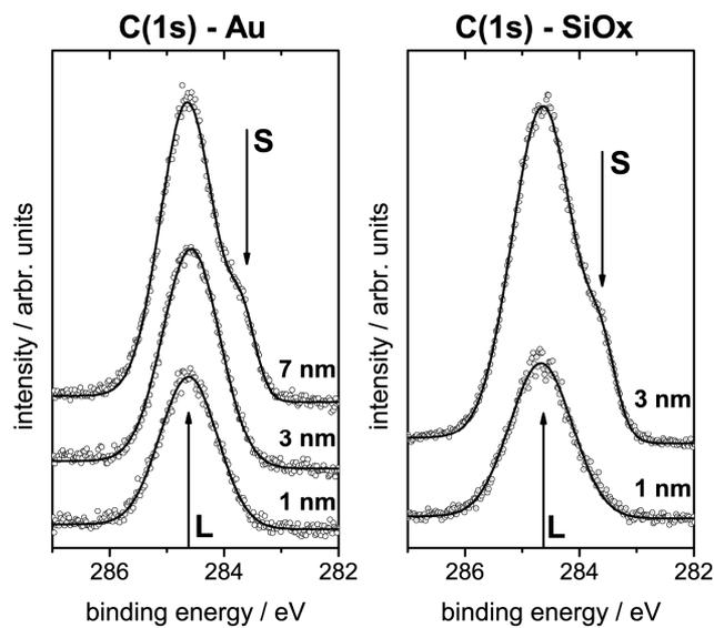
Figure S5: XPS-C(1s) results for DH3T thin films of different thickness prepared by physical vapour deposition on flame-annealed polycrystalline gold (left) and SiO<sub>x</sub> (right) substrates demonstrating an orientational transition from lying (L) to standing (S) DH3T upon subsequent growth.
