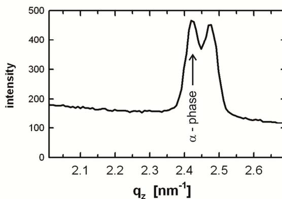
Figure S1: X-ray diffraction of a polycrystalline powder of the molecule dihexyl-terthiophene (DH3T) performed after heat treatment above the melting point.
