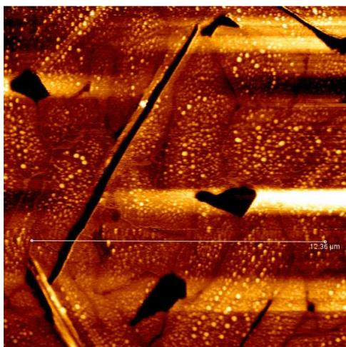
Figure S3: Atomic force microscopy micrograph of a vapour deposited film of DH3T with a layer thickness of 44nm. The image covers an area of 15 $\mu$ m x 15  $\mu$ m.
