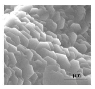
Figure S1. Cross sectional SEM image of ZnO:P nanoplatelets.
