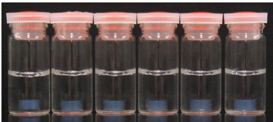
Fig. S6 The stability of boronate hydrogel ( \phi 8\text{ mm} \times 5\text{ mm} ) against pH. The boronate hydrogels were immersed in aqueous solutions (3 mL) of different pH values (from left to right: pH = 1, 3, 5, 7, 9, and 11) for three months at room temperature.
