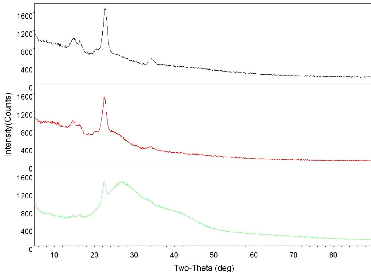
Figure S9. XRD pattern of Pt nanostructures on polypyrrole-coated cellulose fibers prepared using (a) 0.2882 M, (b) 5, and (c) 2.882 M of pyrrole.
