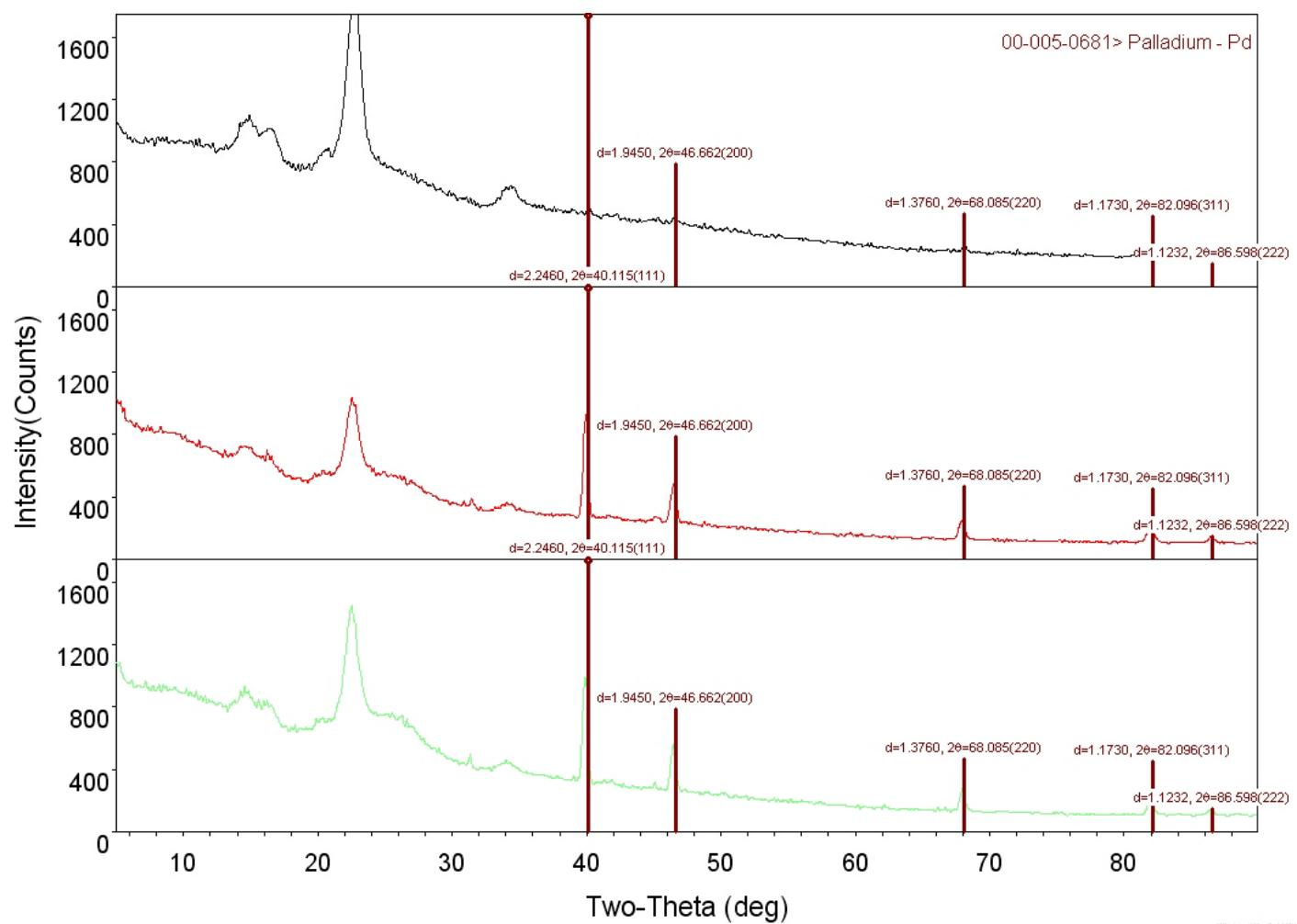
Figure S8. XRD patterns of Pd nanostructures on polypyrrole-coated cellulose fibers prepared using (a) 0.2882 M, (b) 1.441 M, and (c) 2.882 M of pyrrole.
