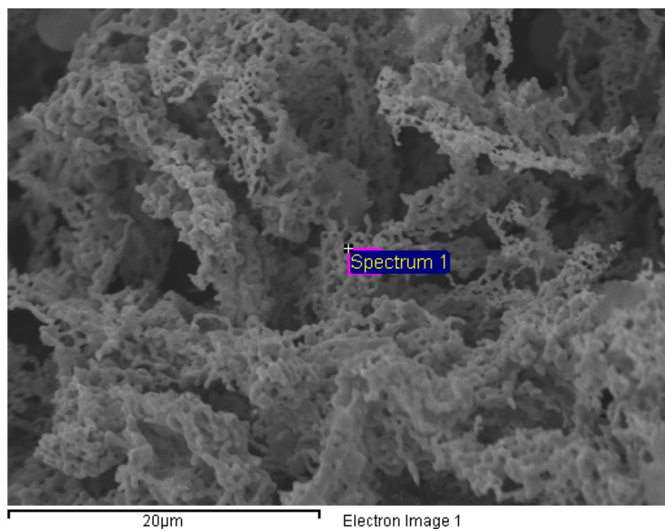
Figure S11. SEM image of autocatalytic reduced Pd on 5 ml polypyrrole coated after cellulose fibers after microwave ignition for 1 minute.
