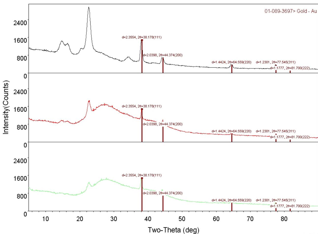
Figure S7. XRD pattern of Au nanostructures on polypyrrole-coated cellulose fibers prepared using (a) 0.2882 M, (b) 5, and (c) 2.882 M of pyrrole.
