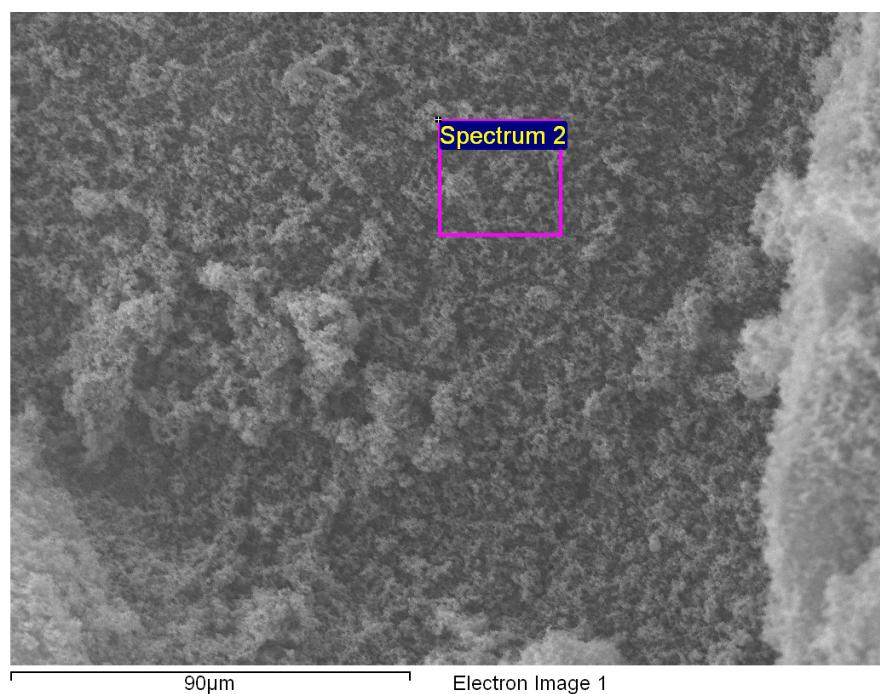
Figure S5. SEM image of self-assembled Pt nanoparticles on cellulose nanofibers, prepared using a high concentration of pyrrole (10 mL).
