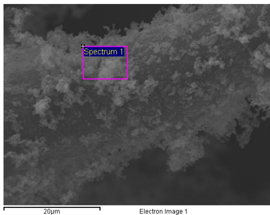
Figure S4. SEM image of self-assembled Pd nanoparticles on cellulose nanofibers, prepared using a medium concentration of pyrrole (5 mL).
