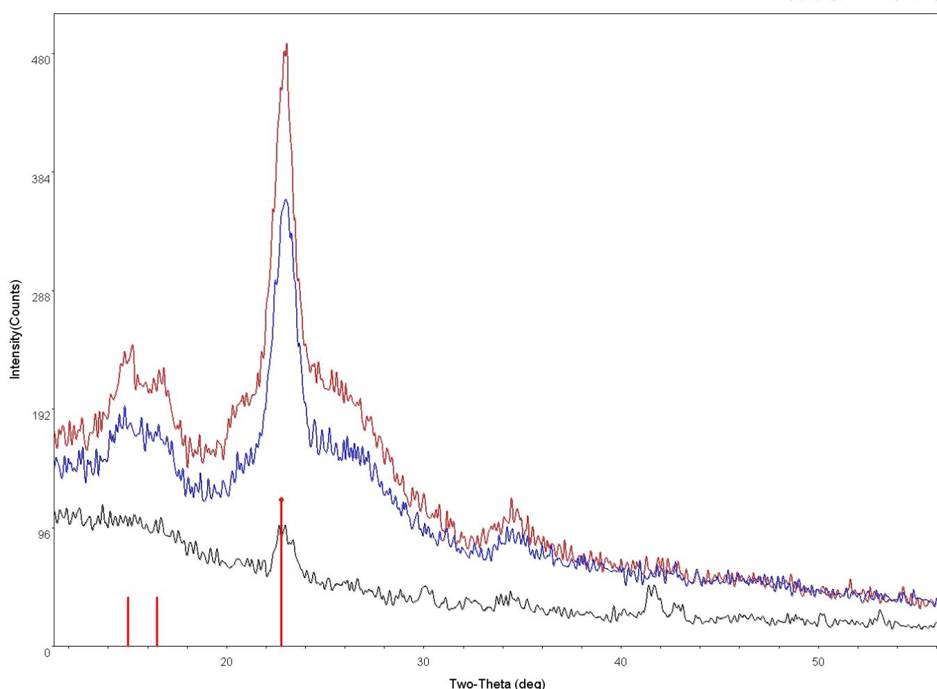
Figure S1. The XRD pattern of control cellulose sample, coated with Polypyrrole. Red line- 2.882 M, blue line-1.441 M, and black line-0.2882 M of pyrrole used for the reaction.
