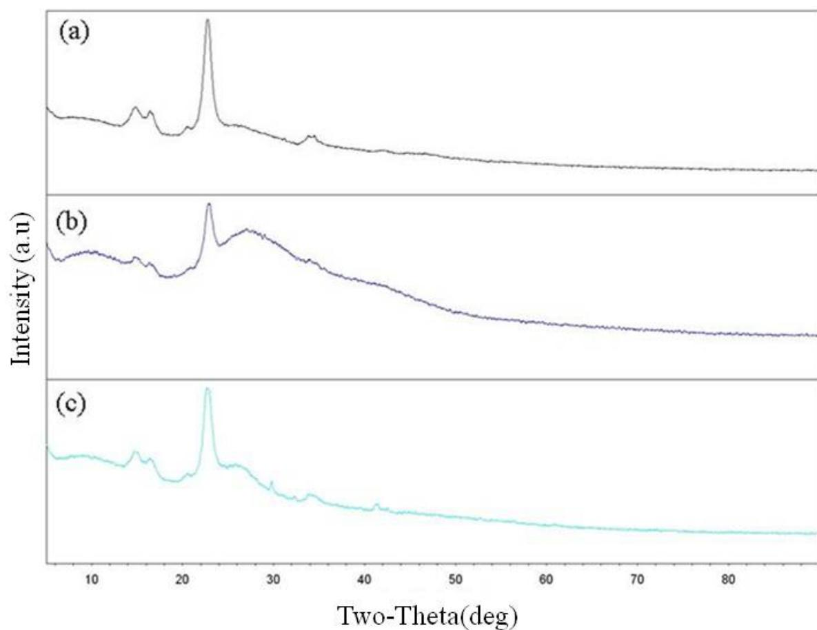
Figure S10. XRD patterns of iron nanoparticles formed on polypyrrole-coated cellulose fibers
