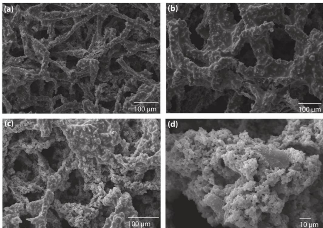
Figure S6. The decoration of Fe nanostrctures on cellulose nanofibers, prepared using (a) 0.2882 M, (b) 1.441 M, and (c-d) 2.882 M of pyrrole.
