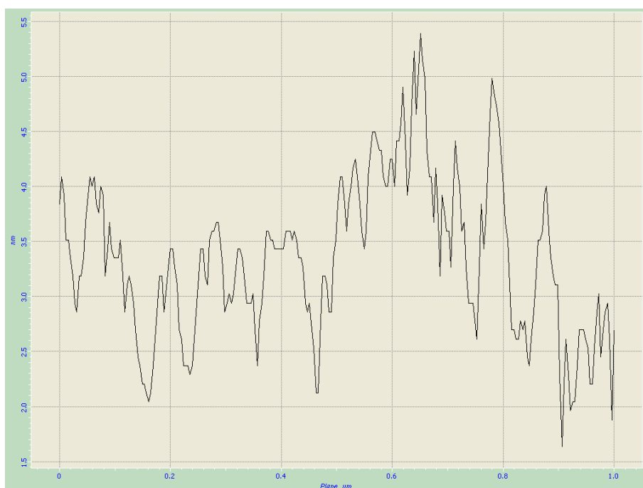
Fig. S2d Depth of pores of fresh SP2 along X axis.
