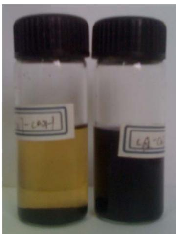
Fig. S1 CA-cMWCNTs (left) and a mechanic mixture of CA and cMWCNTs (right) in DMAc after half a month's standing.
