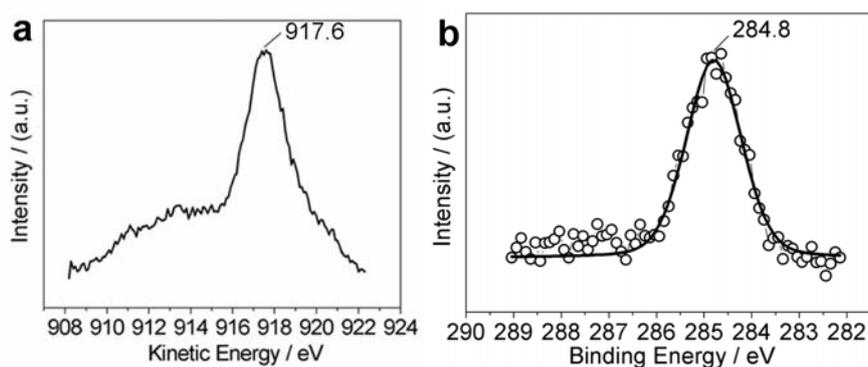
**Figure S4.** (a) Cu LMM Auger line and (b) C 1s XPS peak of the annealed NRs which mainly shows the hydrocarbon composition. The content of carbon species in this sample is determined to be only 5.9 at.%.
