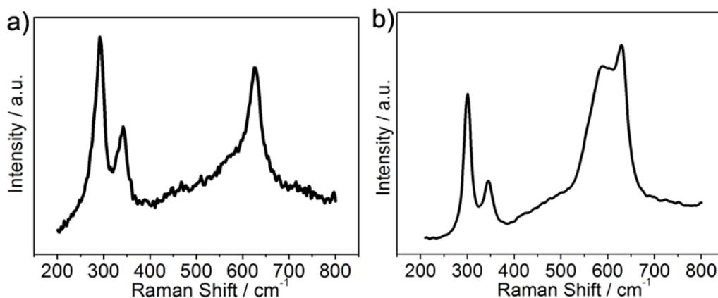
**Figure S7.** (a) Raman spectrum of the new-prepared CuO NRs, showing unobvious shoulder peak at  $592 \text{ cm}^{-1}$ . (b) Raman spectrum of the 5-day  $\text{O}_2$  exposed CuO NRs.
