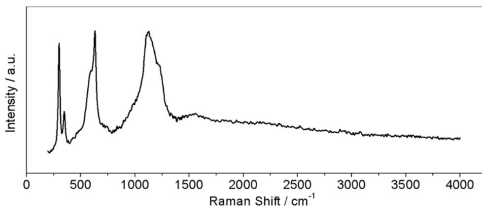
**Figure S8.** Full scan of Raman spectrum of the annealed CuO NRs, showing unobvious peak at  $3600 \text{ cm}^{-1}$  reflecting the characteristic of hydroxyl. The broad band above  $1100 \text{ cm}^{-1}$  should be derived from the contributions from two-phonon processes<sup>3</sup> and adsorbed oxygen.<sup>4</sup> Detailed discussion on the broad band is beyond the scope of this paper.
