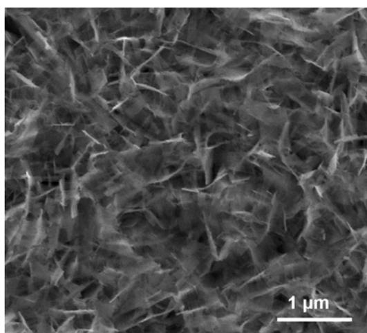
**Figure S2.** SEM image of a sample obtained via the corrosion of a Cu foil in a liquid membrane (wholly covering the substrate) of 1 M KOH for 5 days, demonstrating the formation of a flocc-like structure.
