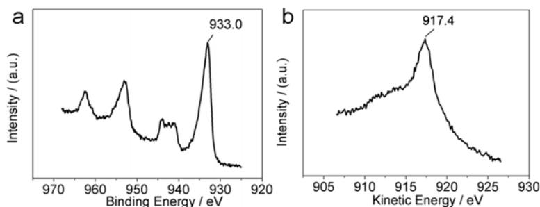
**Figure S10.** (a) Cu 2p photoelectron line and (b) Cu LMM Auger line of the octadecane-adsorbed CuO NRs after 5-days exposure to  $O_2$  at room temperature.
