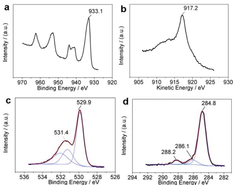
**Figure S6.** XPS of the new-prepared NRs without annealing. (a) Cu 2p photoelectron line. (b) Cu LMM Auger line. (c) O 1s photoelectron line. (d) C 1s photoelectron line. The content of the detected carbon species by XPS is 39.8 at.%.
