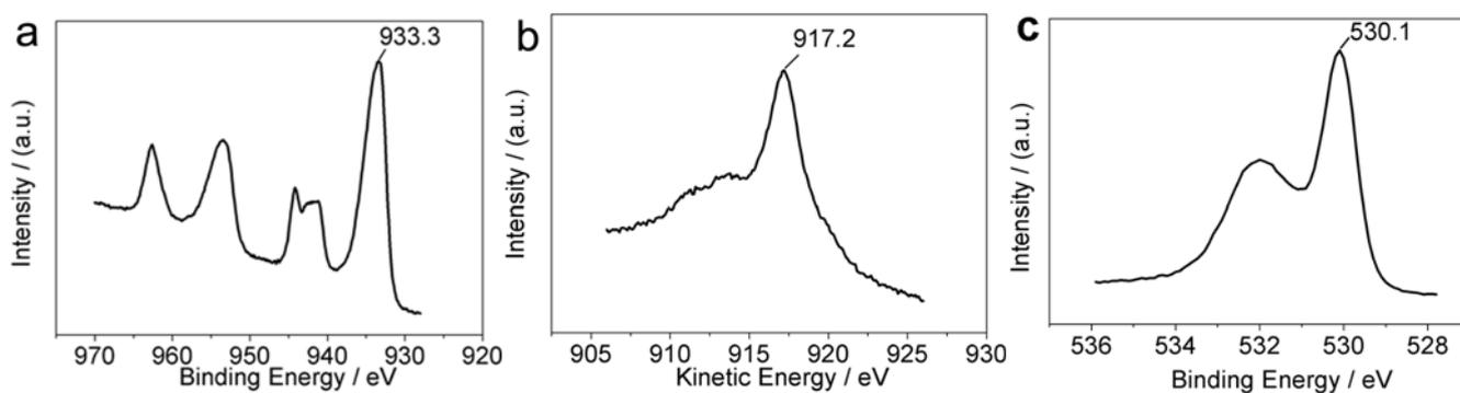
**Figure S9.** (a) Cu 2p photoelectron line, (b) Cu LMM Auger line, and (c) O 1s photoelectron line of the NRs after exposure to CO at 60 °C for 5 days. The ratio of  $O_{\text{lattice}} 1s/Cu 2p3$  is measured to be 0.96, showing the CuO as the dominant composition of the surfaces of the NRs.
