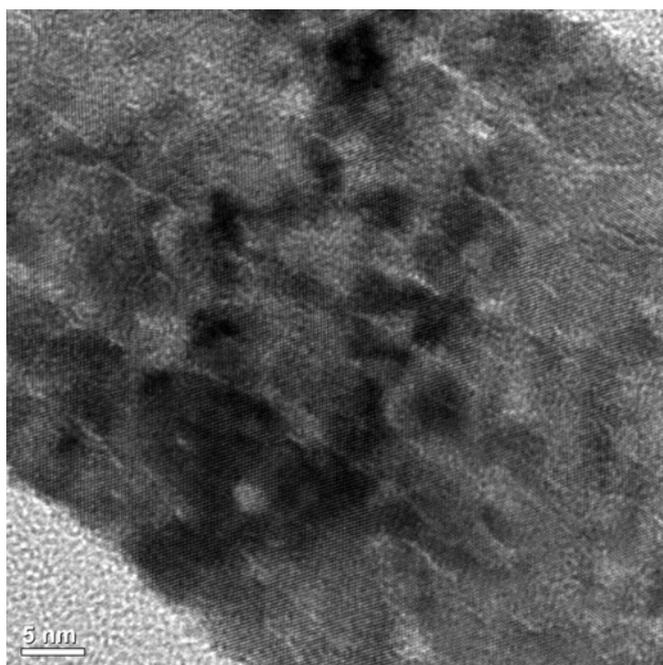
**Figure S1.** HRTEM image of the CuO NRs without annealing, which clearly shows that many grain boundaries are formed in the structures.
