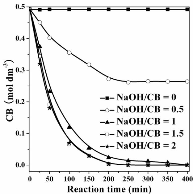
**Fig. S4.** Effect of NaOH/CB molar ratio on the CB concentration over  $2.5\text{Ni}/\text{C}$  catalyst.
