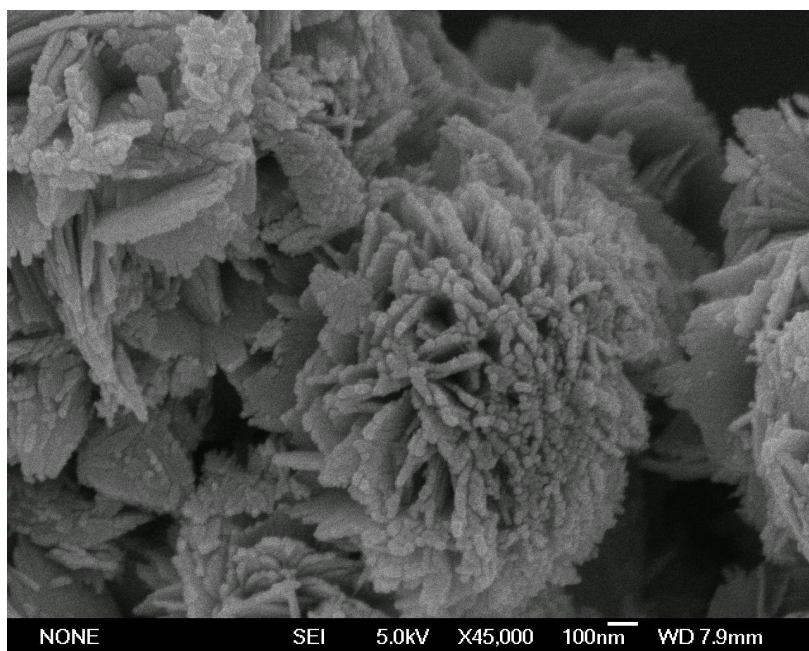
Fig. S5 SEM image of flower-like CuO after cycling test at various rates.
