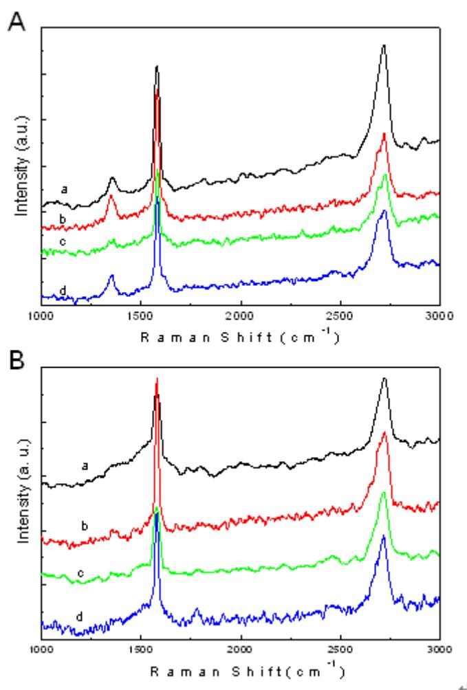
**Figure S6.** Raman spectra of individual graphene sheets deposited from solution on holey carbon TEM grids. (A) Raman spectra of graphene sheets by non-covalent functionalization of pyrene-PEG<sub>2K</sub> (a,b) and pyrene-PEG<sub>5K</sub> (c,d), respectively. (B) Raman spectra of graphene sheets by non-covalent functionalization of pyrene-PCL<sub>19</sub> (a,b) and pyrene-PCL<sub>48</sub> (c,d), respectively.
