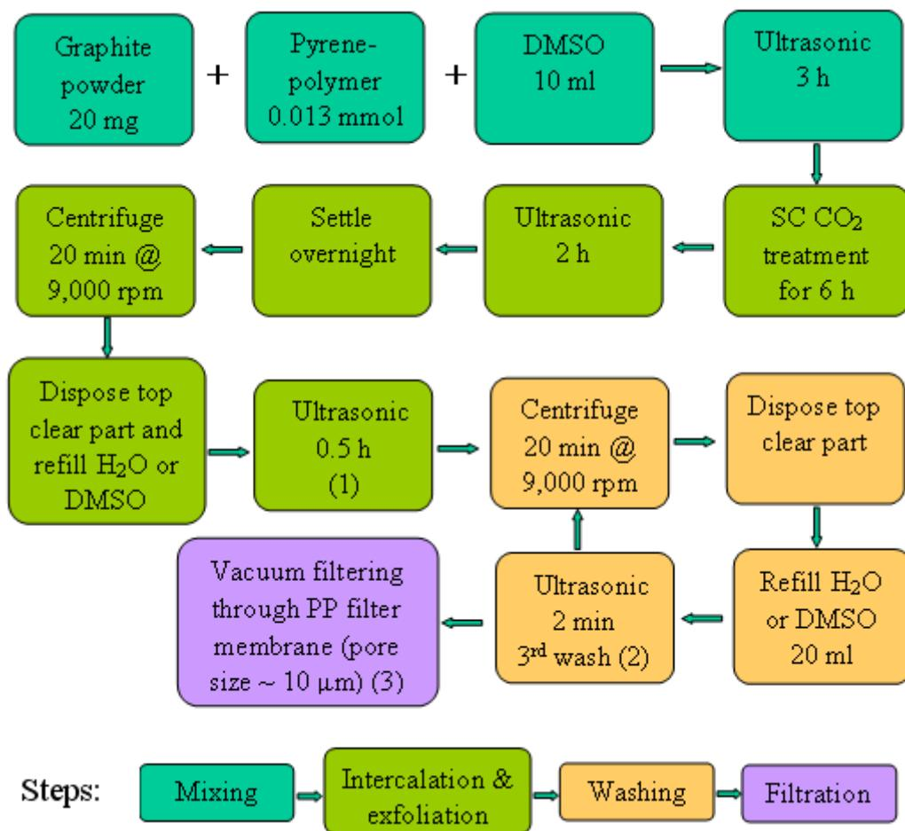
**Figure S3.** Process flow of intercalation and exfoliation of graphite with different steps (mixing, intercalation & exfoliation, washing and filtration) indicated in color key. (1)-(3) represent the stage 1-3, respectively.
