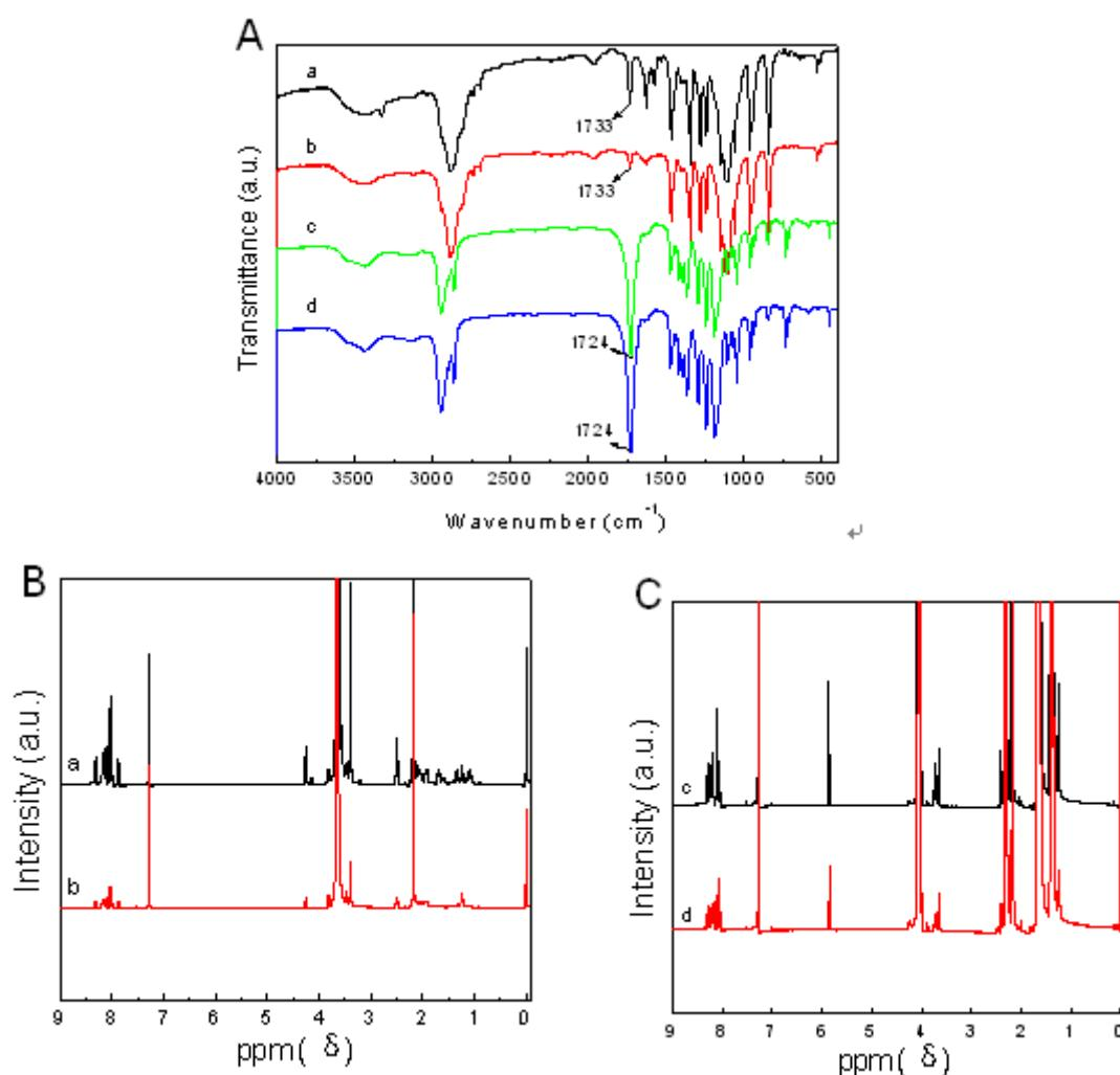
**Figure S1.** (A) FT-IR spectra of (a) pyrene-PEG<sub>2K</sub>, (b) pyrene-PEG<sub>5K</sub>, (c) pyrene-PCL<sub>19</sub> and (d) pyrene-PCL<sub>48</sub>, (B)  $^1\text{H}$  NMR spectra of (a) pyrene-PEG<sub>2K</sub> and (b) pyrene-PEG<sub>5K</sub>, and (C)  $^1\text{H}$  NMR spectra of (c) pyrene-PCL<sub>19</sub> and (d) pyrene-PCL<sub>48</sub>.
