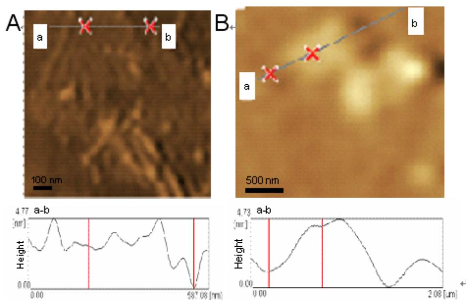
**Figure S4.** Tapping mode AFM images and topographic height profiles of graphene sheets by non-covalent functionalization of pyrene-PEG<sub>2K</sub> (A) and pyrene-PCL<sub>19</sub> (B) on Si surface, respectively.
