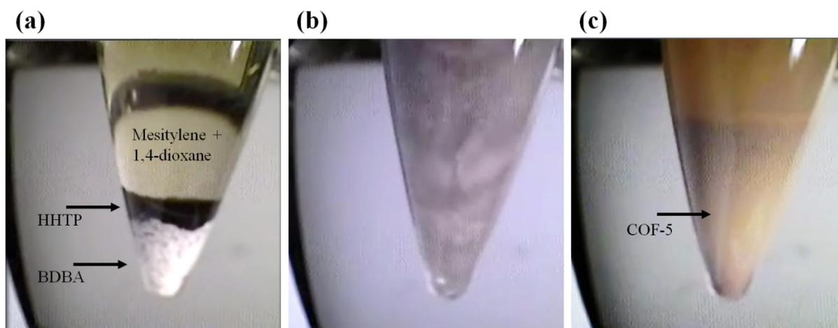
**Fig. S5.** Video Capture images of COF-5 sonochemical synthesis; (a) setup, (b) applying sonication, and (c) after reaction (top portion in (a) is the reflected image of HHTP).
