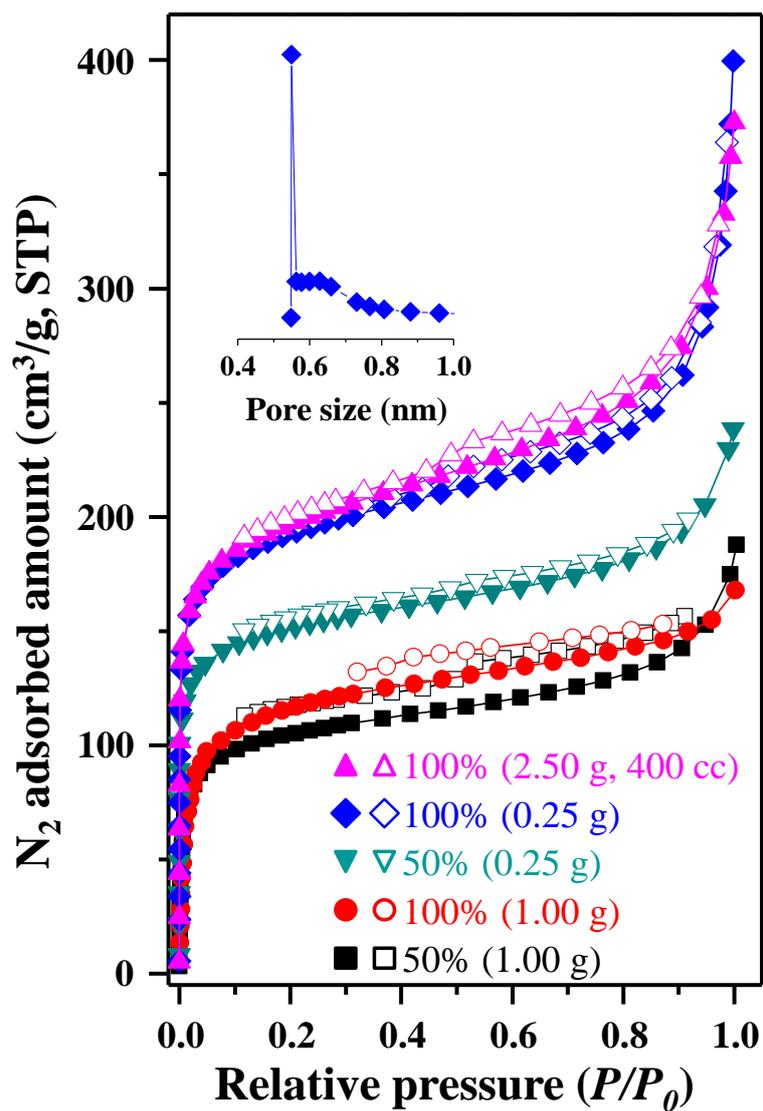
**Fig. S4.** N<sub>2</sub> adsorption-desorption isotherms of the COF-1 samples (inset is the pore size distribution of COF-1 sample of entry 4 in Table 1): ■□ (entry 1 in Table 1); ●○ (entry 2); ▼▽ (entry 3); ◆◇ (entry 4); and ▲△ (entry 5).
