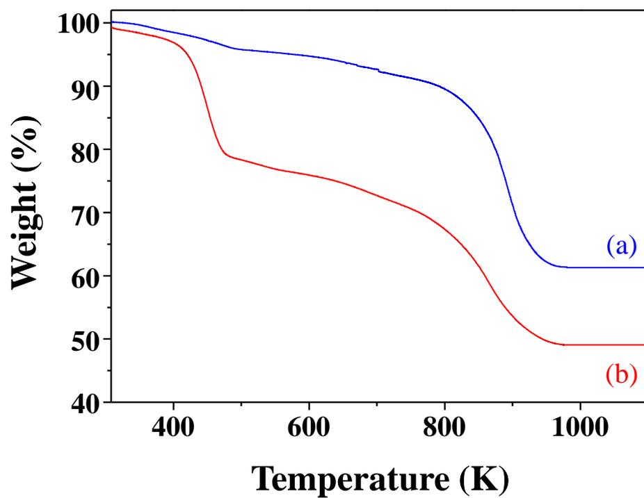
**Fig. S3.** Thermogravimetric analysis of the COF-1 sample: (a) washed with acetone ( $2 \times 50$  mL $\times 10$ ) and dried at 353 K overnight and (b) as-synthesized (acetone washed once and dried).
