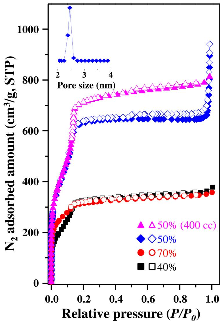
**Fig. S7.** N<sub>2</sub> adsorption-desorption isotherms of the COF-5 samples (inset is the pore size distribution of COF-5 sample of entry 8 in Table 1): ■□ (entry 6 in Table 1); ◆◇ (entry 8); ●○ (entry 12); ▲△ (entry 14).
