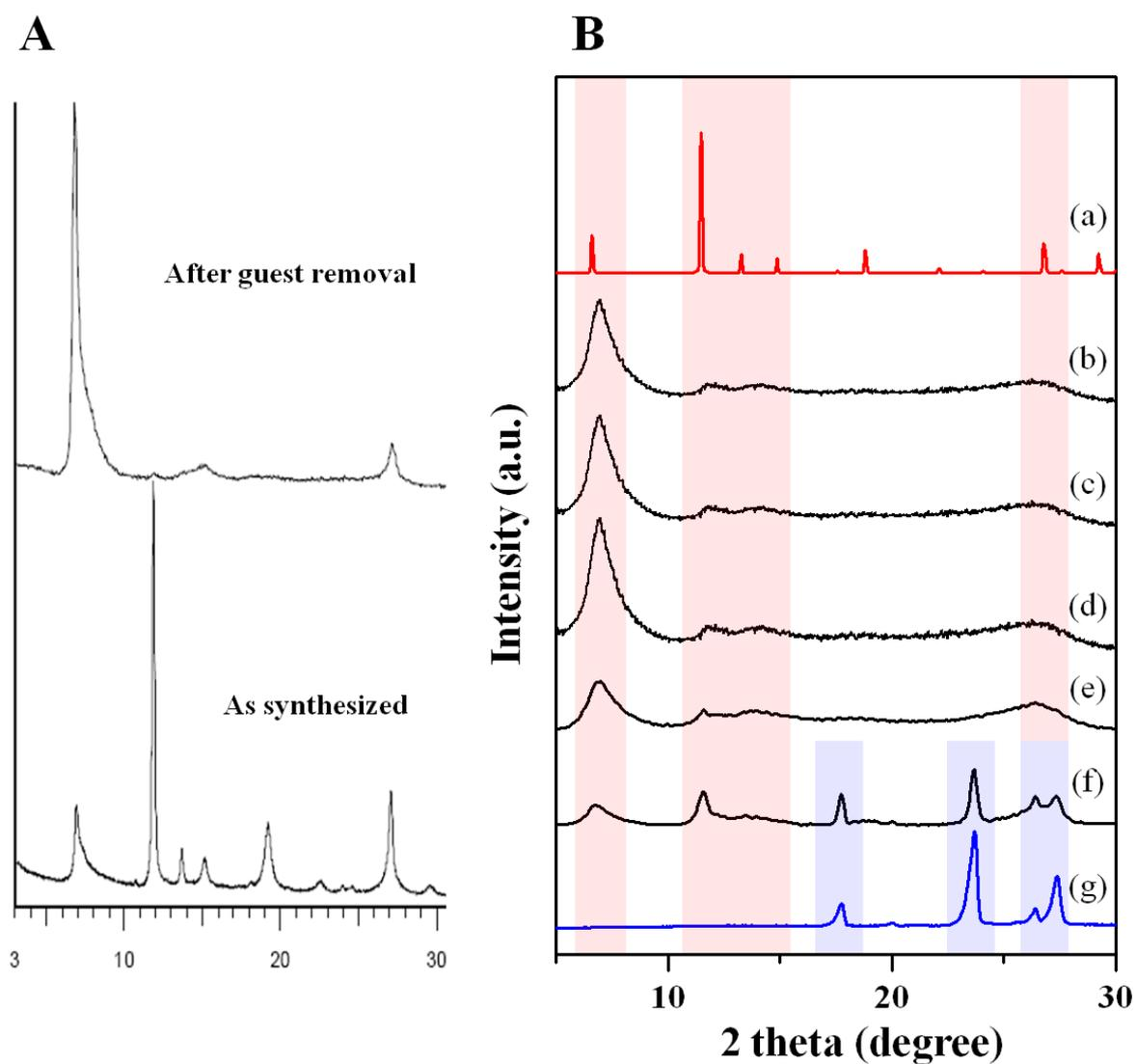
**Fig. S2.** XRD patterns; (A) experimental data of COF-1 XRD patterns before and after activation in the literature,<sup>§</sup> and (B) COF-1 simulated (a), COF-1 samples in Table 1 of (b) entry 5, (c) entry 4, (d) entry 3, (e) entry 2, and (f) entry 1, and (g) BDBA.
