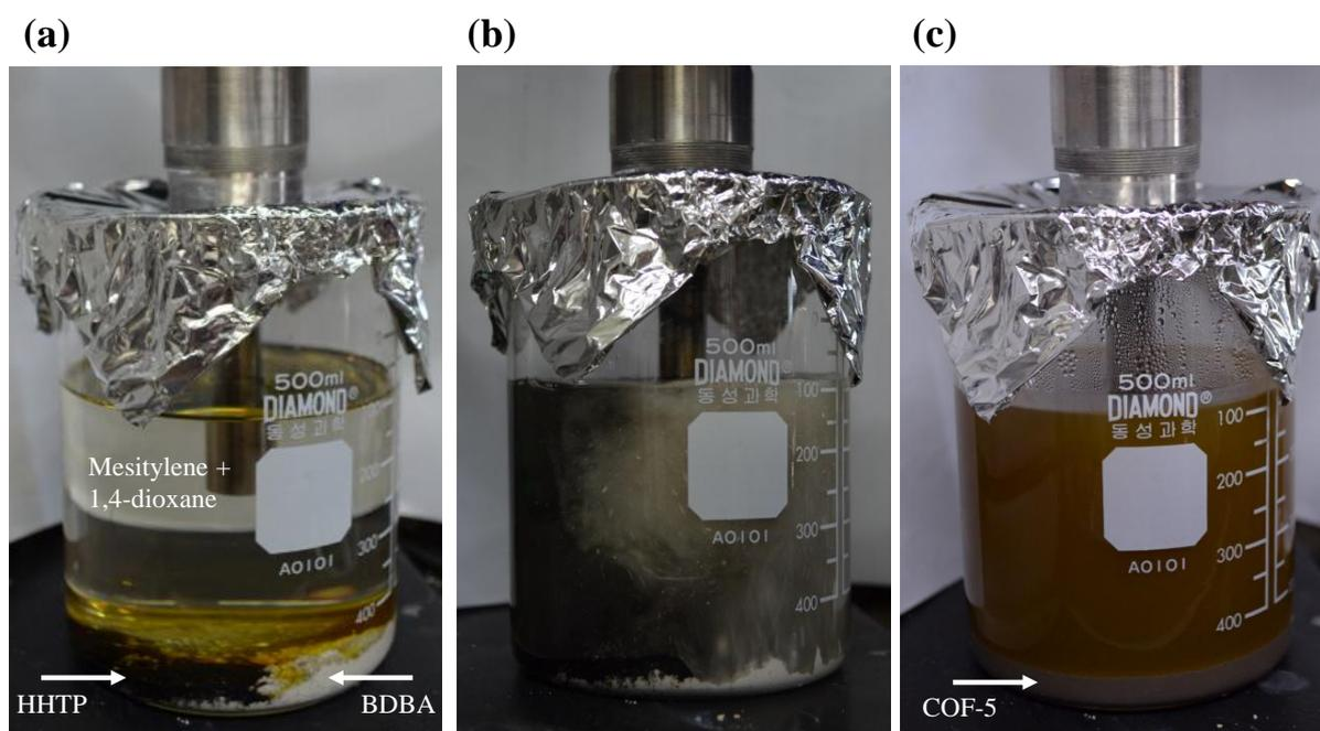
**Fig. S10.** COF-5 sonochemical synthesis procedures in a 0.5 L-batch (entry 14 in Table 1); (a) setup, (b) applying sonication, and (c) after reaction.
