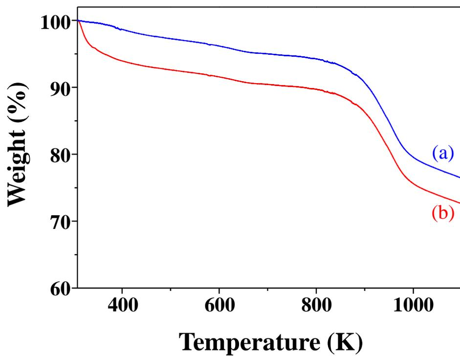
**Fig. S8.** Thermogravimetric analysis of the COF-5 sample: (a) washed with acetone ( $2 \times 50$  mL $\times 10$ ) and dried at 353 K overnight and (b) as-synthesized (acetone washed once and dried).
