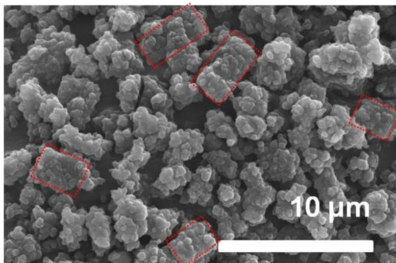
**Fig. S9.** SEM image of the COF-5 samples (entry 10 in Table 1, red rectangle: BDBA morphology).
