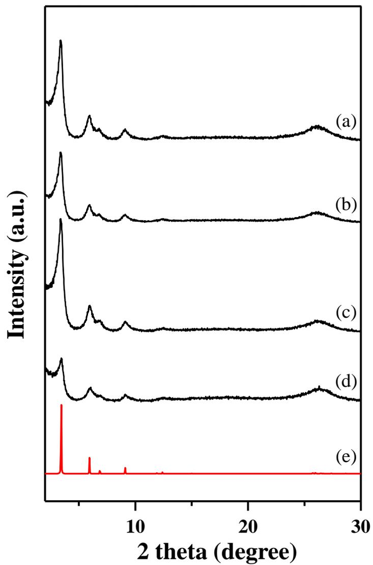
**Fig. S6.** XRD patterns after guest removal; (a) entry 14 in Table 1, (b) entry 12, (c) entry 8, and (d) entry 6 of COF-5 samples, and (e) simulated COF-5.
