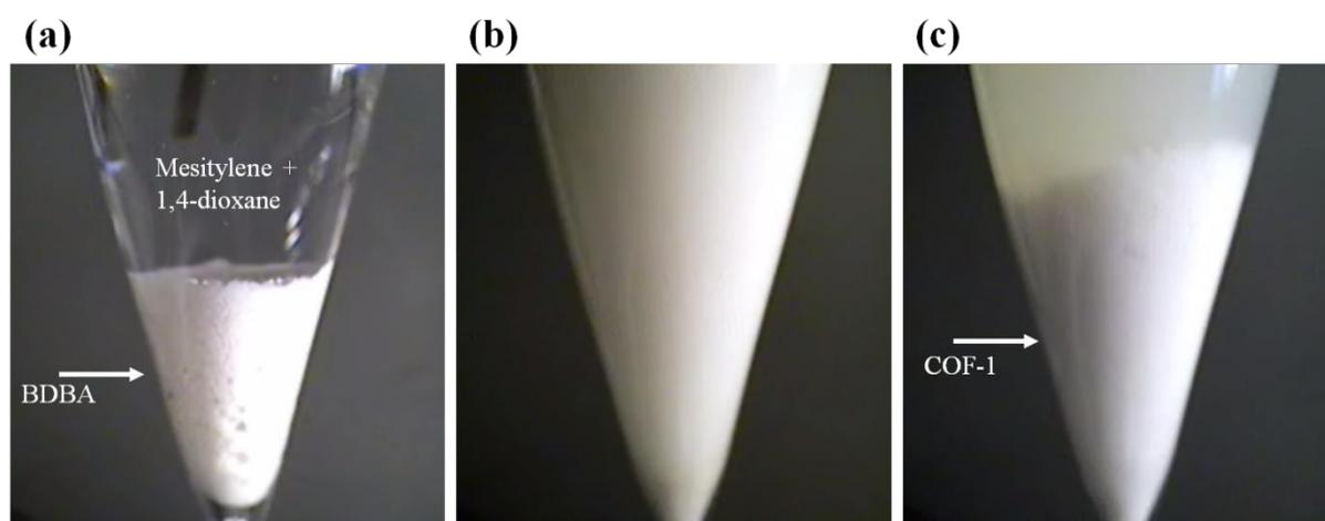
**Fig. S1.** Video Capture images of COF-1 sonochemical synthesis; (a) setup, (b) applying sonication, and (c) after the reaction.
