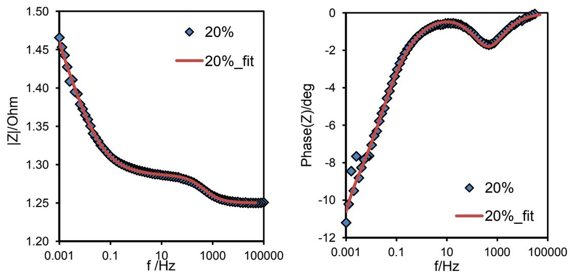
Fig. S7 Bode plots for AC cathode with 20% PTFE and the fitting curves with the equivalent circuit
