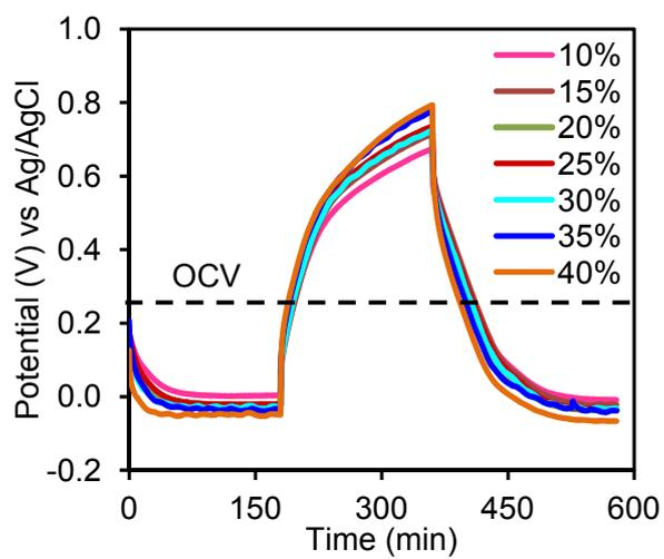
Fig. S8 Charge-discharge diagram for AC cathodes with different PTFE binder contents (10, 15, 20, 25, 30, 35, 40%, No DL, 43 mg/cm<sup>2</sup> AC)
