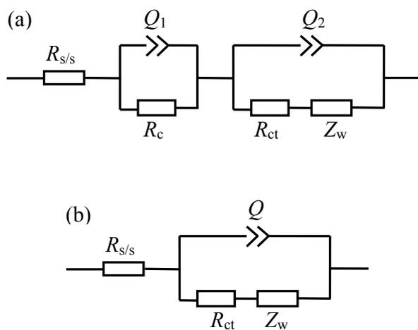
Fig. S1 Equivalent circuits for EIS spectra with (a) AC cathodes and (b) Pt/C cathodes.
