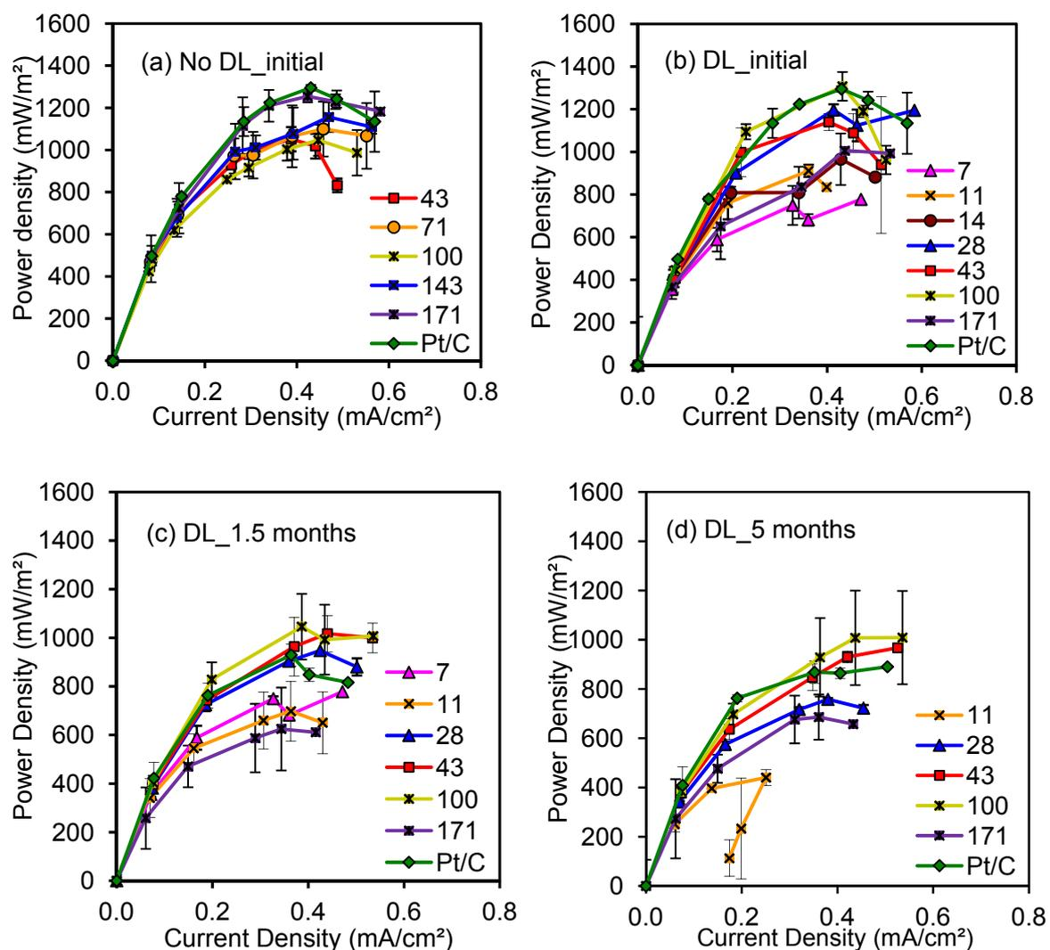
Fig. S3 Power generation obtained using (a) AC cathodes (43, 71, 100, 143, 171 mg/cm<sup>2</sup> AC, 10% PTFE) without DL, Pt/C cathodes in the initial cycles; (b) AC cathodes (7, 11, 14, 28, 43, 100, 171 mg/cm<sup>2</sup> AC, 10% PTFE) with DL, Pt/C cathodes in the initial cycles; (c) AC cathodes (7, 11, 28, 43, 100, 171 mg/cm<sup>2</sup> AC, 10% PTFE) with DL, Pt/C cathodes after 1.5 months; (d) AC cathodes (11, 28, 43, 100, 171 mg/cm<sup>2</sup> AC, 10% PTFE) after 5 months
