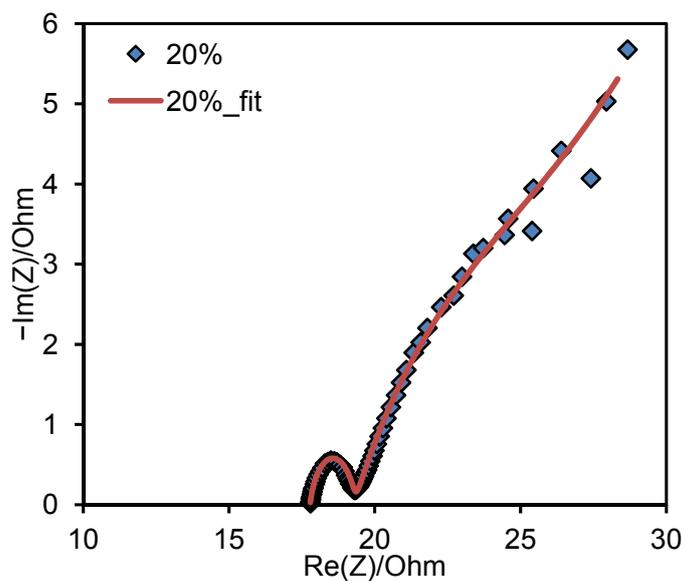
Fig. S6 An example of Nyquist plots for AC cathode (with 20% PTFE content) and the fitting curve with equivalent circuit
