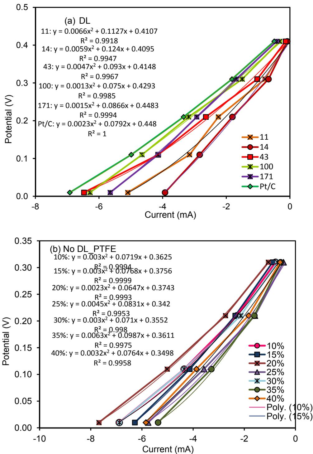
Fig. S5 Regressions for cathode current-voltage curves using (a) AC cathodes (11, 14, 43, 100, 171 mg/cm<sup>2</sup> AC, 10% PTFE) with DL and Pt/C cathodes; (b) AC cathodes (10, 15, 20, 25, 30, 35, 40, 43 mg/cm<sup>2</sup> AC) without DL
