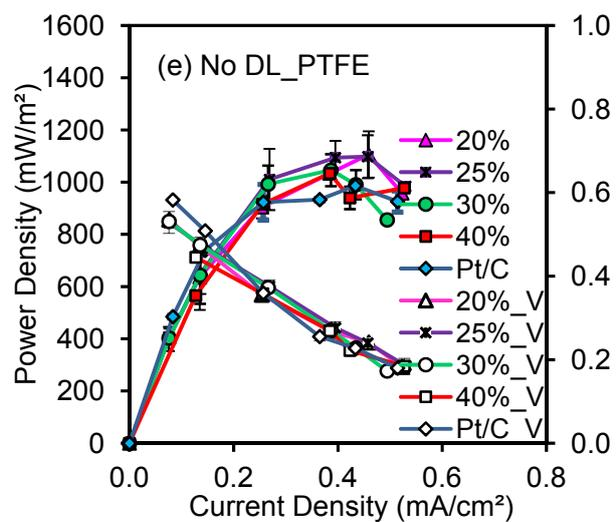
Fig. S4 Power generation obtained using AC cathodes (20, 25, 30, 35, 40% PTFE, 43 mg/cm<sup>2</sup> AC) without DL, Pt/C cathodes after 1 month
