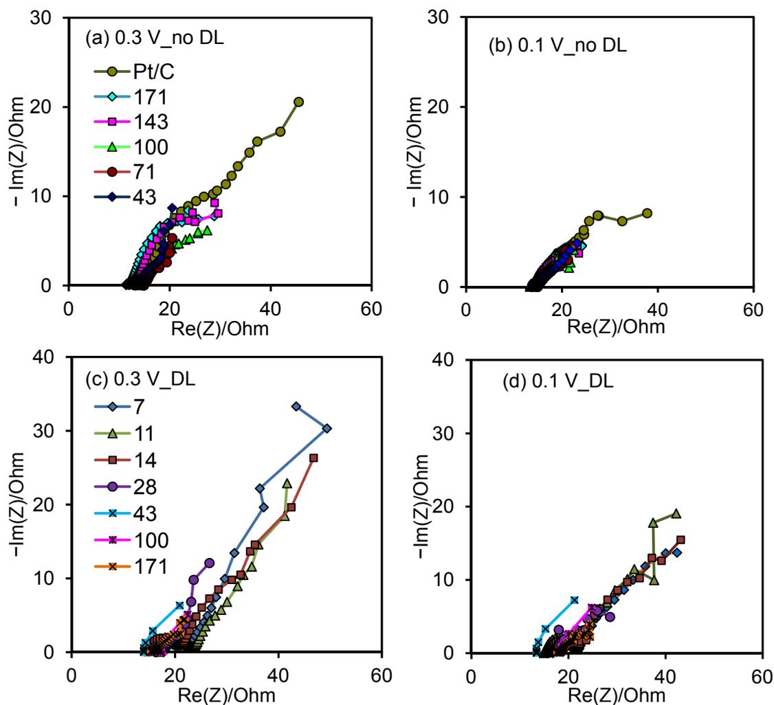
Fig. S2 Nyquist plots of ac air cathodes (a) at 0.3 V, (b) at 0.1 V using 43, 71, 100, 143, 171 mg/cm<sup>2</sup> AC, 10% PTFE without DL; (c) at 0.3 V, (d) at 0.1 V using 7, 11, 14, 28, 43, 100, 171 mg/cm<sup>2</sup> AC, 10% PTFE with DL.
