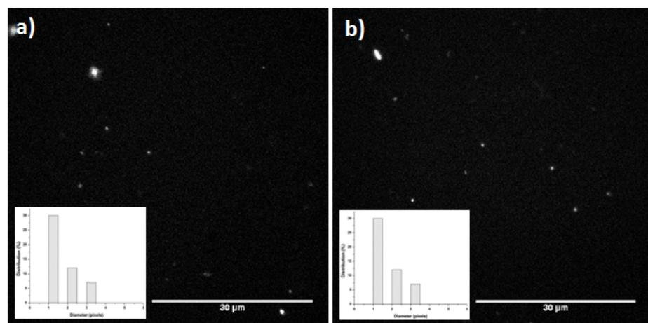
**Supplementary Figure S9:** The diameter of fluorescence signals from nanoparticles dispersed on cover-glass visualised using 470 nm excitation / 620 nm emission **a)** citric acid coated ( $\text{Y}_{0.96}\text{Eu}_{0.04}\text{OOH}$ ) nanoparticles **b)** citric acid coated ( $\text{Y}_{0.96}\text{Eu}_{0.04}\text{O}_3$ ) nanoparticles (insets show the measured diameter of fluorescence signals).
