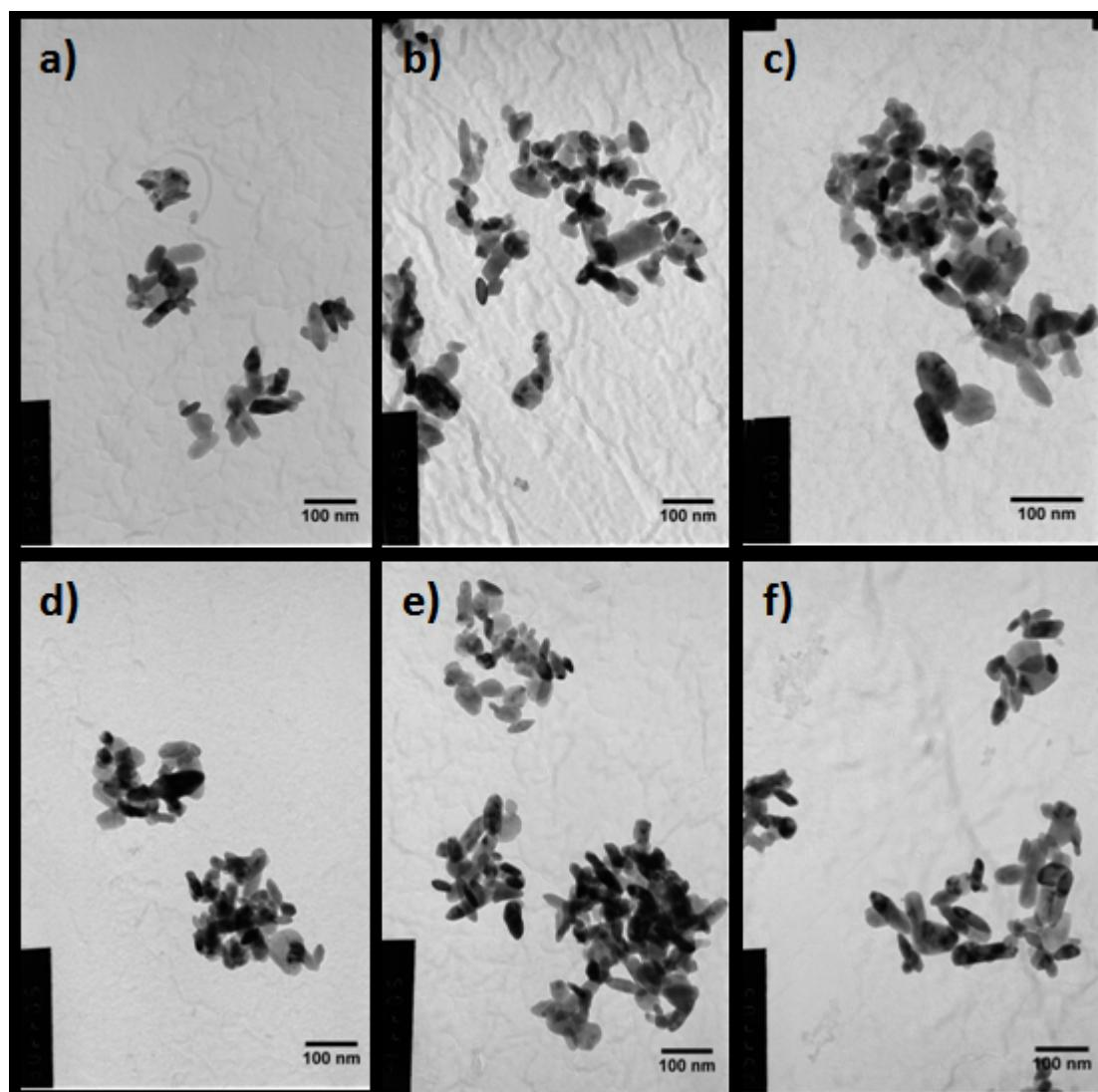
**Supplementary Figure S6:** TEM images of  $(Y_{0.96}Eu_{0.04})OOH$  phosphor nanoparticles heat treated at 500 °C for **a)** 60 s **b)** 180 s **c)** 300 s **d)** 600 s **e)** 1200 s **f)** 1800 s (Images were captured using JEOL 100CX)
