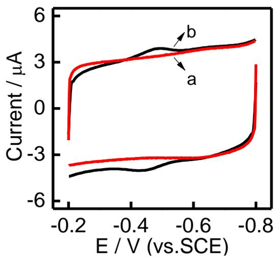
**Figure S9.** CV curves of CYP3A4/CPR-microsomes/PDDA/Au/PDDA/G modified GCE in 0.1 M PBS, pH 7.4 at  $100 \text{ mV s}^{-1}$ . (a) Nitrogen saturated, (b) air saturated, and (c) with the addition of  $46 \mu\text{M}$  nifedipine to air saturated buffer solution.
