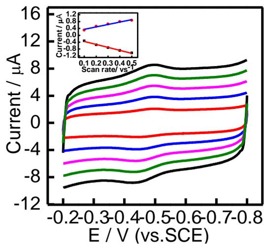
**Figure S8.** CV curves obtained at (a) PDDA/G and (b) CYP3A4/CPR-microsomes/PDDA/G modified GCE at a scan rate of  $100 \text{ mV s}^{-1}$  in anaerobic  $0.1 \text{ M}$  PBS, pH 7.4.
