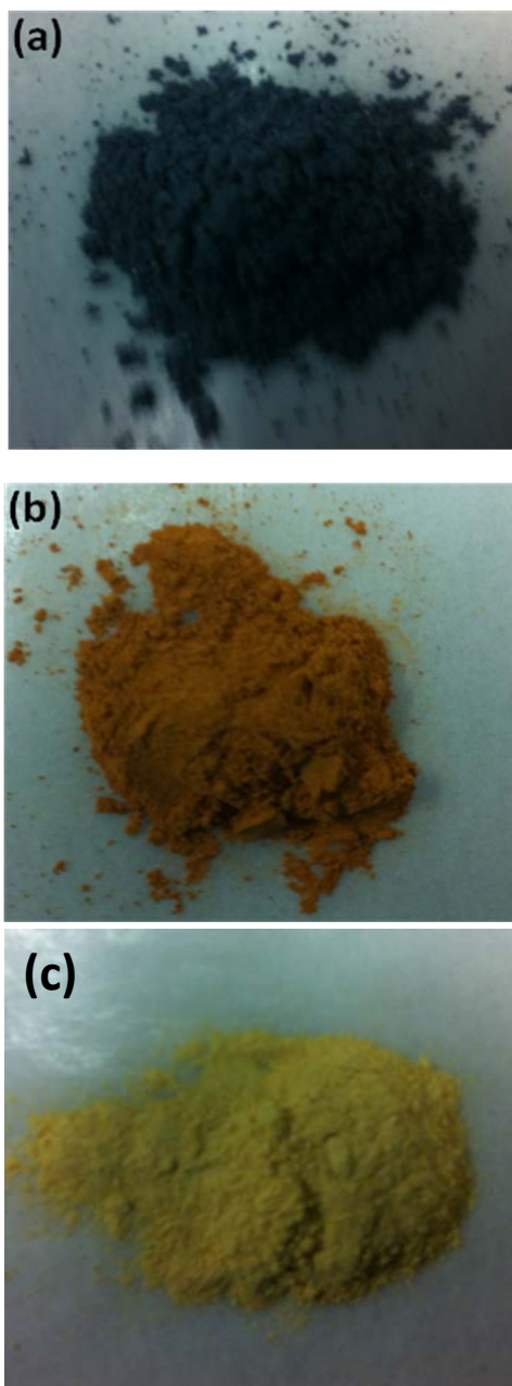
Fig. S2 Appearance of the BCZGP x=0.1 sample (a) as-prepared (b) after exposure to pure \text{CO}_2 at 600 °C for 24 h (c) after exposure to \text{H}_2\text{O} vapour treatment for 24 h at ~90 °C.
