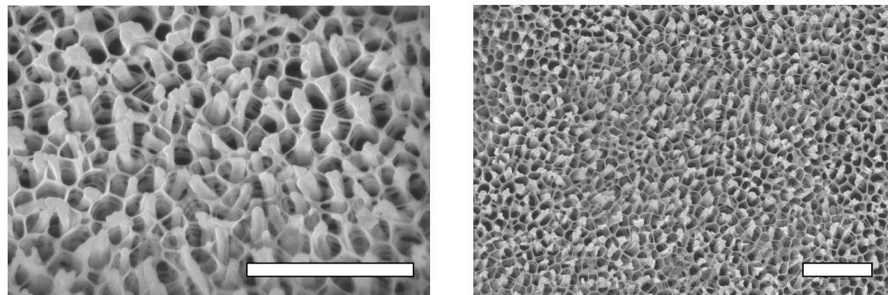
**Fig. ESI2** SEM images of PEDOT inverse-nanotube array formed in titania nanotubes (Fig. ESI1) with pulse current protocol at 1.0 mA anodic pulse (10ms) followed by cathodic pulse at -1.0 mA (4ms) and rest current at 0 mA (500ms). Titania nanotubes were dissolved for polymer structure observation. The scale bars at the bottom represent 1μm.
