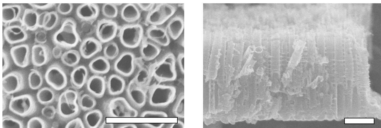
**Fig. ESI1** SEM images of titania nanotubes formed in glycerol-water electrolyte (55:45 v/v) containing ammonium fluoride (0.27 M) at 30V for 3h. The tubes were annealed for 3h in Ar atmosphere at 450°C. The scale bars at the bottom represent 500nm.
