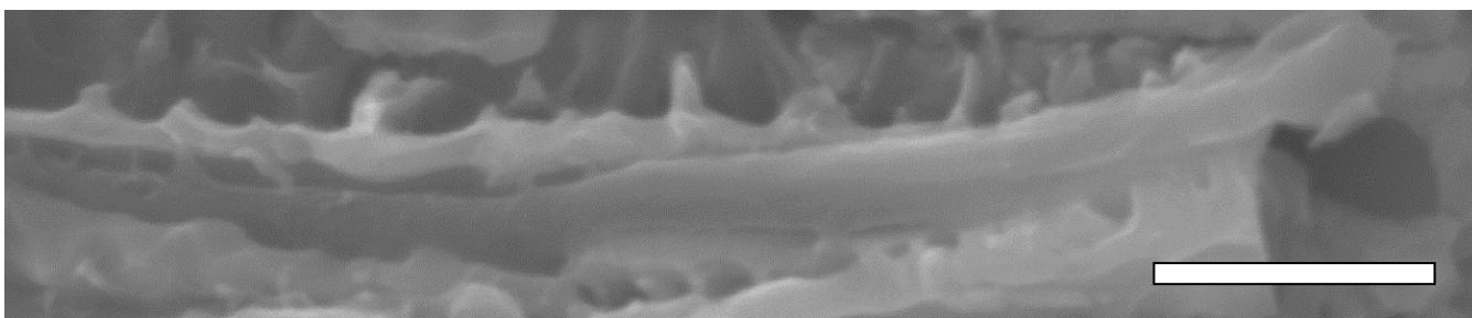
**Fig. ESI3** The image shows single PEDOT nanowire which was filled inside titania nanotube. The brightest parts on the picture represent broken titania nanotube. The polymer was deposited with protocol at 0.85 mA anodic pulse (10ms) followed by cathodic pulse at -0.85 mA (4ms) and rest current at 0 mA (500ms). The scale bar at the bottom represents 200 nm.
