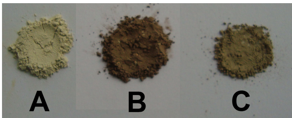
Figure S10. Photo graphs of pure \text{Bi}_2\text{O}_3 , \text{Bi}_2\text{O}_3/\text{Bi}_2\text{O}_{3+x} composite and \text{Bi}_2\text{O}_3/\text{Bi}_2\text{O}_{3+x} composite after the photo catalytic degradation of MO for 6 h visible light reaction illustrating photo stability.
