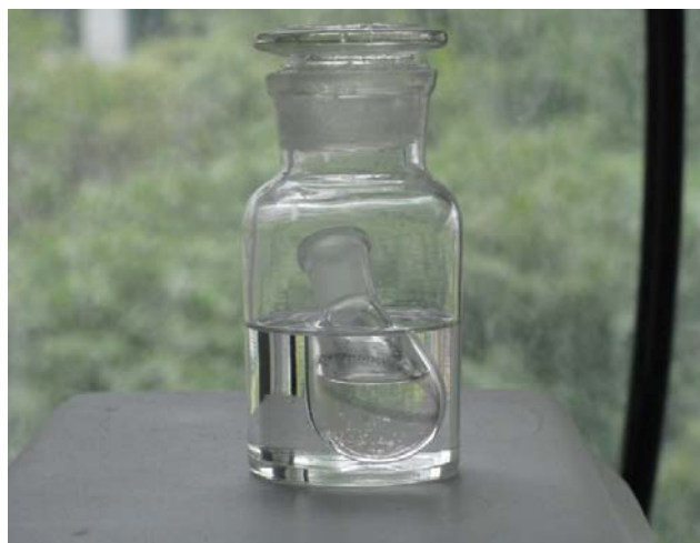
Figure S6. Apparatus for crystallization of 2a & 2b
