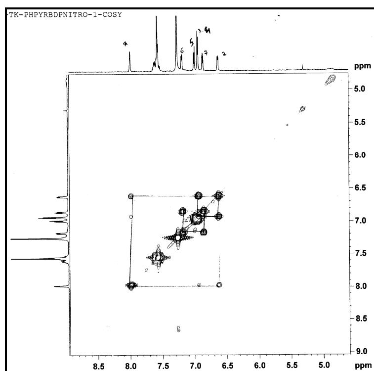
**Figure 20:**  $^1\text{H}$ - $^1\text{H}$  COSY NMR spectrum of compound 7 recorded in  $\text{CDCl}_3$
