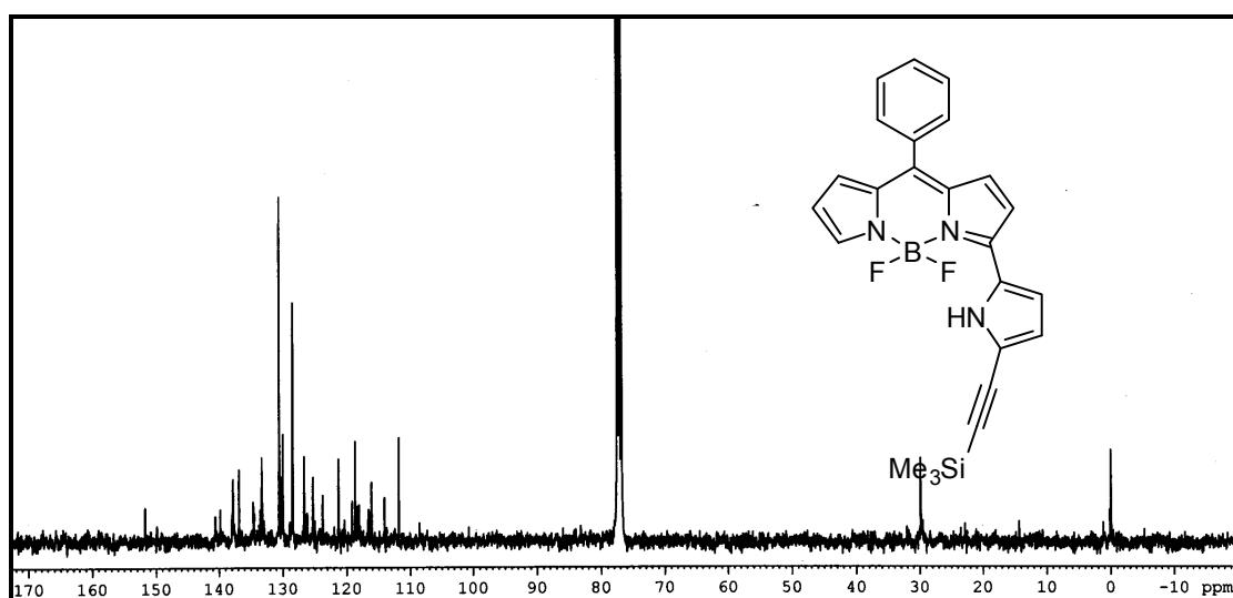
Figure 29:  $^{13}\text{C}$  NMR spectrum of compound 8 recorded in  $\text{CDCl}_3$
