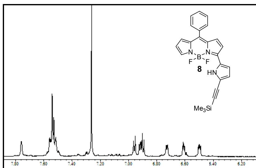
**Figure 25:** <sup>1</sup>H NMR spectrum of compound **8** in the selected region recorded in CDCl<sub>3</sub> ( $\delta$  in ppm)
