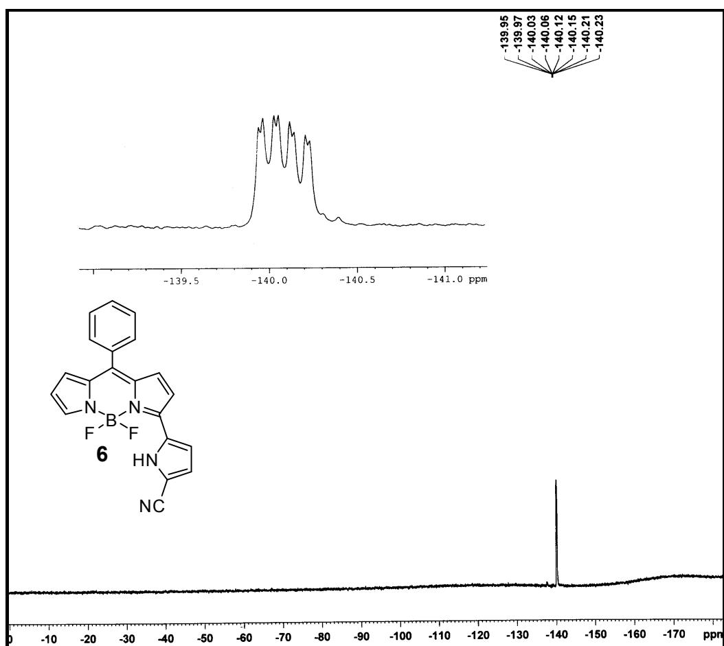
Figure 15:  $^{19}\text{F}$  NMR spectrum of compound 6 recorded in  $\text{CDCl}_3$
