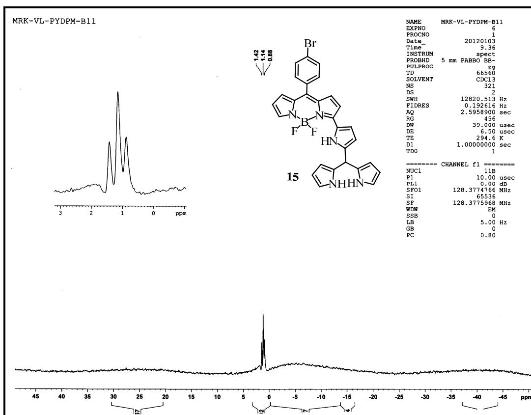
Figure 57 : <sup>11</sup>B NMR spectrum of compound 15 recorded in CDCl<sub>3</sub>.
