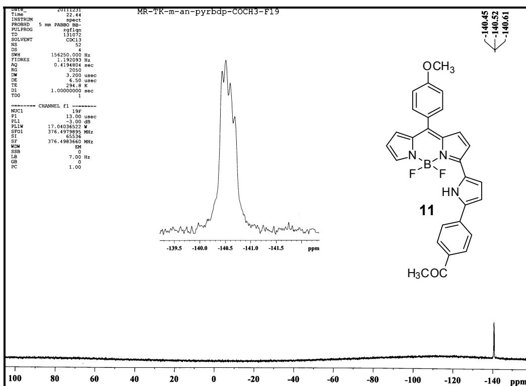
Figure 39:  $^{19}\text{F}$  NMR spectrum of compound **11** recorded in  $\text{CDCl}_3$
