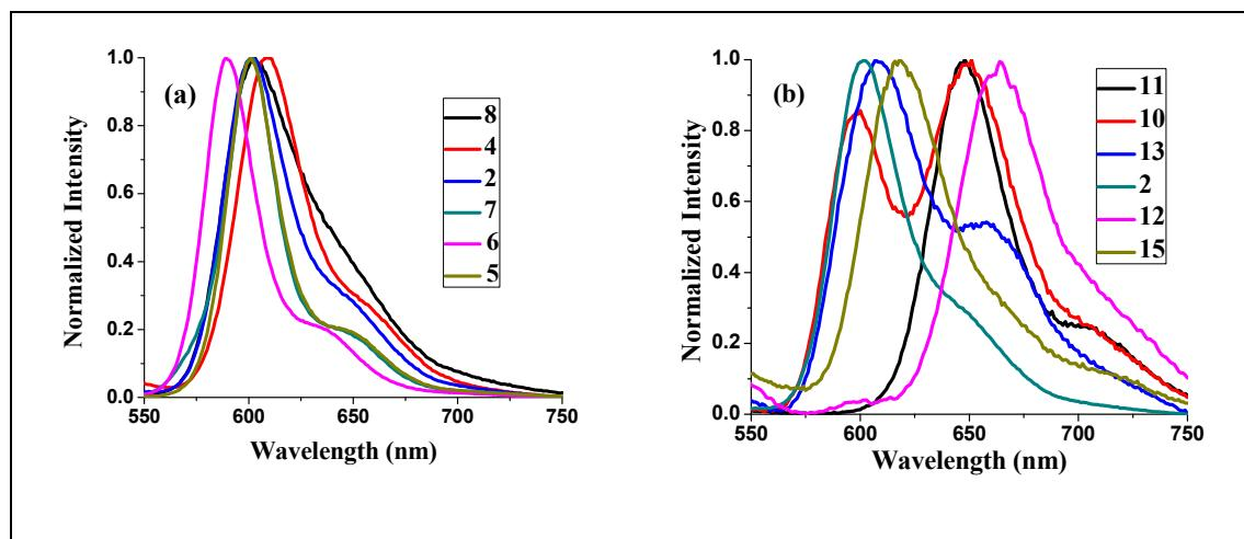
**Figure 66:** Comparison of normalized emission spectra of (a) functionalized 3-pyrrolyl BODIPYs and (b) aryl substituted 3-pyrrolyl BODIPYs recorded in  $\text{CHCl}_3$  using  $\lambda_{\text{exc}} = 488 \text{ nm}$ .
