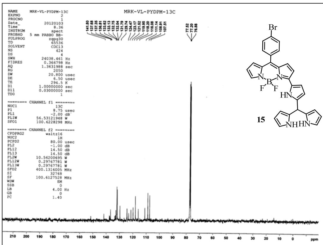
Figure 58 :  $^{13}\text{C}$  NMR spectrum of compound **15** recorded in  $\text{CDCl}_3$
