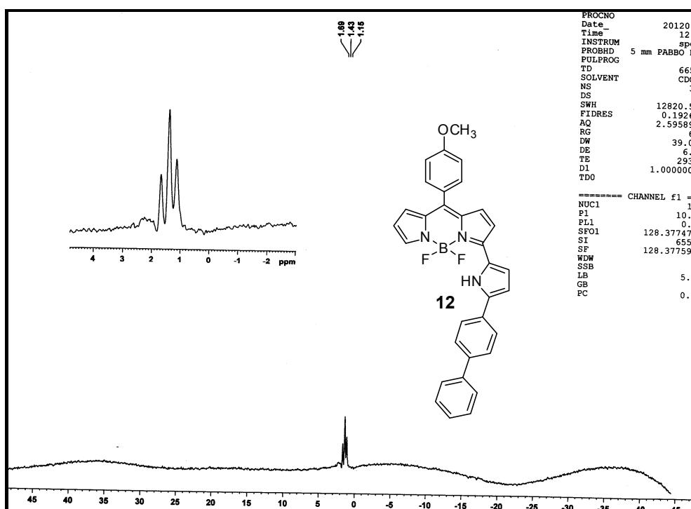
**Figure 46:**  $^{11}\text{B}$  NMR spectrum of compound **12** recorded in  $\text{CDCl}_3$
