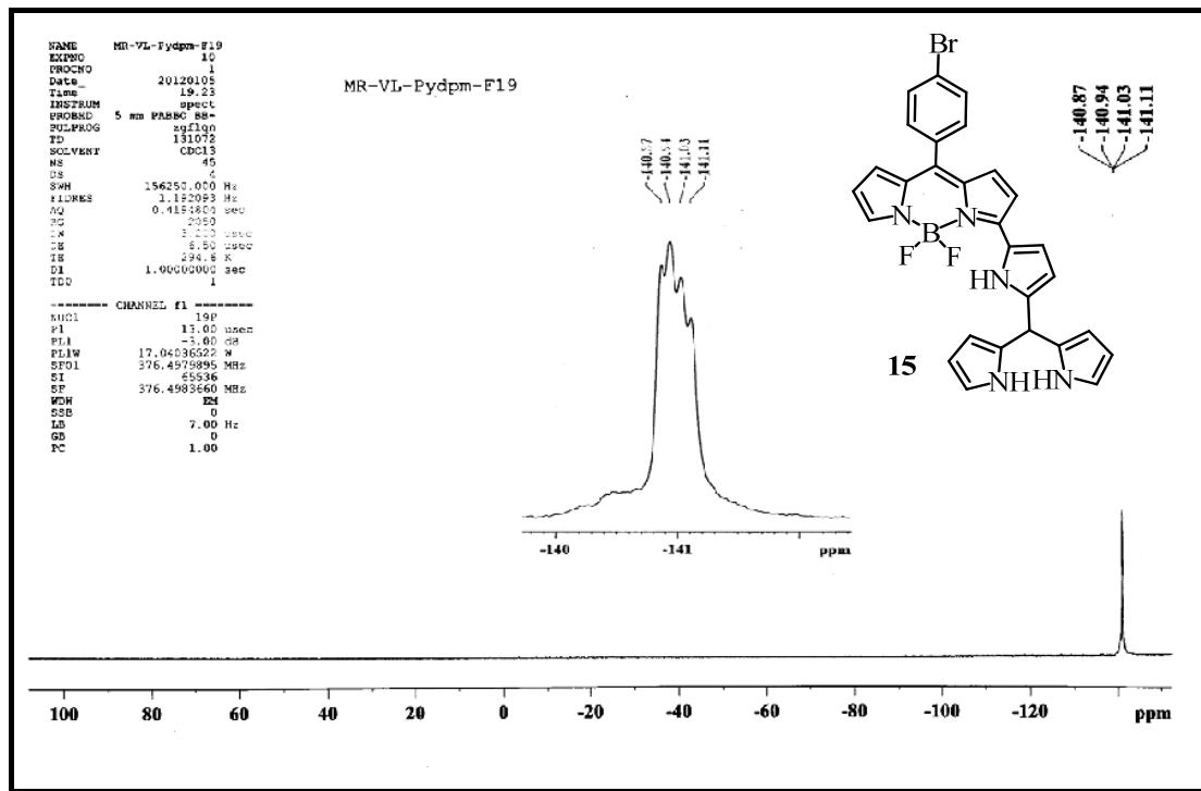
Figure 56 :  $^{19}\text{F}$  NMR spectrum of compound 15 recorded in  $\text{CDCl}_3$
