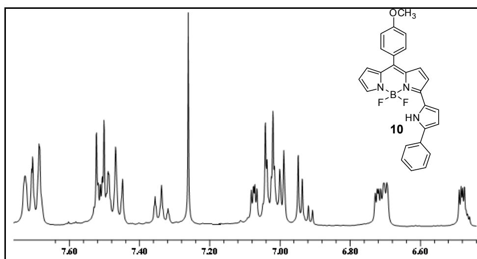
**Figure 31:** <sup>1</sup>H NMR spectrum of compound **10** in the selected region recorded in  $\text{CDCl}_3$
