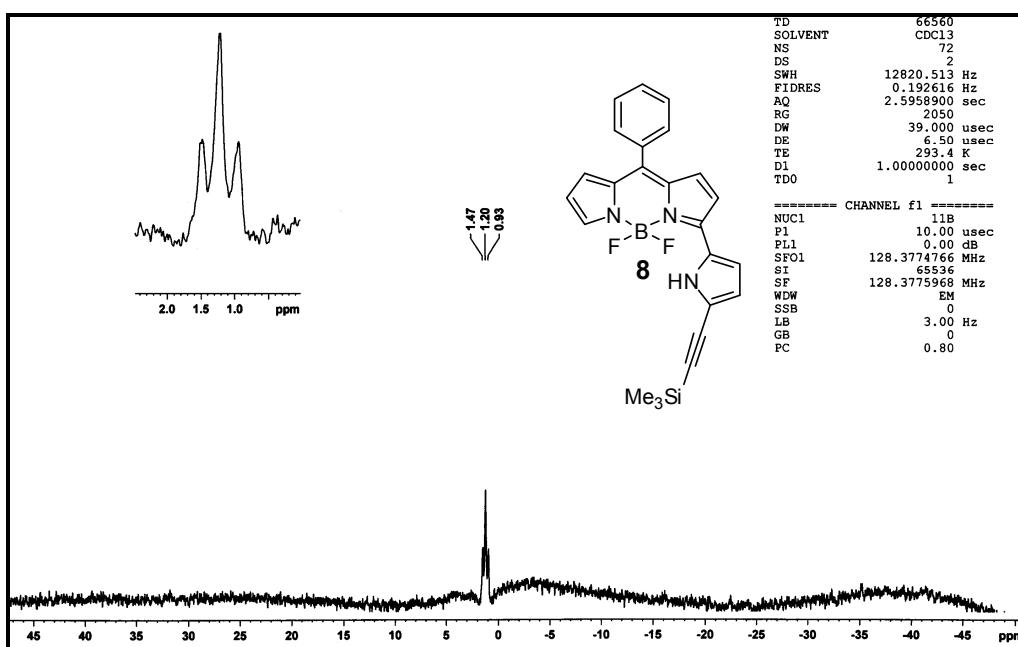
Figure 28:  $^{11}\text{B}$  NMR spectrum of compound 8 recorded in  $\text{CDCl}_3$
