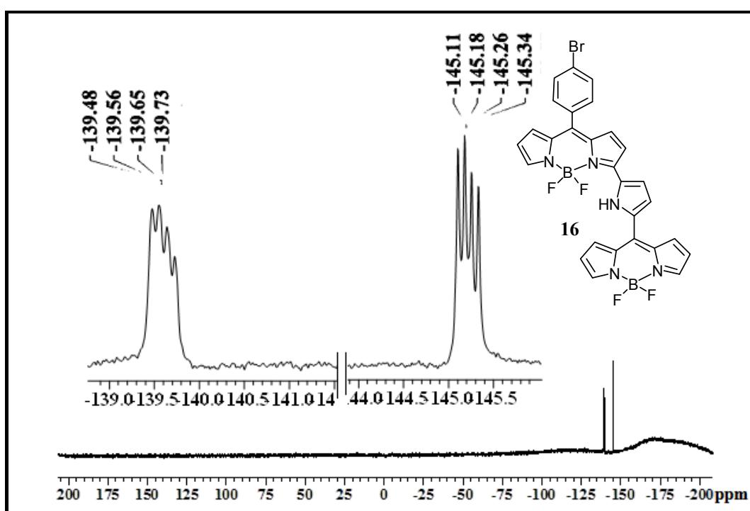
**Figure 62:** <sup>19</sup>F NMR spectrum of compound **16** recorded in CDCl<sub>3</sub>.
