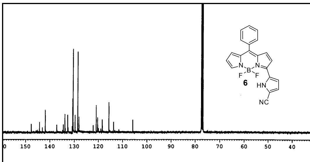
Figure 17: <sup>13</sup>C NMR spectrum of compound 6 recorded in CDCl<sub>3</sub>
