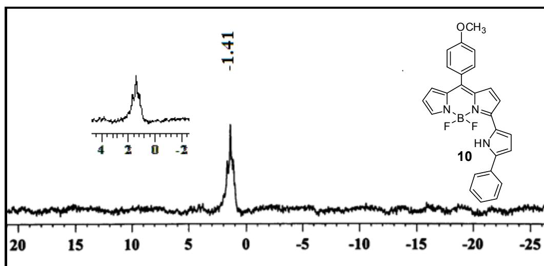
Figure 34:  $^{11}\text{B}$  NMR spectrum of compound **10** recorded in  $\text{CDCl}_3$  ( $\delta$  in ppm)
