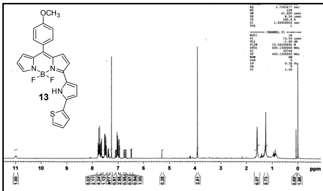
**Figure 50:** <sup>1</sup>H NMR spectrum of compound 13 recorded in CDCl<sub>3</sub>
