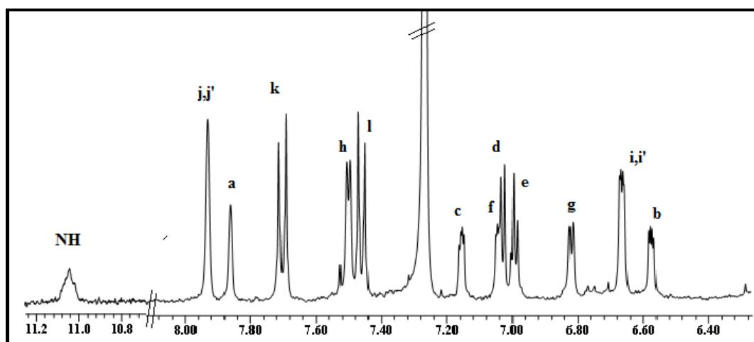
**Figure 61 :** <sup>1</sup>H NMR spectrum of compound 16 in selected region recorded in CDCl<sub>3</sub> ( $\delta$  in ppm).
