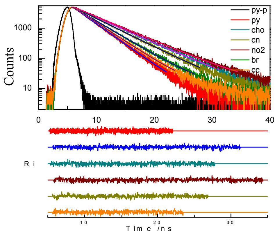
**Figure 68:** Fluorescence decay profile and weighted, residual, distribution fit of compounds **2** along with **4-8** in chloroform. The excitation wavelength used was 560 nm collected at corresponding wavelengths.
