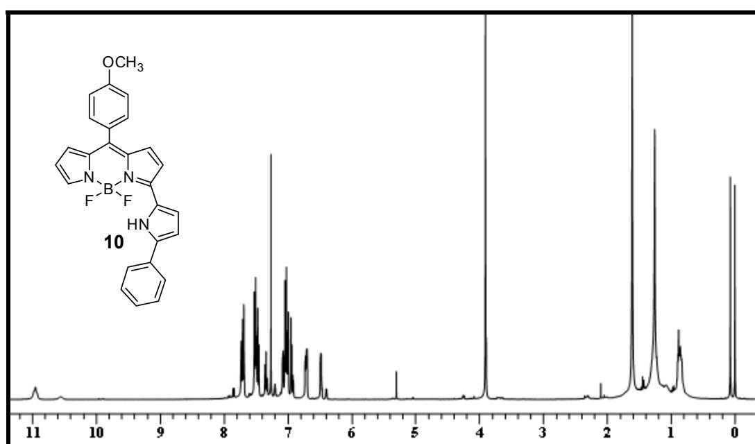
**Figure 32:** <sup>1</sup>H NMR spectrum of compound **10** recorded in  $\text{CDCl}_3$
