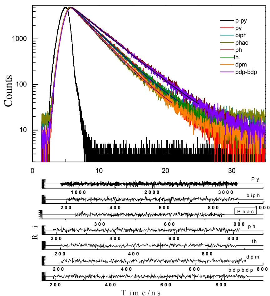
**Figure 69:** Fluorescence decay profile and weighted, residual, distribution fit of compounds **2** along with **10-16** in chloroform. The excitation wavelength used was 560 nm collected at corresponding wavelengths.
