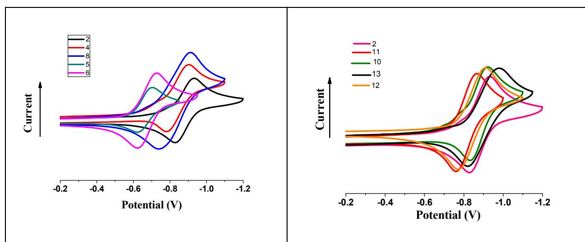
**Figure 67:** Comparison of the first reduction waves of cyclic voltammograms of compounds **2-13** at  $50 \text{ mV s}^{-1}$  scan rate recorded in  $\text{CH}_2\text{Cl}_2$  containing  $0.1 \text{ M}$  Tetrabutylammonium perchlorate as supporting electrolyte.
