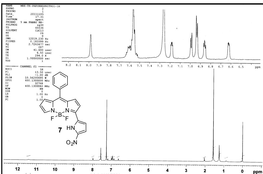
**Figure 19:** <sup>1</sup>H NMR spectrum of compound 7 recorded in CDCl<sub>3</sub>. The inset shows <sup>1</sup>H NMR spectrum in selected region.
