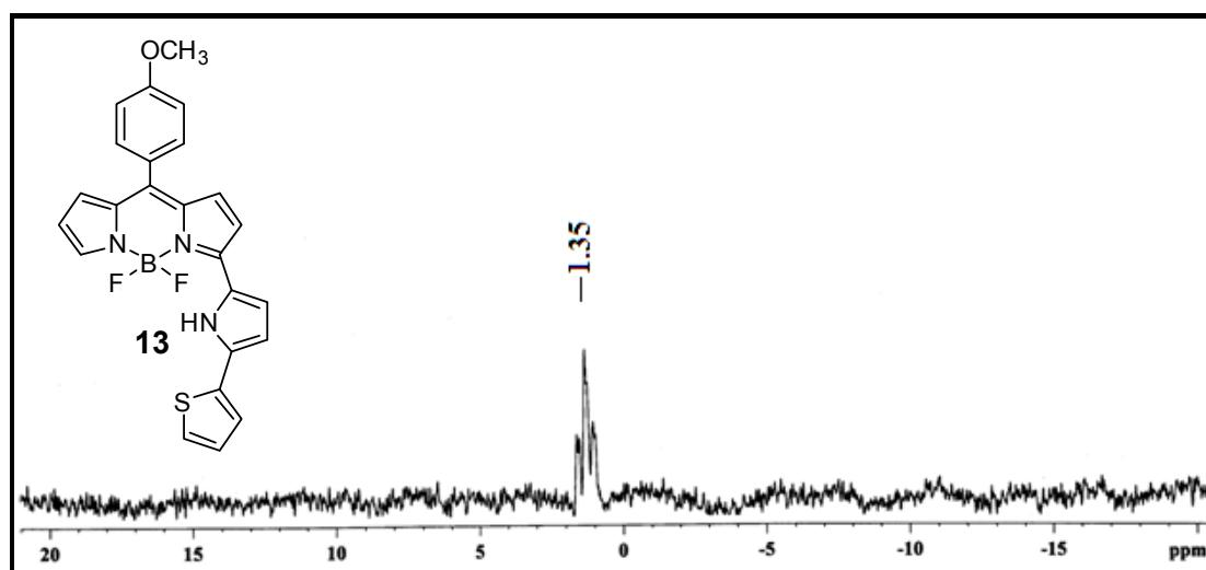
Figure 52:  $^{11}\text{B}$  NMR spectrum of compound 13 recorded in  $\text{CDCl}_3$
