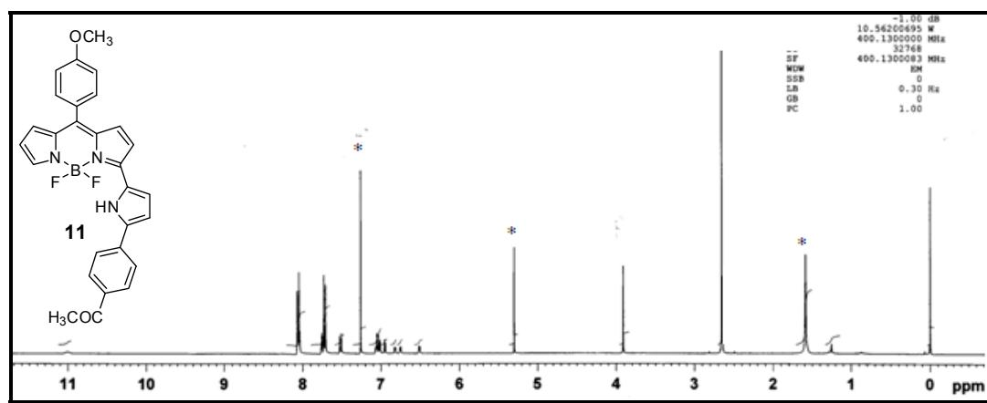
**Figure 38:** <sup>1</sup>H NMR spectrum of compound 11 recorded in  $\text{CDCl}_3$
