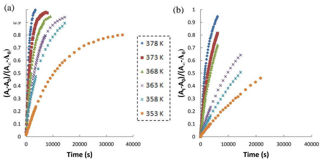
**Figure 4.** Plots of the normalised absorbance at 351 nm against time for the AB-modified ODN's **18a** (a) and **18b** (b)
