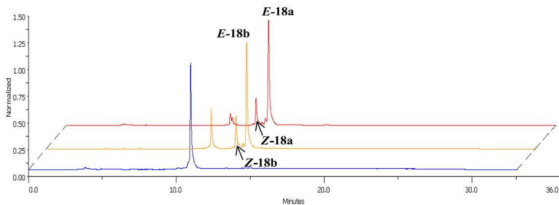
**Figure 3.** HPLC traces of crude ODN reaction products bearing an AB photoswitch at an internal position; starting material reference HO-5'-d(Tp)<sub>4</sub>Xpd(Tp)<sub>3</sub>dT-3'OH (obtained from **16**, blue), *meta*-disubstituted cycloadduct **18b** (orange), and *para*-disubstituted cycloadduct **18a** (red)
