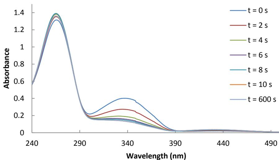
**Figure 7.** Overlaid UV/Vis spectra of **18a** upon irradiation at 366 nm for 0, 2, 4, 6, 8, 10 and 600 s
