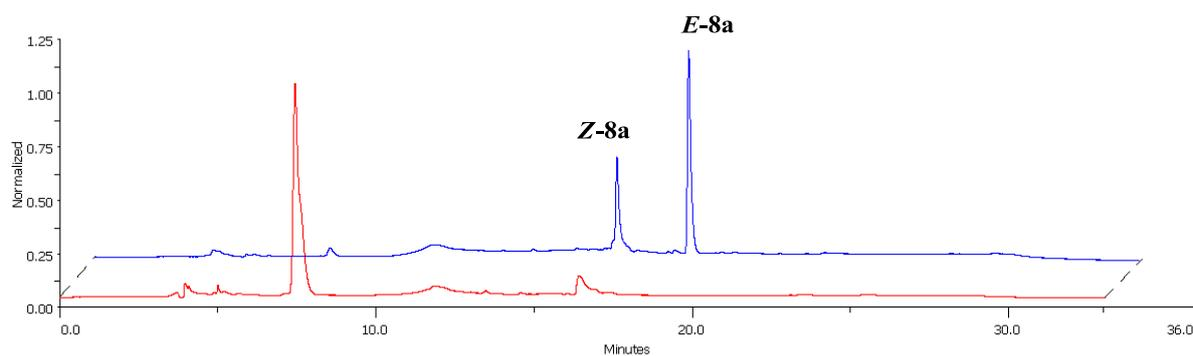
**Figure 1.** HPLC traces of the crude AB-labelled nucleoside **8a** (blue) and the starting material reference, 2'-O-propargyl uridine (red)
