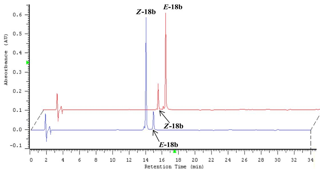
**Figure 10.** Overlaid HPLC traces of **18b** in the *Irr* (blue) and *DA* (red) photostationary states
