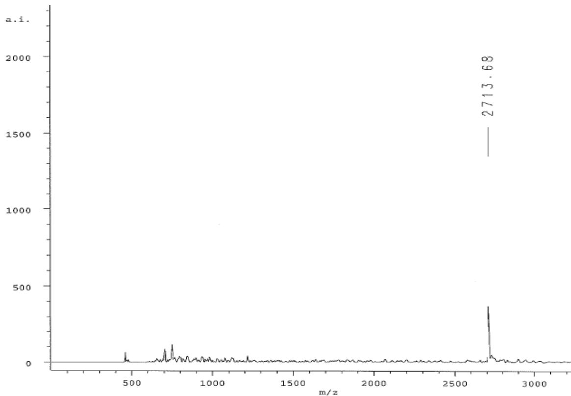
**Figure 28.** MALDI-TOF MS spectrum of HO-5'-d(Tp)<sub>4</sub>Xpd(Tp)<sub>3</sub>dT-OH obtained from **16** following deprotection and cleavage from the resin
