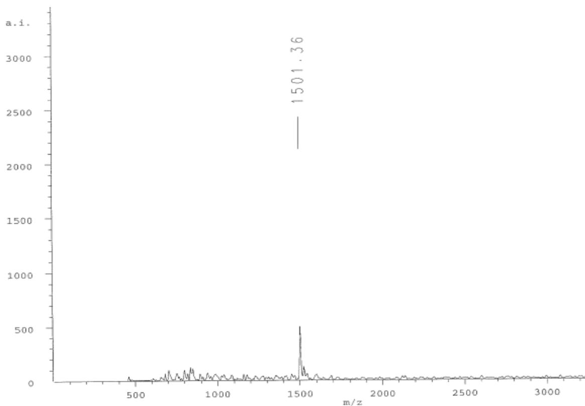
**Figure 26.** MALDI-TOF MS spectrum of HO-5'-Xpd(Tp)<sub>3</sub>dT-OH obtained from **13** following deprotection and cleavage from the resin
