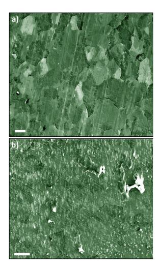
Figure S3: a) SEM image of pristine graphene grown on Ni foils showing that the graphene grain structure is similar to the underlying Ni crystal domains (scale bar:  $10~\mu m$ ). b) SEM image of albumin/fibrinogen -coated graphene showing complete coverage of protein on the substrate (scale bar:  $10~\mu m$ ).
