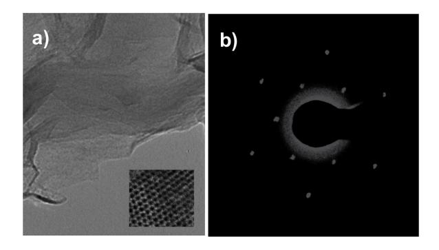
Figure S2: a) Transmission electron micrograph for single-layer graphene grown on Cu substrates. The inset shows high-resolution image with the honey comb lattice of graphene. b) Electron-diffraction pattern conforms that the 1 sccm samples grown on Cu substrates are indeed single-layers.
