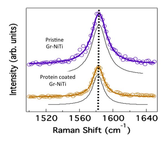
Figure S1: The micro-Raman spectra of bare and fibrinogen-coated graphene. The solid traces represent the results of Lorentzian lineshape data analysis (open circles) which suggests no evidence of a shift in the *G*-band frequency, and hence no charge transfer from the fibrinogen to Gr-NiTi.
