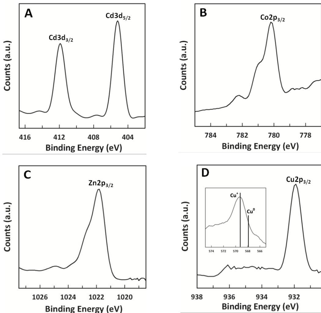
**Fig. S2** X-ray photoelectron spectroscopy (XPS) spectra obtained from (A) Fe/CdS, (B) Fe/CoS, (C) Fe/ZnS, and (D) Fe/Cu<sub>2</sub>S NPs (inset : Auger Cu LMM spectrum).
