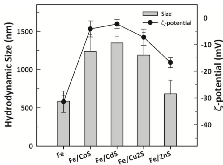
**Fig. S4** Hydrodynamic sizes and  $\zeta$ -potentials of the diluted suspension of Fe and Fe/MeS NPs (20 mg/L) at pH  $7.0 \pm 0.2$  in the absence of background electrolyte.
