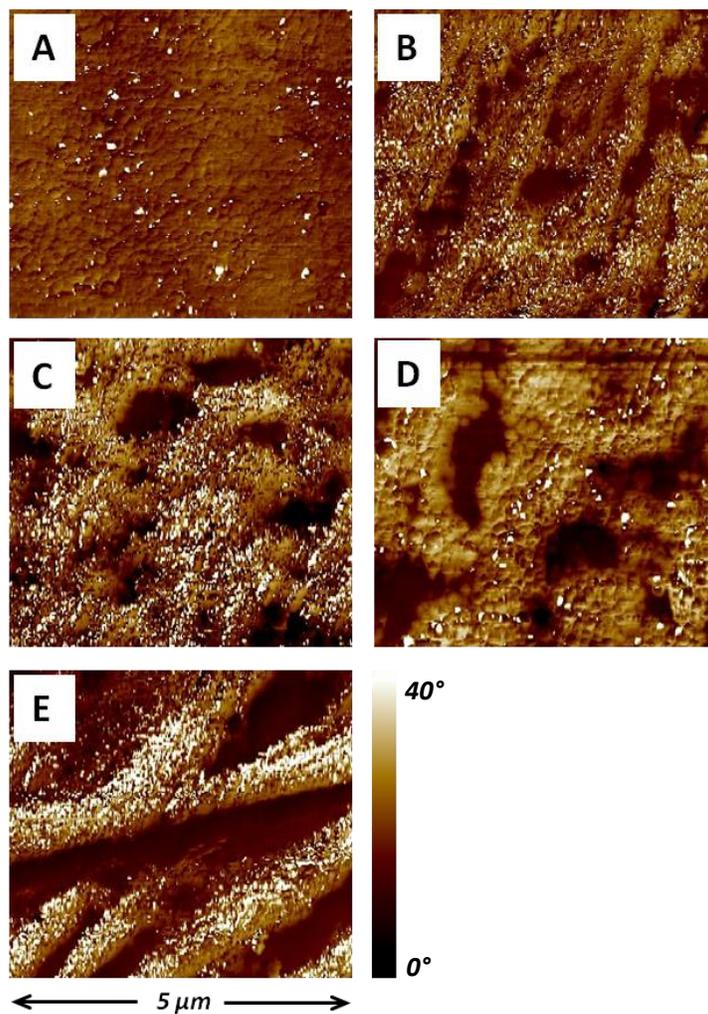
**Fig. S3** Electrostatic force microscopy (EFM) images of (A) Fe, (B) Fe/CdS, (C) Fe/CoS, (D) Fe/ZnS, and (E) Fe/Cu<sub>2</sub>S NPs.
