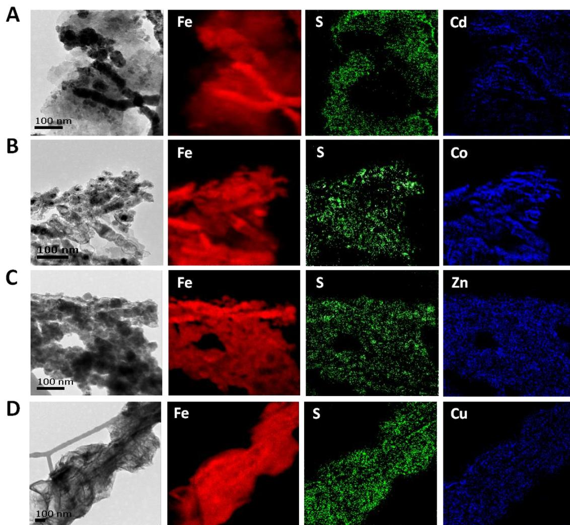
**Fig. S1** Energy filtered transmission electron microscopy (EFTEM) images of (A) Fe/CdS, (B) Fe/CoS, (C) Fe/ZnS, and (D) Fe/Cu<sub>2</sub>S NPs.
