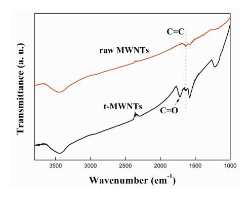
**Figure S2.** The FTIR spectra of the raw MWNTs and t-MWNTs, respectively. Curve of the t-MWNTs has peaks located at 1720 and 1250 cm<sup>-1</sup>, corresponding to C=O and C-O stretching, respectively, indicating that a large amount of oxygen-containing groups has been introduced to the surface of MWNTs during acid treatment.
