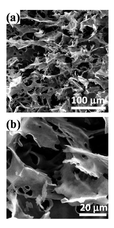
**Figure S3.** SEM images of the fracture surface of the thermally treated MWNT-carbon hybrid aerogel at low and high magnifications, exhibit a 3D network with pore sizes of tens of micrometers, indicating that the thermal treatments did not change the essential morphology of hybrid aerogels.
