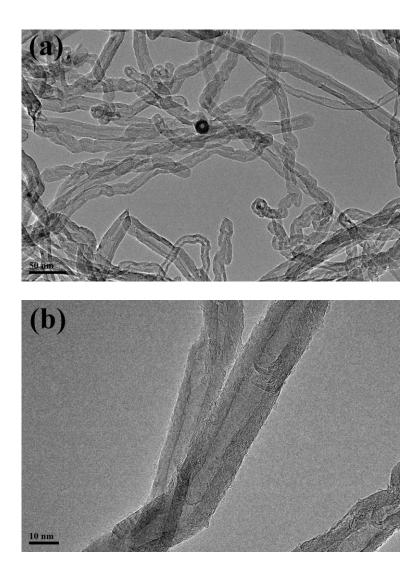
Figure S1. TEM images of the raw MWNTs at low and high magnifications.
