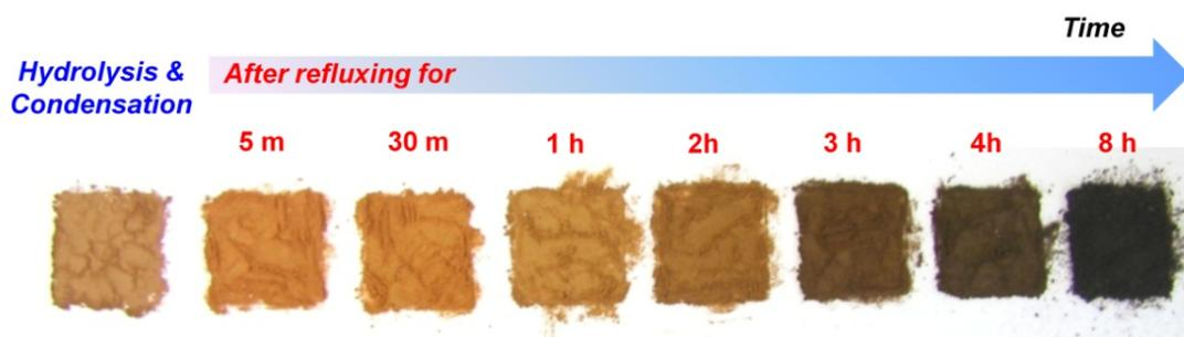
**Fig. S2** Photograph of isolated powders of iron oxides at different reaction times.
