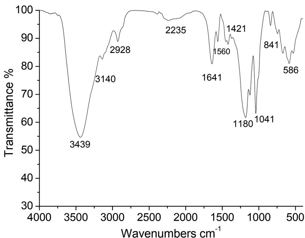
**Figure S7-3.** IR of poly[(3-(1-vinylimidazoliumyl)propanesulfonate)-*co*-(sodium 4-styrene sulfonate)] **A** on KBr Pellets. IR (KBr,  $\text{cm}^{-1}$ ):  $\nu = 3439$  (O–H,  $\text{H}_2\text{O}$ , vs); 3140 (C–H, m); 2928 (C–H, w); 1641 (m), 1560 (w), 1421 (w), (C=N and C=C); 1180 ( $\text{SO}_3^-$ , s); 1042 ( $\text{SO}_3^-$ , s); 586 (C–H, m).
