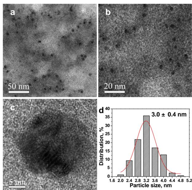
**Figure S3-2.** TEM micrographs (a-c) and size distributions (d) of recovered Pd after three times recycling.
