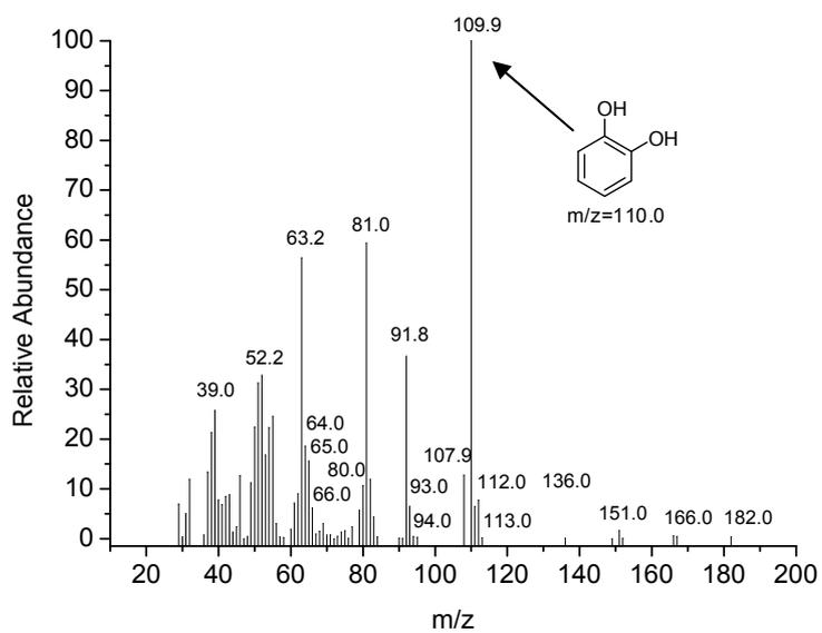
Figure S6-5. GC-MS of pyrocatechol (Table 2, run 7)
