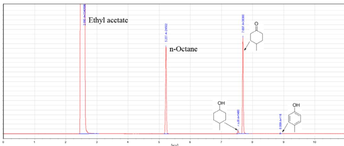
Figure S5-3. GC of 4-methylphenol hydrogenation (Table 2, run 3)
