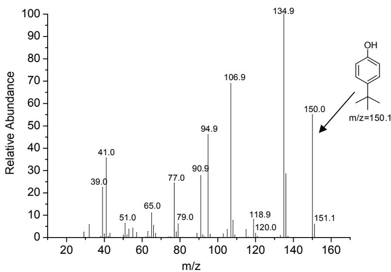
Figure S6-2. GC-MS of 4-tert-butylphenol (Table 2, run 4)
