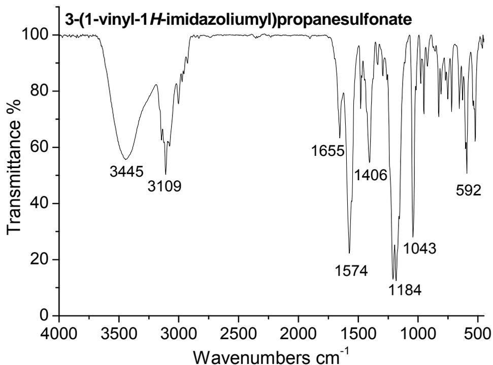
**Figure S7-2.** IR of 3-(1-vinyl-1*H*-imidazoliumyl)propanesulfonate **3** on KBr Pellet. IR (KBr,  $\text{cm}^{-1}$ ):  $\nu = 3445$  (O–H, vs); 3109 (C–H, w); 1655 (w), 1574 (vs), 1406 (m), (C=N and C=C); 1184 ( $\text{SO}_3^-$ , vs); 1043 ( $\text{SO}_3^-$ , vs); 592 (C–H, w).
