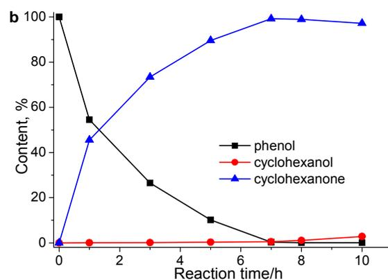
**Figure S2-2** time-conversion profile. Reactions conditions: phenol (33 mg, 0.35 mmol),  $K_2PdCl_4$  (5 mol% relative to phenol), **A** (20 mol% relative to phenol), HPA (10 mol% relative to phenol),  $H_2$  (0.1 MPa), water (3 mL), reaction temperature, (80°C).
