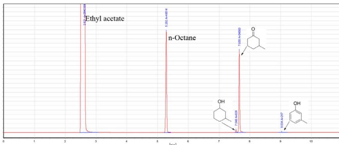
Figure S5-2. GC of 3-methylphenol hydrogenation (Table 2, run 2)
