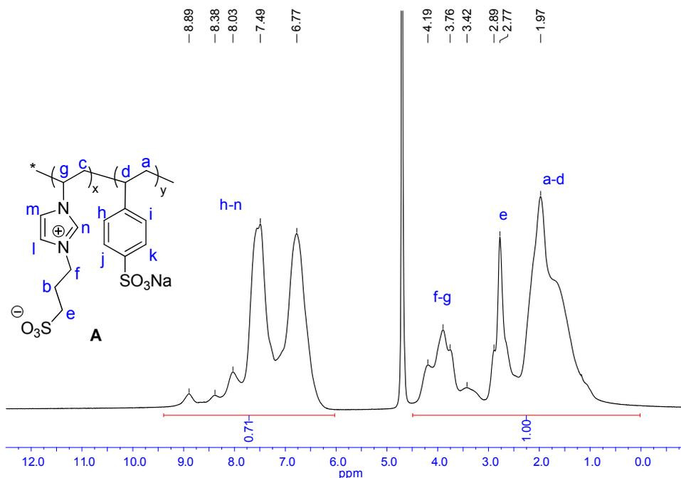
**Figure S7-4.**  $^1\text{H}$  NMR (400 MHz,  $\text{D}_2\text{O}$ ) of poly[(3-(1-vinylimidazoliumyl)propanesulfonate)-*co*-(sodium 4-styrene sulfonate)] **A**,
