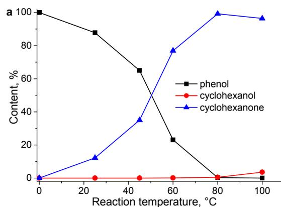
**Figure S2-1** temperature-conversion profile. Reactions conditions: phenol (33 mg, 0.35 mmol),  $K_2PdCl_4$  (5 mol% relative to phenol), **A** (20 mol% relative to phenol), HPA (10 mol% relative to phenol),  $H_2$  (0.1 MPa), water (3 mL), reaction time, (7 h).
