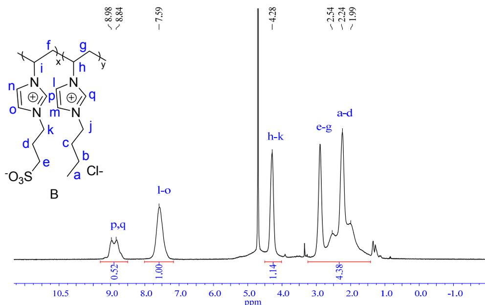
**Figure S7-5.**  $^1\text{H}$  NMR of **B** in  $\text{D}_2\text{O}$ . Based on the integration in  $^1\text{H}$  NMR of copolymer **B**, the molar ratio of “x : y” is “1 : 1.7”.
