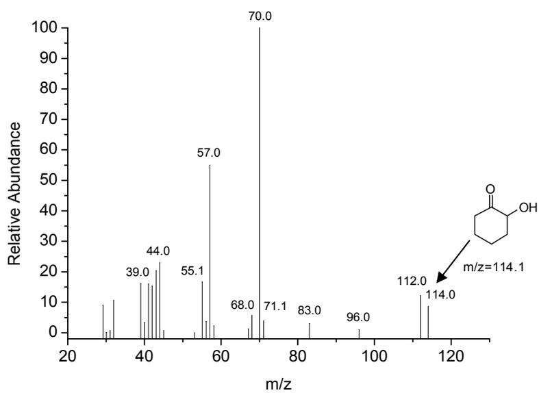
Figure S6-6. GC-MS of 2-hydroxycyclohexanone (Table 2, run 7)
