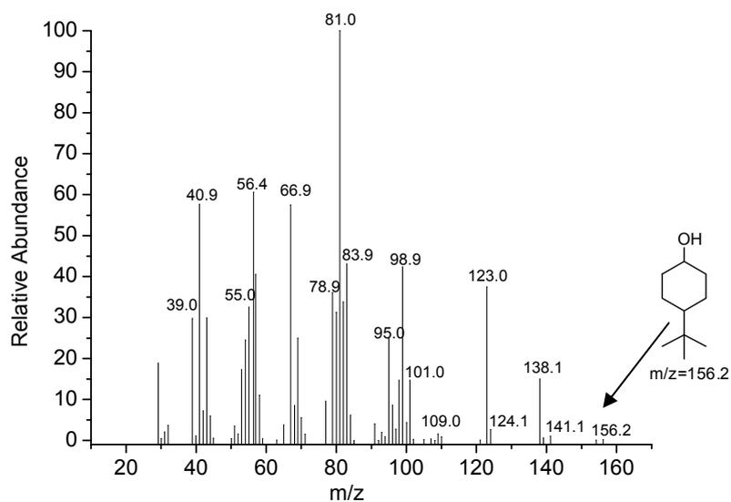
Figure S6-4. GC-MS of 4-tert-butylcyclohexanol (Table 2, run 4)
