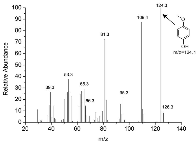
Figure S6-7. GC-MS of 4-methoxyphenol (Table 2, run 8)
