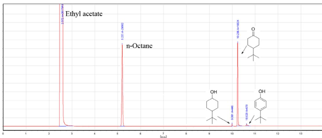
Figure S5-4. GC of 4-tert-butylphenol hydrogenation (Table 2, run 4)
