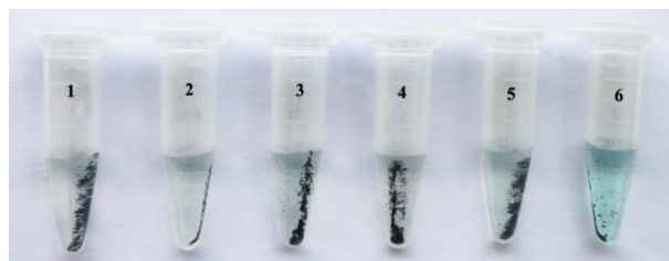
Figure S5 Photographs of TMB–nanohybrid–GOx in the presence of different sugars: (1) blank, (2) 10 mM lactose, (3) 10 mM maltose, (4) 10 mM fructose, (5) 10 mM sucrose, (6) 50 \mu\text{M} glucose. Experimental conditions: 100 \mu\text{L} of 5 mM TMB, 20 \mu\text{L} of 5 \text{mg mL}^{-1} GOx, 50 \mu\text{L} of SWCNT–hemin nanohybrid, 200 \mu\text{L} of 50 mM NaAc–HAc (pH 4.3).
