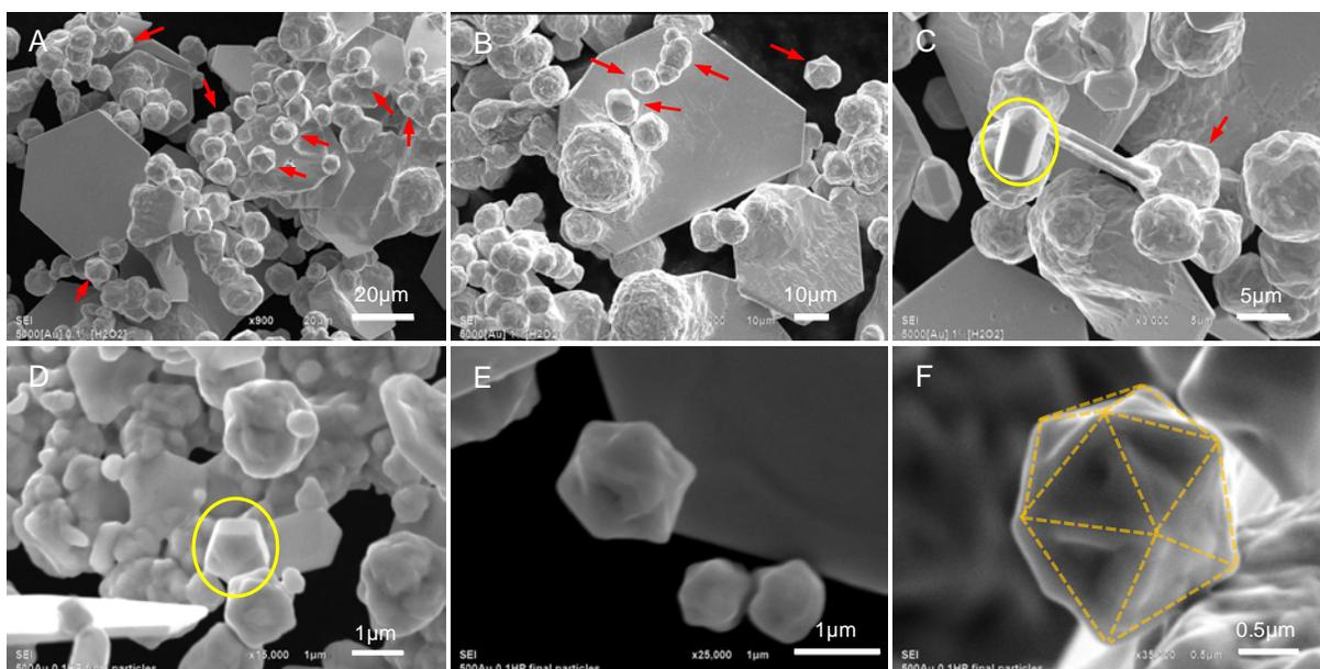
**Figure S2.** SEM micrograph of gold microparticles obtained from the reaction of H<sub>AuCl</sub><sub>4</sub> (25.4 mM) and H<sub>2</sub>O<sub>2</sub> concentration at 32 mM (A, D-F) and 320 mM (B and C) without starch stabilizer. The red arrows in (A), (B) and (C) indicate icosahedron gold quasi-microspheres. The yellow circles in (C) and (D) indicate pentagonal rods. (E and F) icosahedron quasi-microspheres generated during the growth process.
