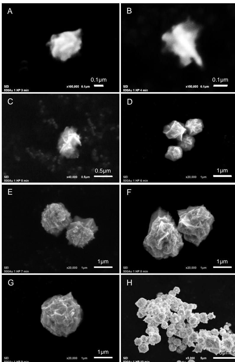
**Figure S6.** Time-dependent SEM micrographs show the development of quasi-spherical gold microparticles. The quasi-spherical gold microparticles were obtained from the reaction of  $\text{HAuCl}_4$  (2.54 mM) and  $\text{H}_2\text{O}_2$  (320 mM) without the starch stabilizer. The SEM micrographs were recorded at (A) 3, (B) 4, (C) 5, (D) 6, (E) 7, (F) 8, (G) 9 and (H) 10 min reaction time.
