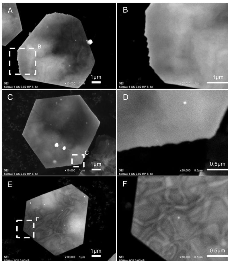
**Figure S4.** SEM micrographs show rough edges of growing gold nanosheets. During the growth process (6 h reaction time, A -D), the edges of the gold nanosheets can be etched by  $O_2/Cl^-$ .<sup>1</sup> The recrystallization process smooth the rough edges after a prolong reaction time of 10 h (E, F). Gold nanosheets were obtained from the reaction of 2.54 mM  $HAuCl_4$ , 6.4 mM  $H_2O_2$  and 1% w/v starch.
