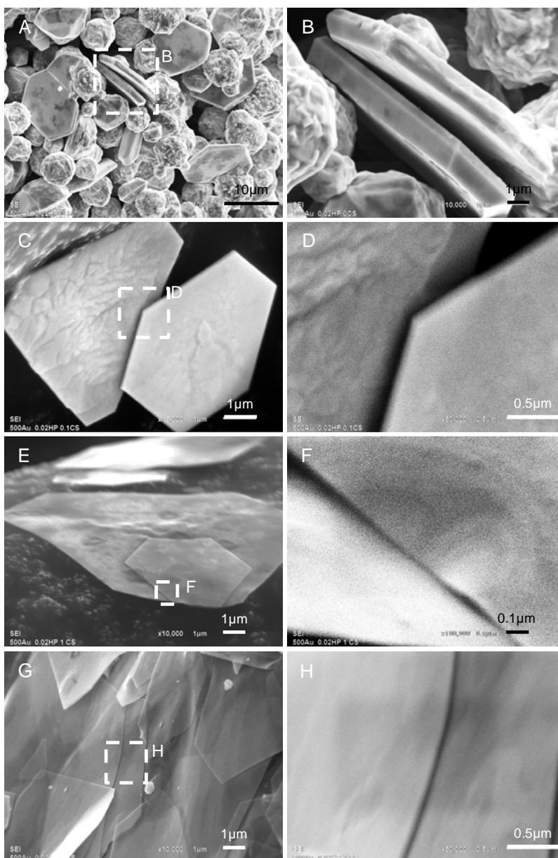
**Figure S3.** SEM micrographs of gold quasi-microspheres, microplates and nanosheets. The thickness of the nanosheets decreases as the concentrations of starch stabilizer was increased. Gold nanosheets were obtained from the reaction of 2.54 mM  $\text{HAuCl}_4$ , 6.4 mM  $\text{H}_2\text{O}_2$  and starch: (A, B) 0%, (C, D) 0.1%, (E, F) 1% and (G, H) 2% w/v.
