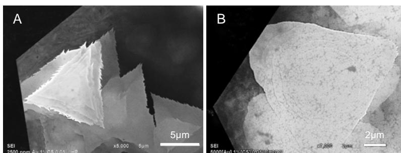
**Figure S5.** SEM micrographs show layer-by-layer epitaxial growth of gold film on the basal planes of gold nanosheets. The growth always ceases at the edge of the basal planes. Gold nanosheets were obtained from the reaction of (A) 12.7 mM and (B) 25.4 mM  $\text{HAuCl}_4$ , 3.2 mM  $\text{H}_2\text{O}_2$  and 1% w/v starch.
