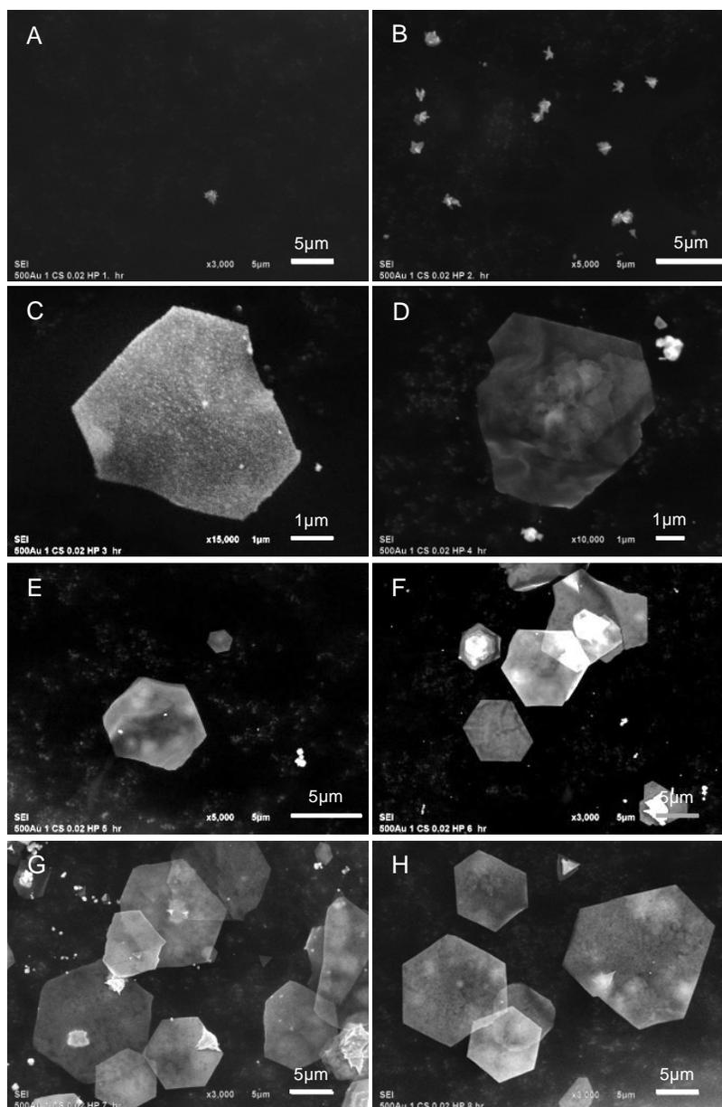
**Figure S7.** Time-dependent SEM micrographs show the development of gold nanosheets. The nanosheets were obtained from the reaction of  $\text{HAuCl}_4$  (2.54 mM),  $\text{H}_2\text{O}_2$  (6.4 mM), and starch (1% w/V). The SEM micrographs were recorded at (A) 1, (B) 2, (C) 3, (D) 4, (E) 5, (F) 6, (G) 7 and (H) 8 h reaction time.
