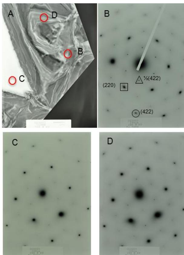
**Figure S8.** (A) TEM image of a nanosheet. The big nanosheets fill up the TEM frame even at a low resolution. (B-D) The corresponding selected area electron diffraction (SAED) pattern of a nanosheets. The positions for the SAED measurements are indicated in the TEM image. The same SAED patterns with hexagonal diffraction spots confirm that the nanosheet is a single crystal bound by {111} facets.
