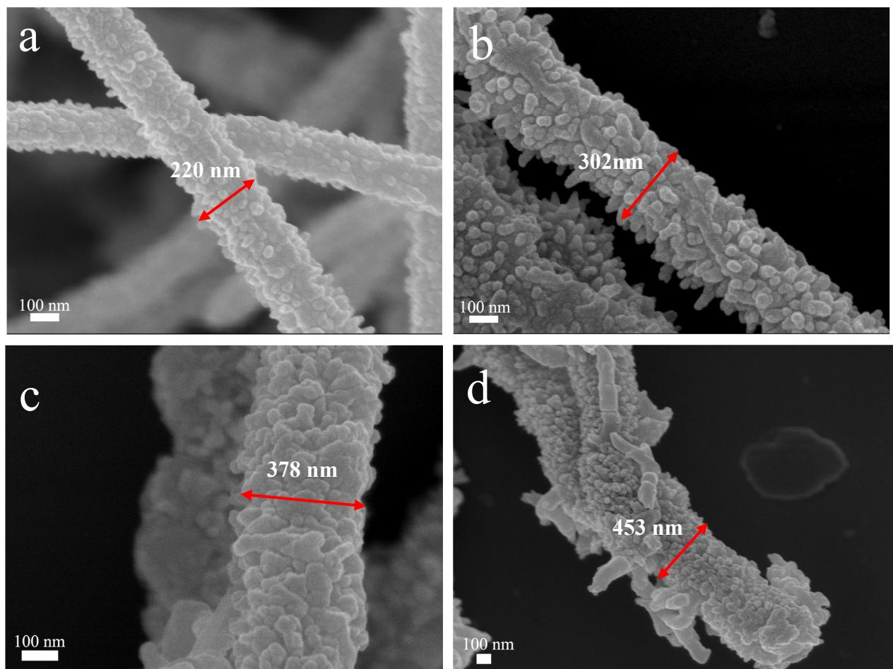
**Figure S2.** SEM images of the PANI/CFs nanocomposites with different concentration of aniline: (a) 5 mM; (b) 10 mM; (c) 25 mM; and (d) 50 mM. Other conditions: aniline/APS=1/1 (molar ratio), CF = $0.3\text{ mg ml}^{-1}$ , and the reaction was carried out 0 °C for 7 h.
