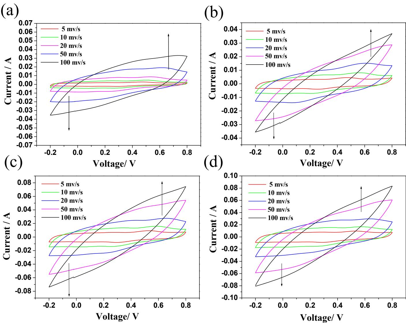
**Figure S3.** The Cyclic voltammetry curves of PANI/CFs with different aniline concentration at different scan rate: 5, 10, 20, 50, and 100 mV/s: (a) 5 mM; (b) 10 mM; (c) 25 mM; and (d) 50 mM.
