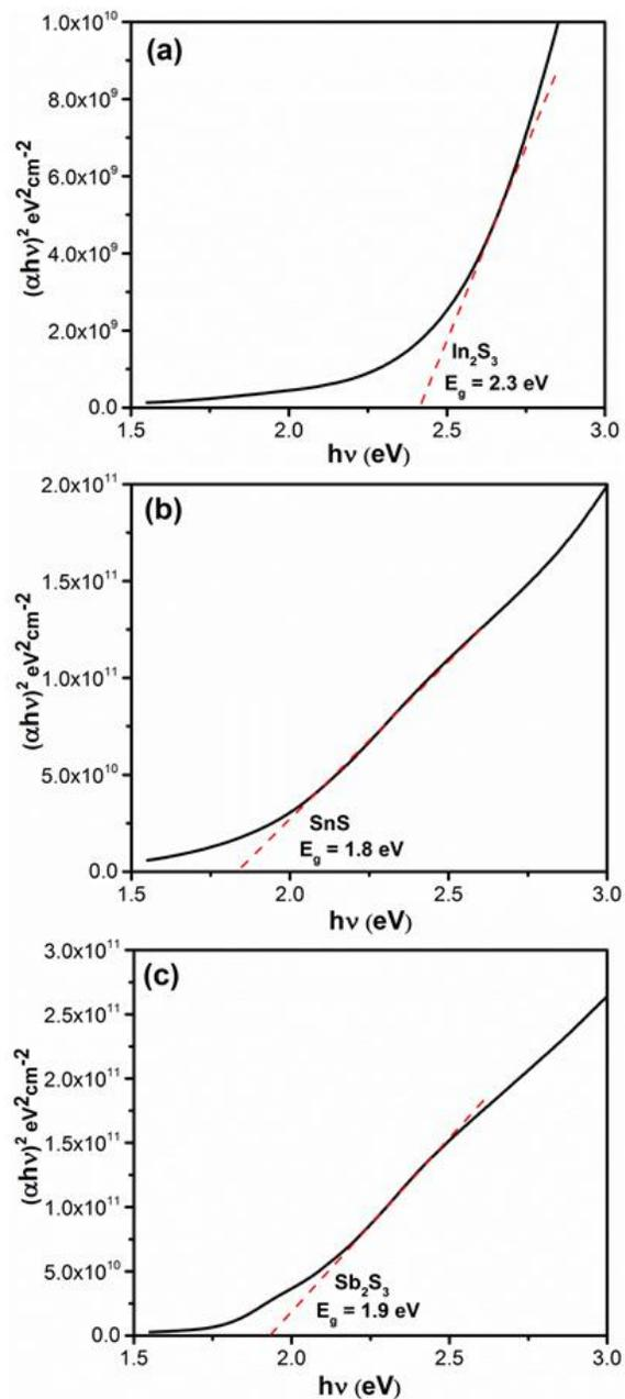
Fig. S4: Band gap calculation for (a)  $\text{In}_2\text{S}_3$ , (b)  $\text{SnS}$ , and (c)  $\text{Sb}_2\text{S}_3$  metal films.  $\text{TiO}_2$ -coated ITO glass substrates were used as background reference, and their spectra were subtracted.
