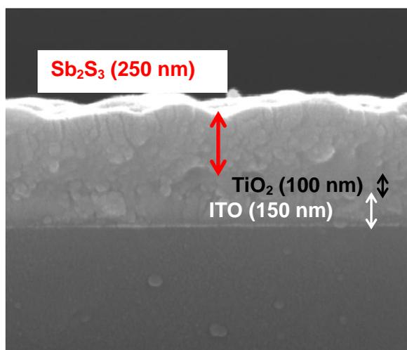
Fig. S3: Cross-sectional SEM image of Sb<sub>2</sub>S<sub>3</sub> films (16 h) on TiO<sub>2</sub>-coated ITO-glass substrates.
