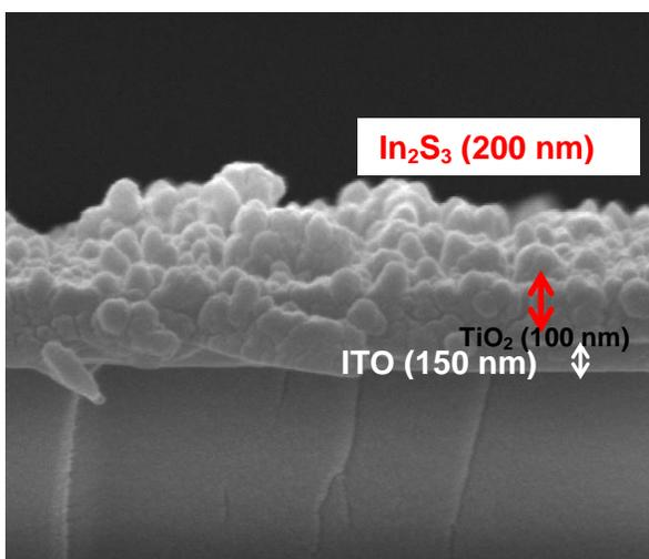
Fig. S1. Cross-sectional SEM image of  $\text{In}_2\text{S}_3$  films (90 min) on  $\text{TiO}_2$ -coated ITO-glass substrates.
