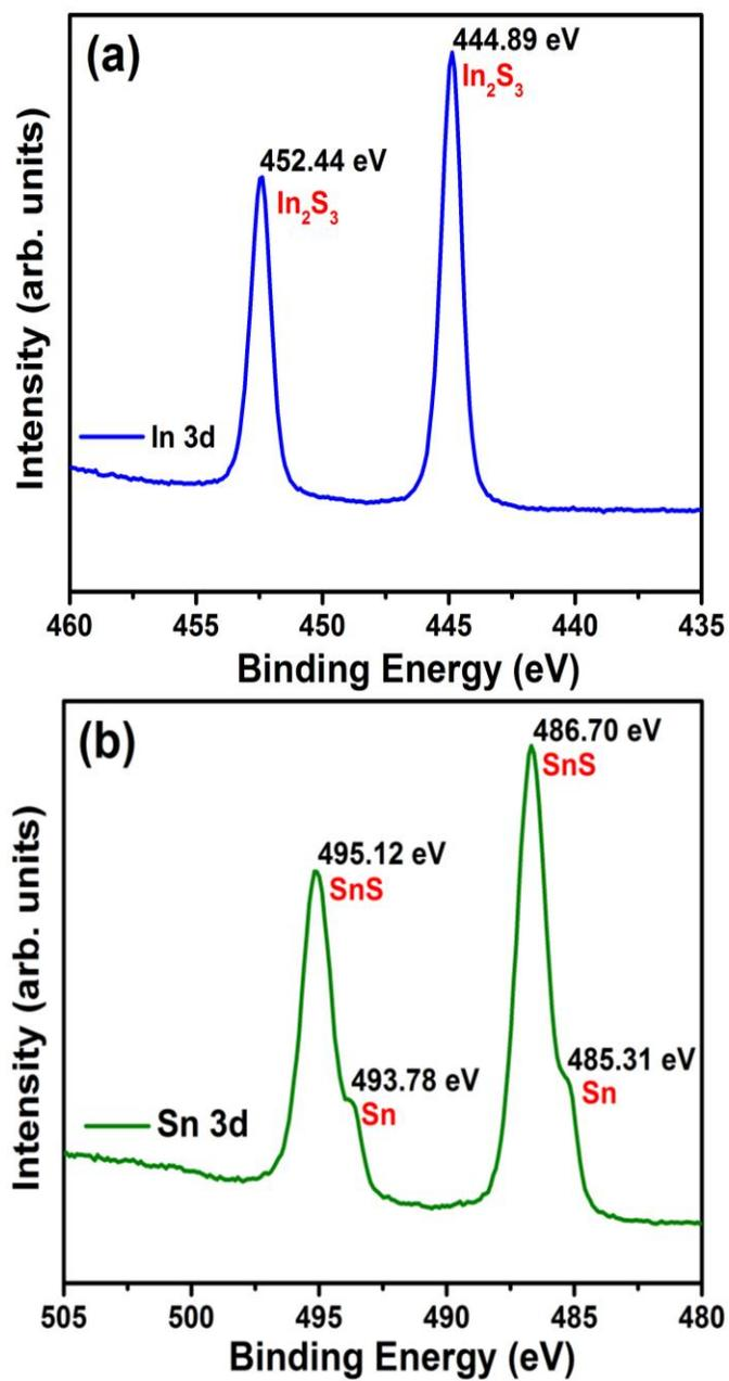
Fig. S5: XPS metal 3d spectra of (a) In and (b) Sn on surface of metal sulfides.
