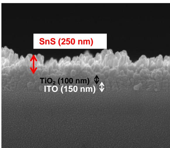
Fig. S2: Cross-sectional SEM image of  $\text{SnS}$  films (80 min) on  $\text{TiO}_2$ -coated ITO-glass substrates.
