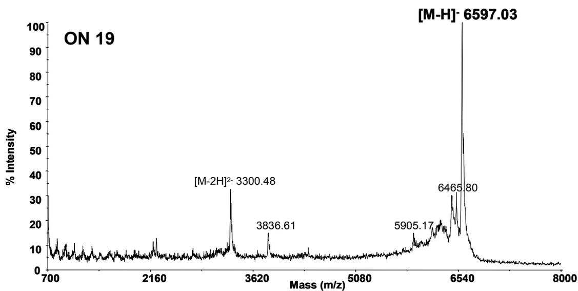
**Figure S51:** MALDI-TOF MS analysis of **pure ON 19:** GpppA<sub>OMe</sub>GU UGU UAG UCU UAC GUG A
