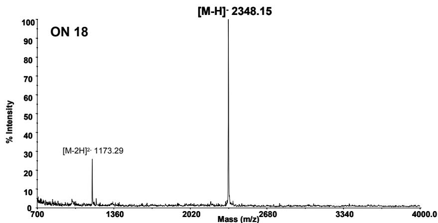
Figure S46: MALDI-TOF MS analysis of pure ON 18: GpppAUA UUA
