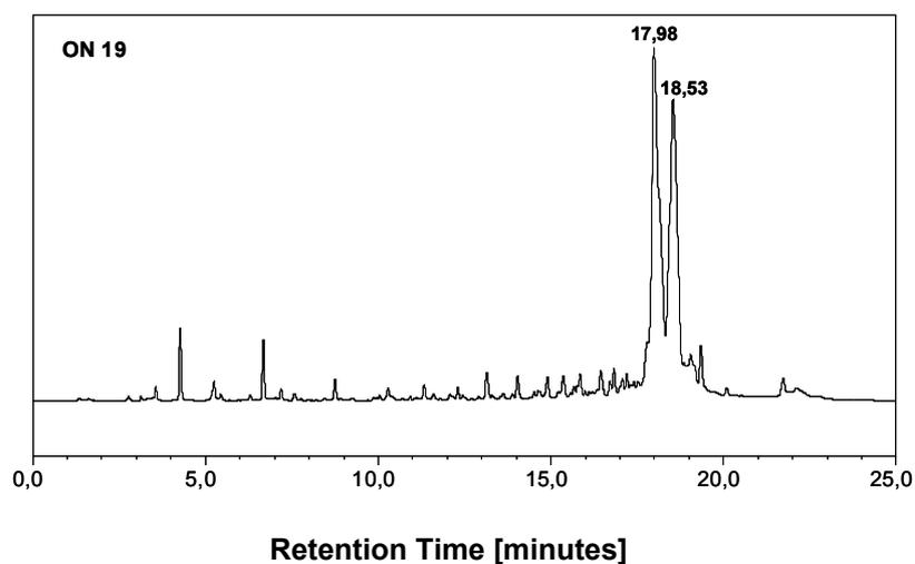
**Figure S49:** IEX-HPLC analysis of crude ON 19 (after NAP-10 G-25 Sephadex) :
