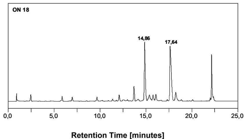
Figure S44: IEX-HPLC analysis of crude ON 18: GpppAUA UUA
