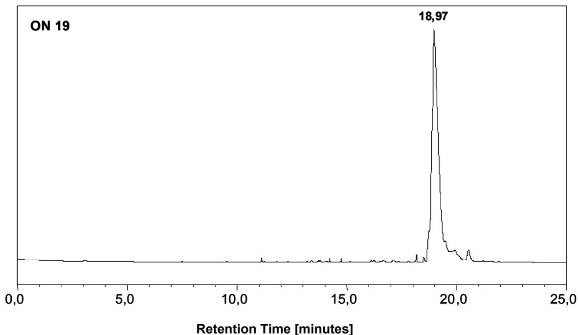
**Figure S50:** IEX-HPLC analysis of **pure ON 19:** GpppA<sub>OMe</sub>GU UGU UAG UCU UAC GUG A
