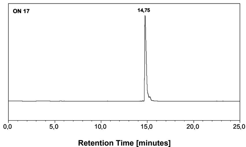
**Figure S41:** IEX-HPLC analysis of pure ON 17: <sup>7m</sup>GpppAUA UUA at  $\lambda$  260 nm
