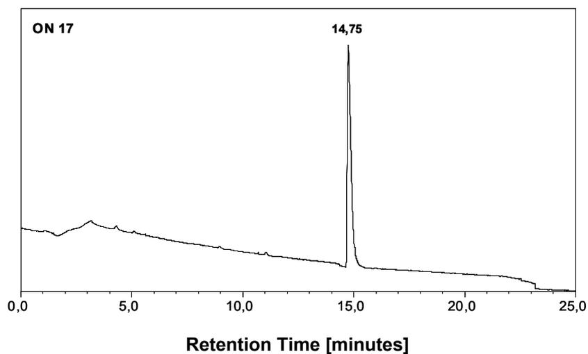
**Figure S42:** IEX-HPLC analysis of pure ON 17: <sup>7m</sup>GpppAUA UUA at  $\lambda$  300 nm.
