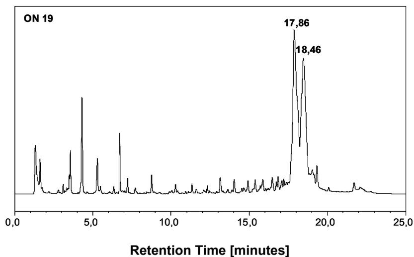
**Figure S48:** IEX-HPLC analysis of crude ON 19: GpppA<sub>OMe</sub>GU UGU UAG UCU UAC GUG A
