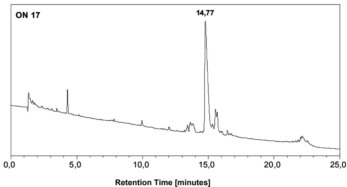
**Figure S40:** IEX-HPLC analysis of crude ON 17:  $^{7m}$ GpppAUA UUA at  $\lambda$  300 nm
