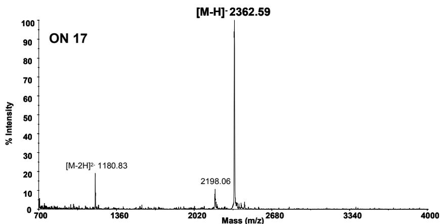
**Figure S43:** MALDI-TOF MS analysis of pure ON 17: <sup>7m</sup>GpppAUA UUA.
