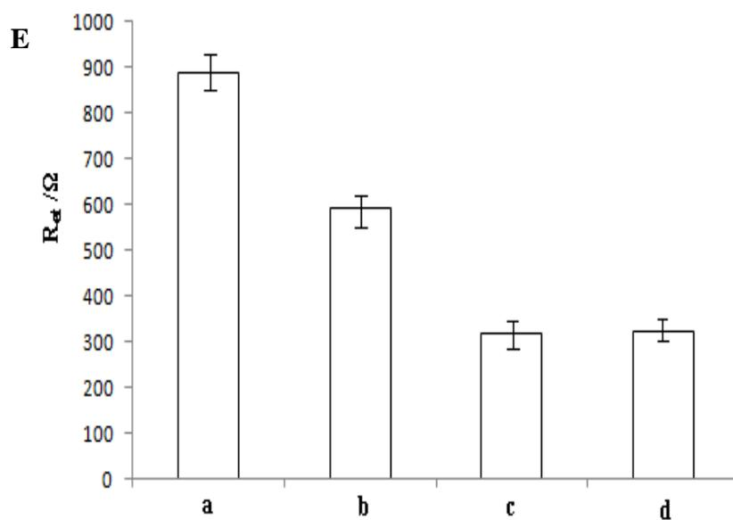
Figure S4. CVs (A) and Nyquist diagrams (B) of 1.0 mM  $[\text{Fe}(\text{CN})_6]^{3-/4-}$  recorded at (a) bare GCE, (b) FePt/GCE, (c) FePt/CNTs/GCE and (d) FePt/GO/GCE. The histograms of above CV (C, D) and EIS (E) results.
