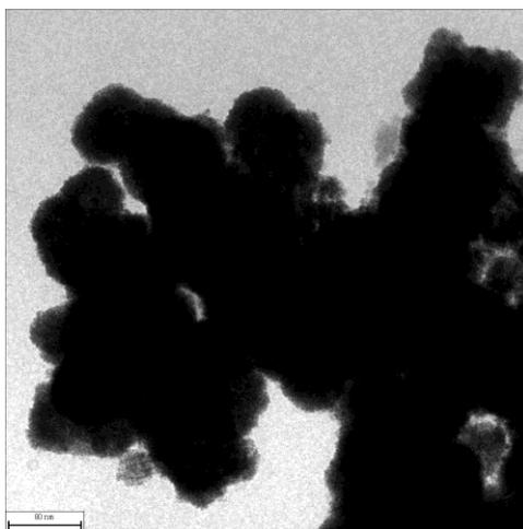
Figure S1. TEM image of aggregated FePt NPs, without the assistance of CNTs or GO
