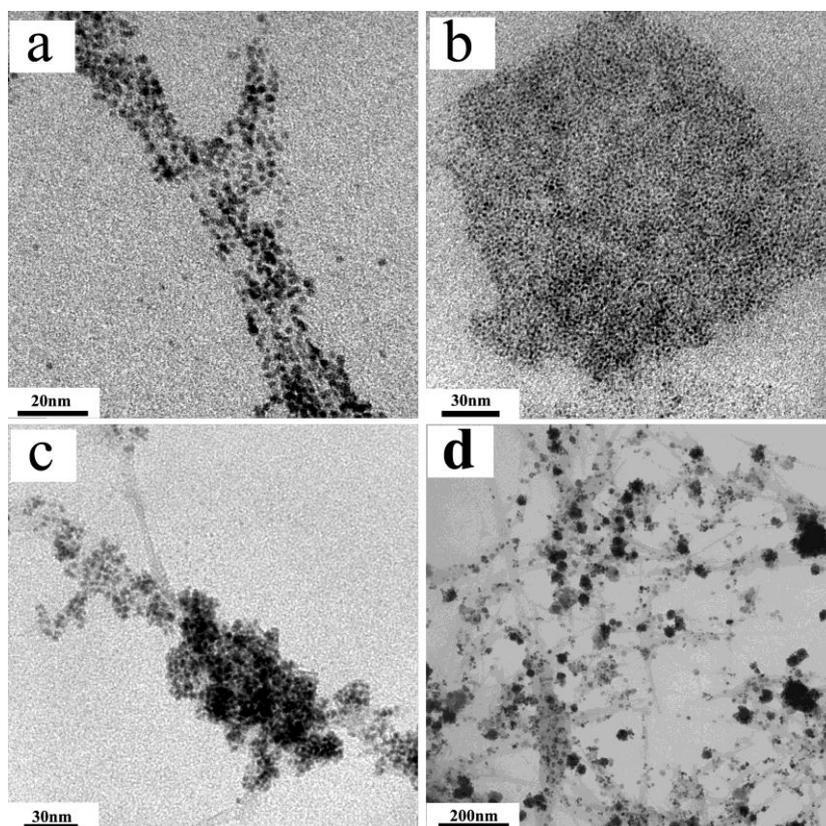
Figure S3. The influence of solvents on the morphology and density of as-prepared samples (a) FePt/CNTs and (b) FePt/GO using EG as solvent and reducing agent. (c) FePt/CNTs, using DMSO as solvents and EG as reducing agent. (d) FePt/CNTs, using OAm and OA as solvents and EG as reducing agent.
