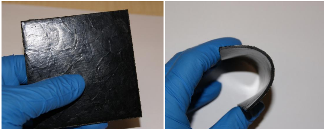
Figure S1. Digital photograph of a PU/D-Graphene nanocomposite film sample containing 0.94 vol.% D-Graphene sheets (100mm × 100mm × 2mm).
